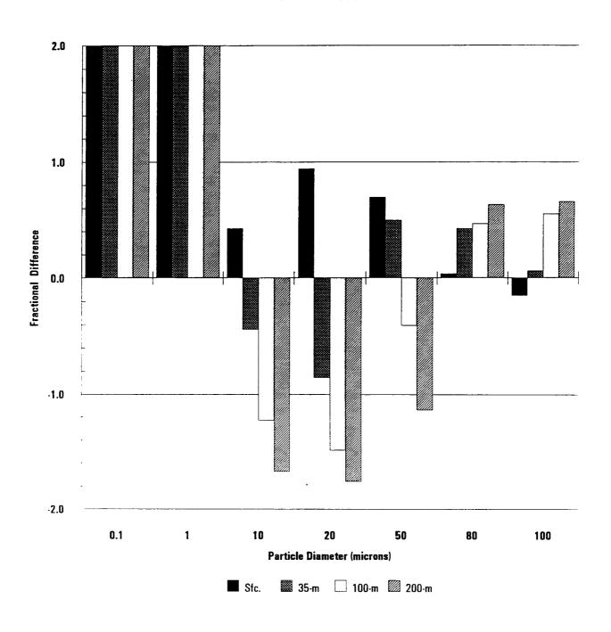
FIGURE 6 Fractional difference (FD) of highest 24-hour ISCST deposition estimates based on old and new algorithms for particle sizes and release heights as indicated  $FD = 2 \; (\text{NEW - OLD}) \; / \; (\text{NEW + OLD})$
