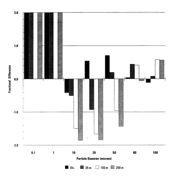
FIGURE 5 Fractional difference (FD) of highest 3-hour ISCST deposition estimates based on old and new algorithms for particle sizes and release heights as indicated  $FD = 2 \; (\text{NEW - OLD}) \, / \, (\text{NEW + OLD})$
