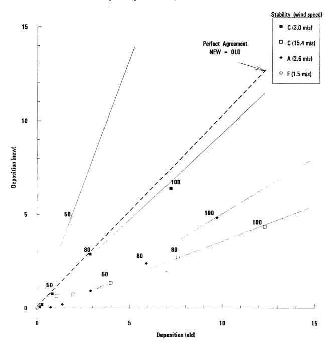
FIGURE 4 Fractional difference (FD) of highest 1-hour ISCST deposition estimates based on old and new algorithms for particle sizes and release heights as indicated  $FD = 2 \, (\text{NEW - OLD}) \, / \, (\text{NEW + OLD})$
