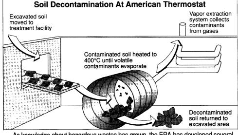
As knowledge about hazardous wastes has grown, the EPA has developed several methods for soil decontamination. Based on the type of contamination at the American Thermostat site, the soil was treated with a low-temperature heat to evaporate the volatile organic compounds.
