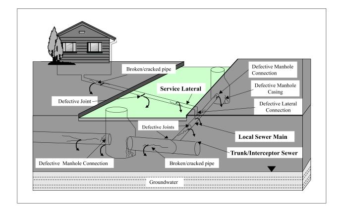
Figure 2-1. Sanitary sewer system components and exfiltration sources.
