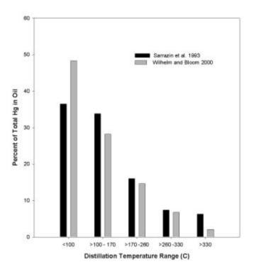
Figure 6-3 – Mercury (Total) in Distilled Products
