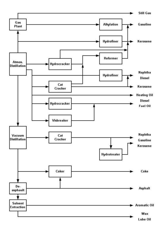
Figure 4-1 - Typical Refining Process
