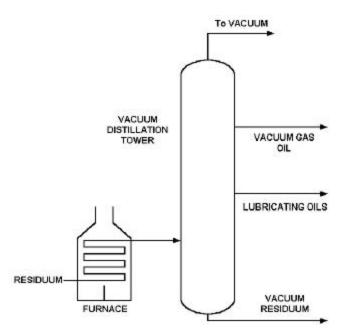
Figure 4-3 – Vacuum Distillation
