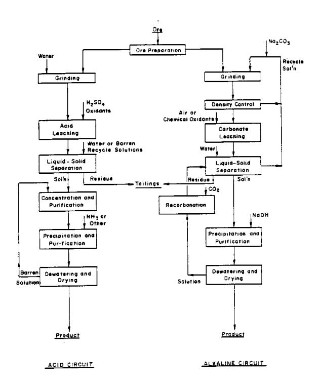
Figure 1-6. Comparison of Acid and Alkaline Leaching Circuits
