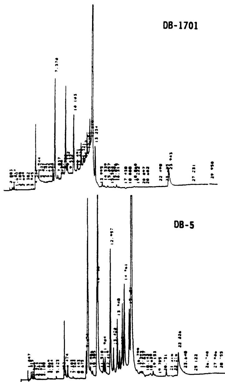
FIGURE 17. GC/ECD chromatogram of Halowax 1001 analyzed on a DB-5/DB-1701 fused-silica open-tubular column pair. The GC operating conditions were as follows: 30 m x 0.53 mm ID DB-5 (1.5- \mu m film thickness) and 30 m x 0.53 mm ID DB-1701 (1.0- \mu m film thickness) connected to a J&W Scientific press-fit Y-shaped inlet splitter. Temperature program: 150°C (0.5 min hold) to 190°C (2 min hold) at 12°C/min then to 275°C (10 min hold) at 4°C/min.
