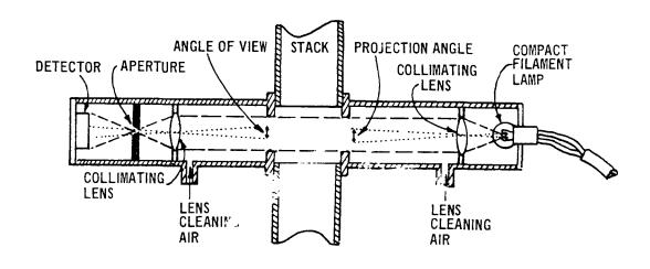
Figure 3-3. Transmissometer with Collimating Features.
