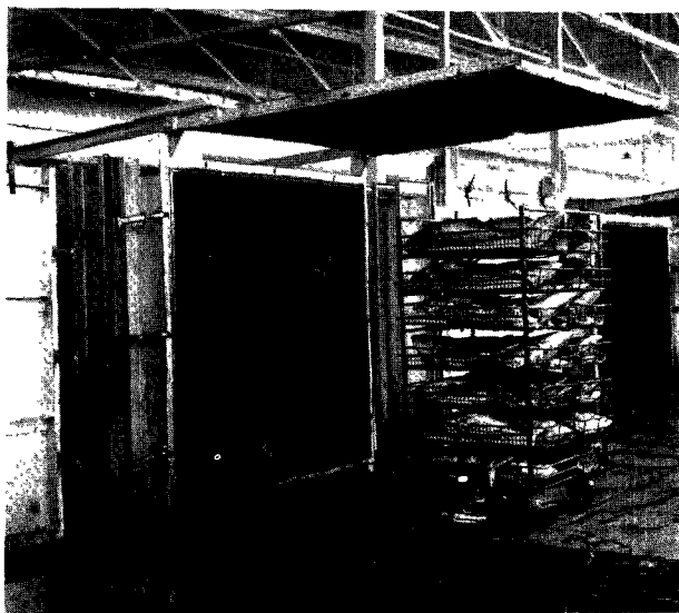
Figure 554. A bank of live-steam-heated cookers used to process raw, whole tuna (Star-Kist Foods Inc., Terminal Island, Calif.).
