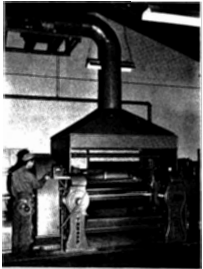
Figure 270. Rubber mill with exhaust hood (National Seal Division, Federal-Mogul-Bower Bearings, Inc., Downey, Calif.).
