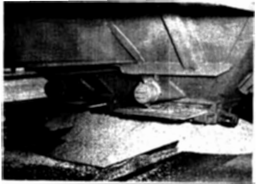
Figure 247. Hopper bottom railroad car unloading grain into a shallow hopper by the choked-feed method (Koppel Bulk Terminal, Long Beach, Calif.).
