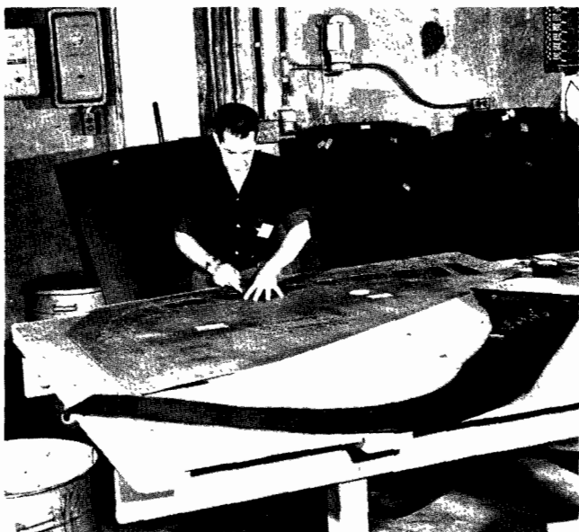
Figure 643. The masking on a titanium part is being scribed by use of a template. After scribing, the masking will be stripped from those areas shown by the holes in the templates. The stripped areas will then be milled. The black part in the foreground and those in the background have not yet been scribed (U.S. Chemical Milling Corporation, Manhattan Beach, Calif.).
