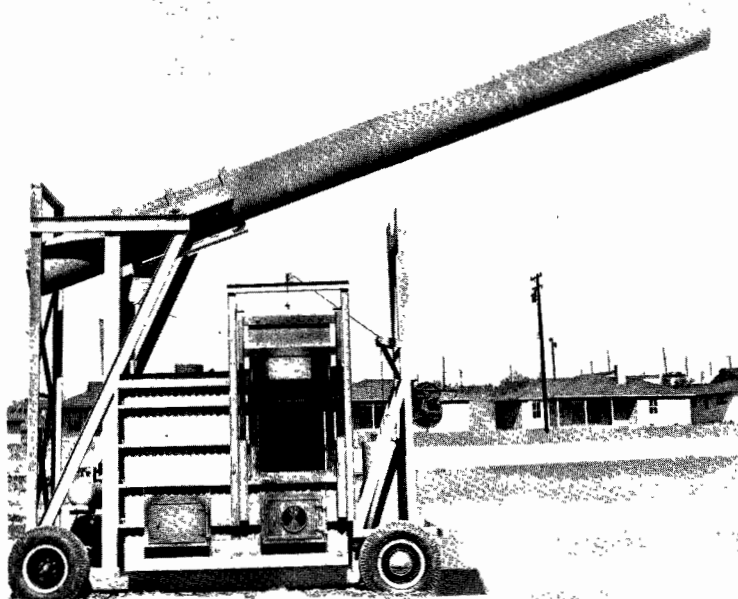
Figure 345. A 500-pound-per-hour mobile incinerator with retractable stack.
