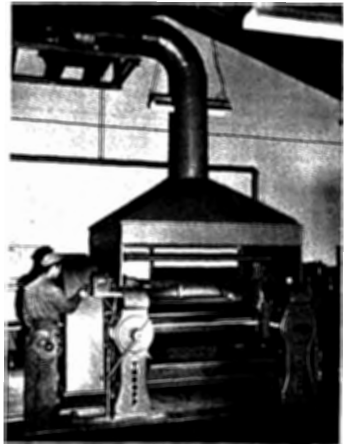
Figure 270. Rubber mill with exhaust hood (National Seal Division, Federal-Mogul-Bower Bearings, Inc., Downey, Calif.).
