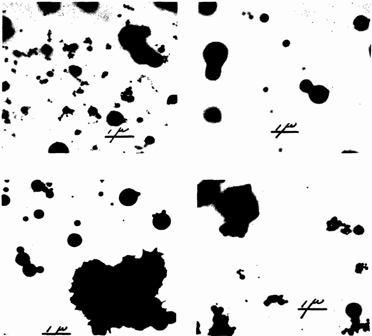
Figure 169. Electron photomicrographs of fumes from an electric furnace producing steel for castings (Allen et al., 1952).
