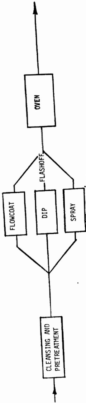
a) ConveyORIZED or batch single coat operation.
