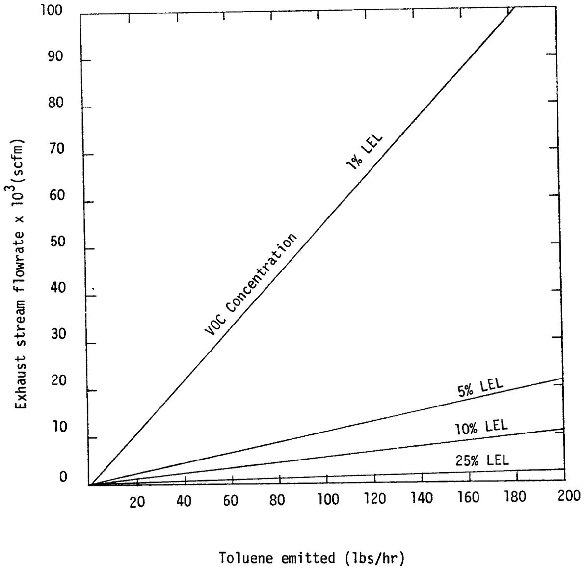
Figure 1-2. Data for toluene, LEL = 1.2% ( $\frac{V}{V}$ ), showing the relationship between VOC emission, exhaust flowrate and VOC concentration.
