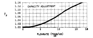
Installed pneumatic conveying system cost includes purchased cost of pneumatic conveying system components, blower, motor, base, coupling, check valve, filter, field erection, piping, concrete, steel, instrumentation, electrical, paint, and indirect costs (prime contractor engineering and construction overhead).
