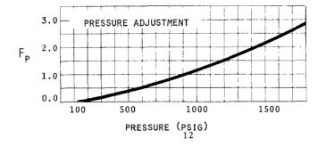
Installed agitated pressure tank cost includes purchased cost of agitated pressure tank (autoclaves include design by vendor, thermometer well, blow pipe,full vacuum rating), motor and drive, skirt, handling and setting, piping, concrete, steel, instrumentation, electrical, insulation, paint, and indirect costs (prime contractor engineering and construction overhead).
