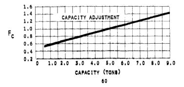
Installed elevator cost includes purchased cost of elevator, motor and drive, field erection by subcontractor, structural steel, subcontractors overhead and profit, indirect costs (prime contractor engineering and construction overhead).
