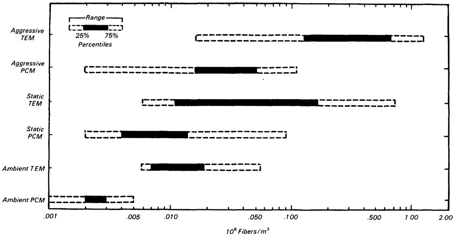
Figure 1. Comparison of airborne fiber concentrations measured by TEM and PCM under aggressive and static conditions.
