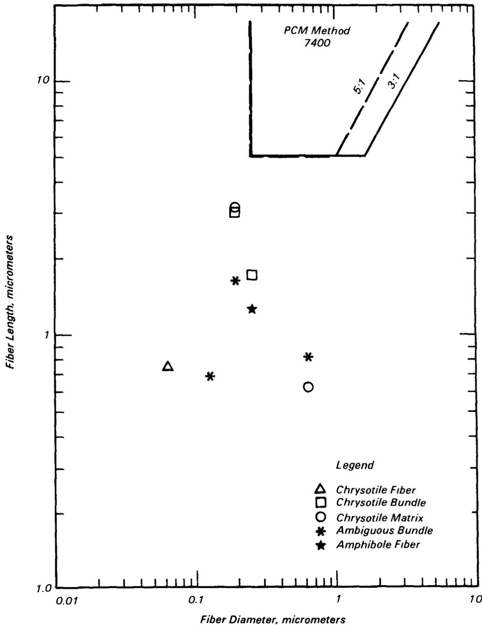
**Figure 4.** Results of TEM analysis under static conditions. Plot of fiber length and diameter for a static postabatement air sample in Room M112. Total asbestos structures/cc of air = 0.067.
