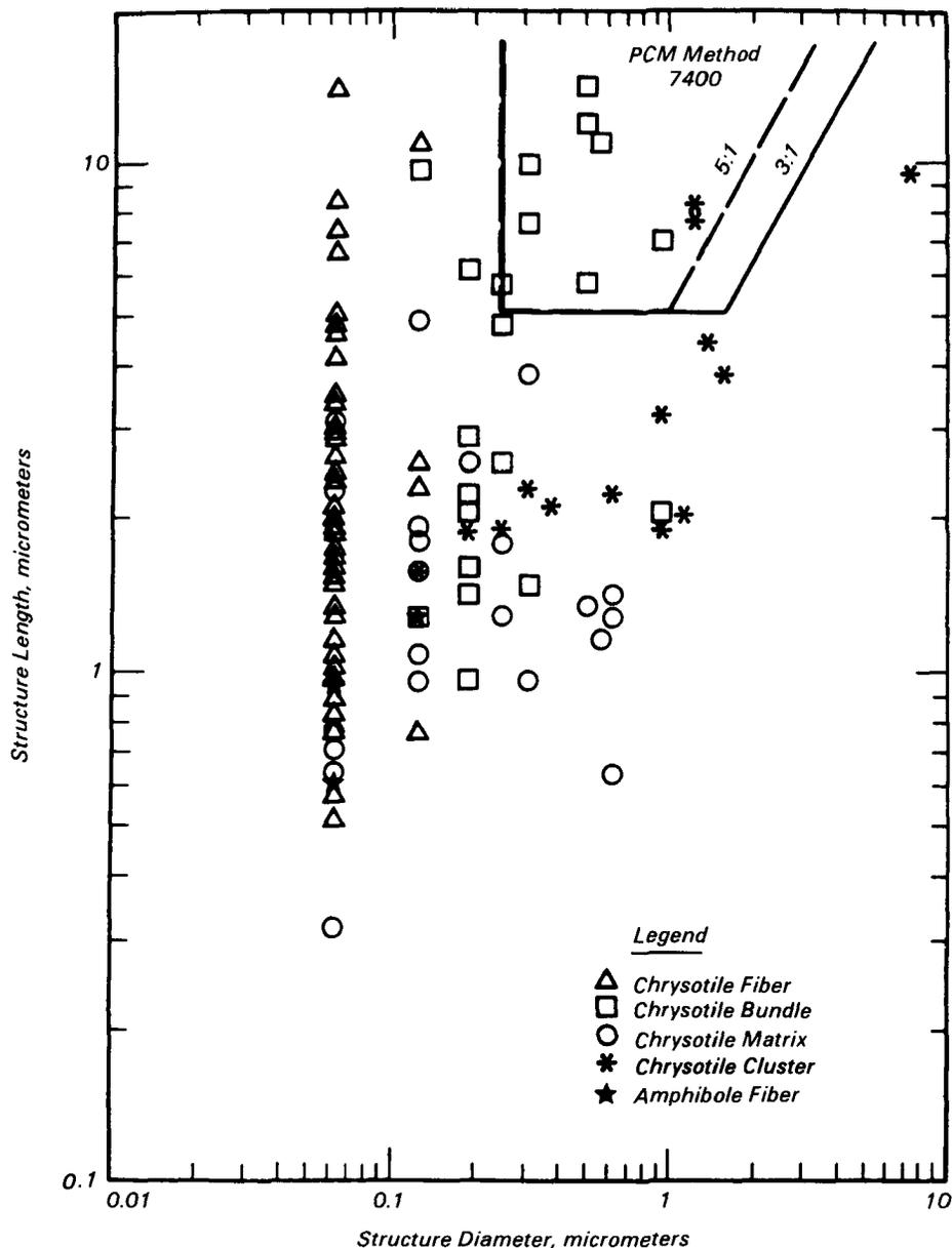
Figure 5. Results of TEM analysis under aggressive conditions. Plot of fiber length and diameter for an aggressive postabatement air sample in Room M112. Total asbestos structures/cc of air = 1.112.
