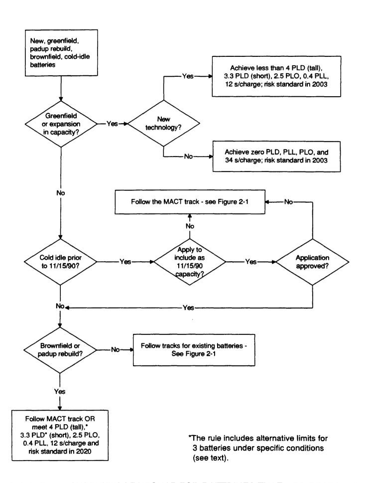
FIGURE 2-2. OVERVIEW OF NESHAP FOR BATTERIES THAT ARE RESTARTED
