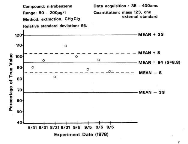
Figure 1. Control chart for nitrobenzene in reagent water.
