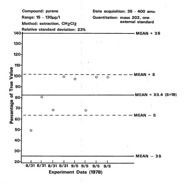
Figure 2. Control chart for pyrene in reagent water.
