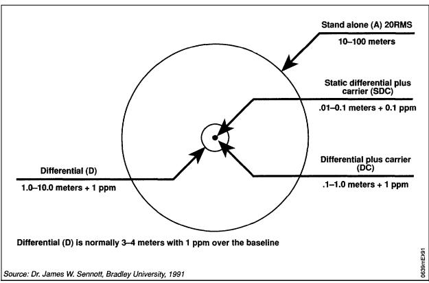
Figure 7. GPS operating modes and accuracy potential.
