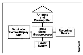
Figure 2. GPS receiver configuration.
