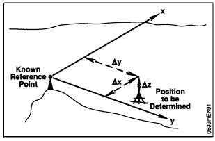
Figure 6. Relative positioning.
