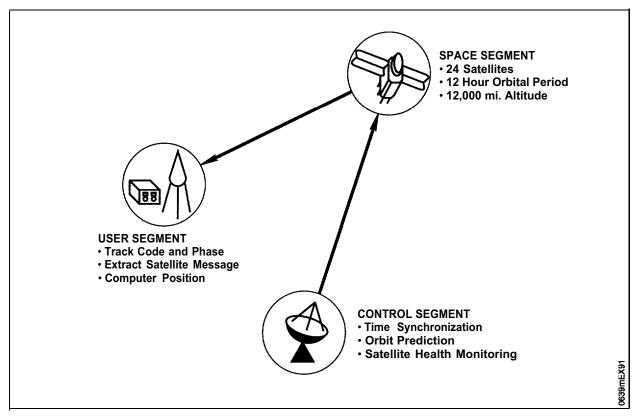
Figure 1. Three major components of the operational GPS complex.
