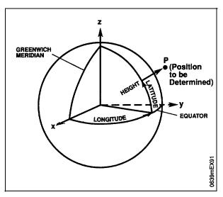
Figure 5. Point positioning.
