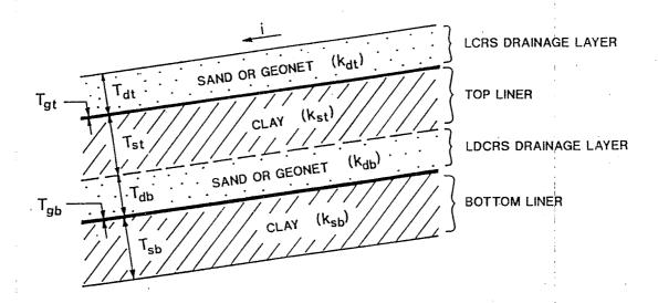
Figure 2. Definitions and terminology for double-liner system components.
