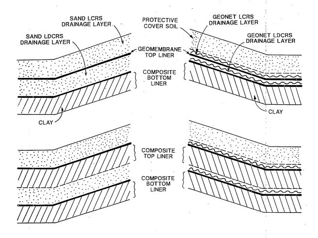
Figure 1. Typical double-liner systems for leachate containment in landfills.
