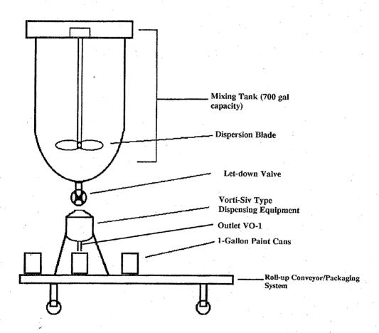
Figure 1. Paint manufacture schematic/packaging system.
