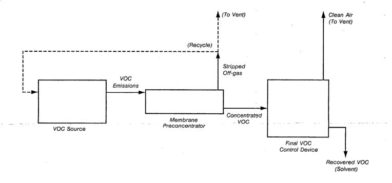
Figure 1. Membrane preconcentrator system..
