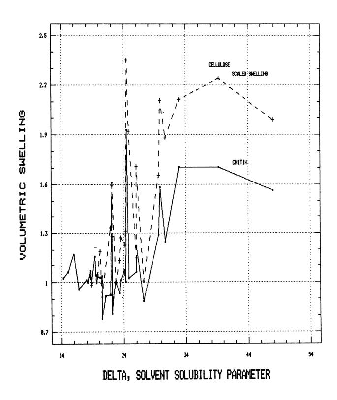
Figure 3. Swelling vs. 8, cellulose and chitin. This figure compares the swelling spectra for cellulose and chitin. The raw spectrum for cellulose was scaled by a constant factor so that the average background value of the swelling was shifted upwards to 1.0. No corrections for ash were applied to either spectrum.
