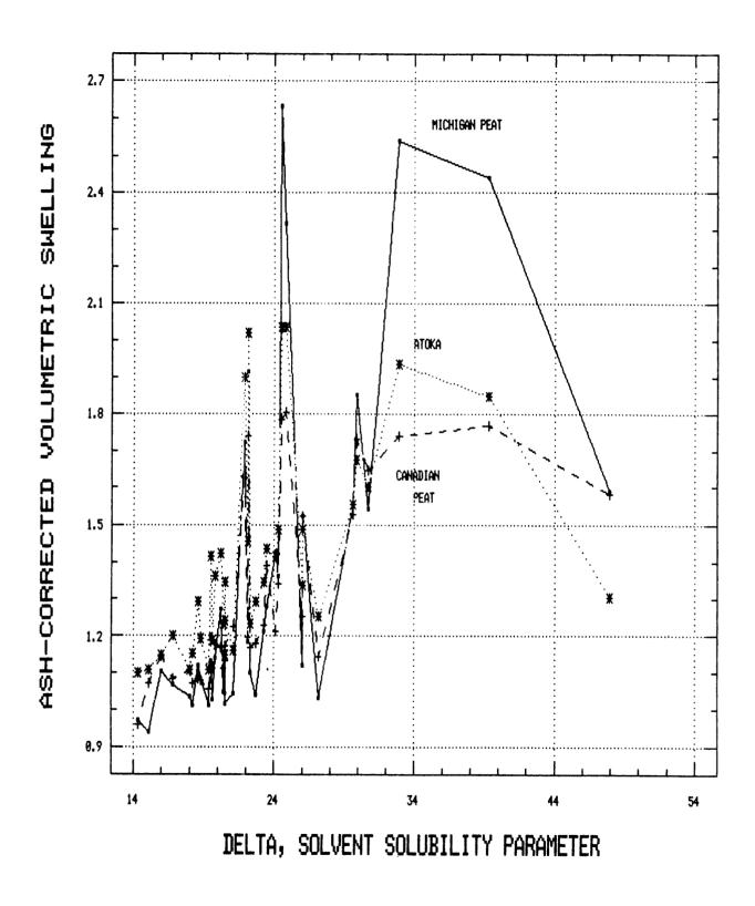
Figure 1. Ash-corrected swelling vs. δ<sub>σ</sub> peat-like materials. The swelling spectra for Michigan and Canadian peat and for the Atoka pine duff are compared in this figure after ash corrections.
