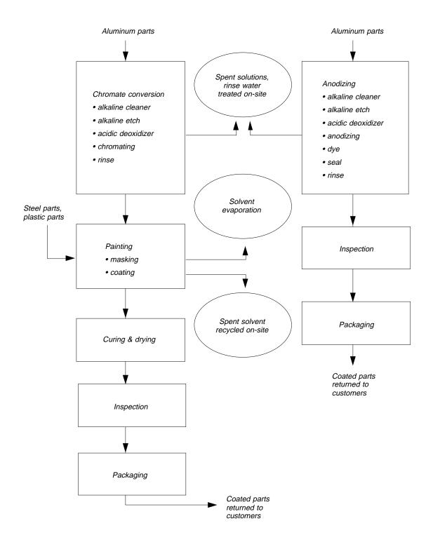
Figure 1. Abbreviated process flow diagram.
