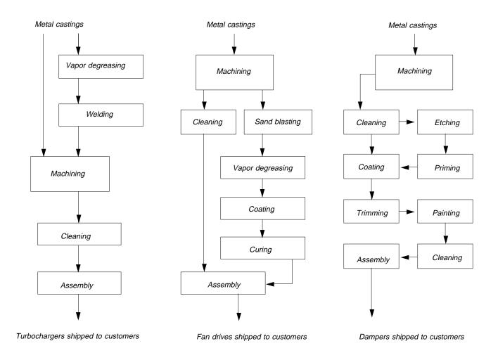
Figure 1. Abbreviated process flow diagram for truck engine parts manufacture.
