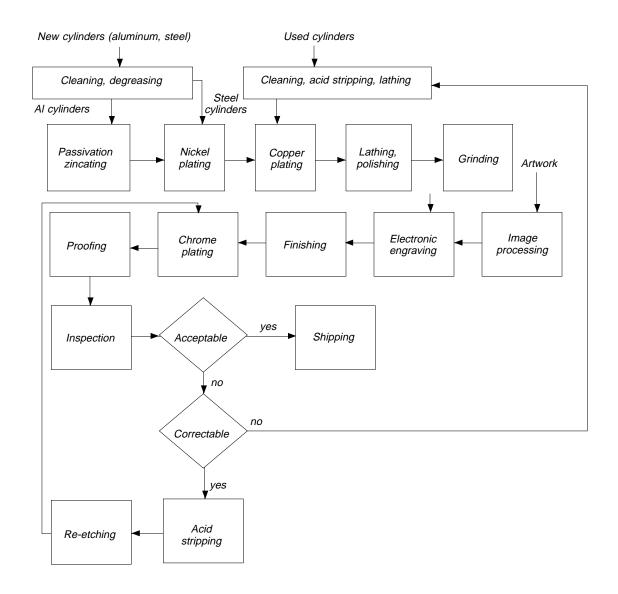
Figure 1. Abbreviated process flow diagram for rotogravure printing cylinders.
