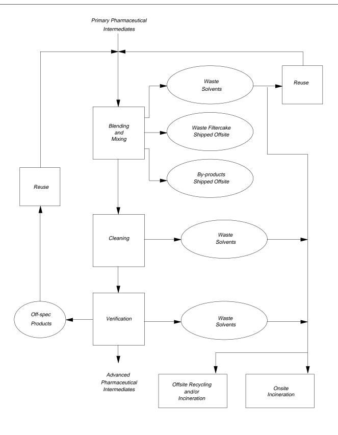
Figure 1. Abbreviated process flow diagram for pharmaceutical manufacture.
