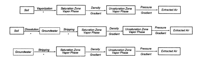
Figure 1. Mechanisms of mass transport during air sparging. (\* Mechanisms enhanced by air sparging.)
