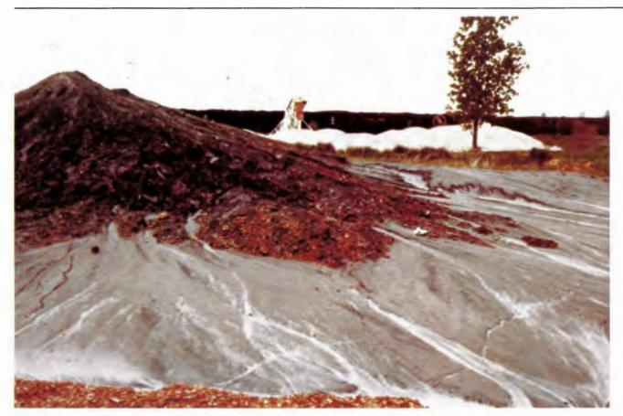
Gypsum filter cake at Site J, which shows signs of slumping and erosion 6 mo after placement
