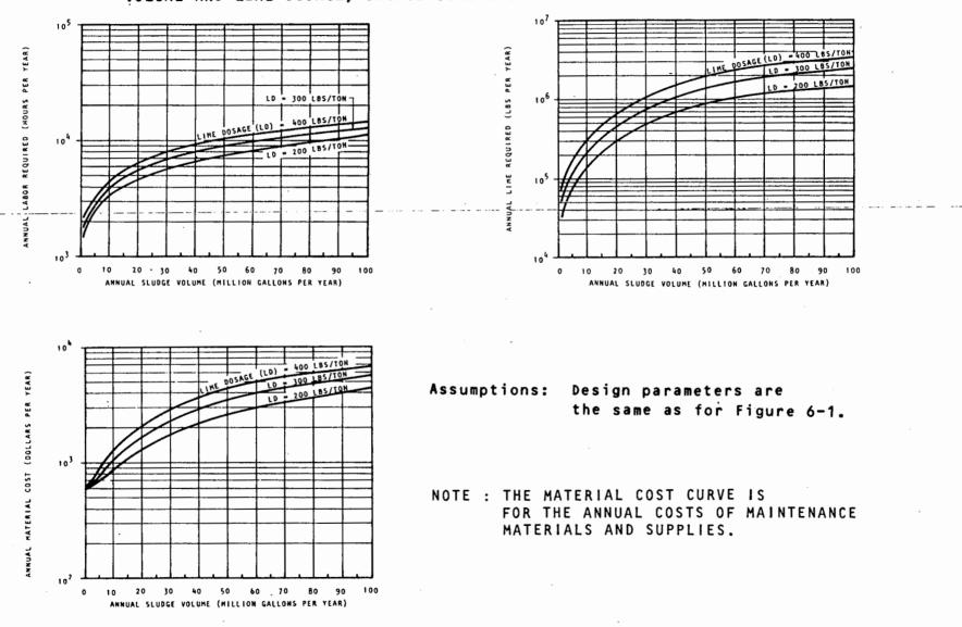
ANNUAL O&M REQUIREMENTS FOR CHEMICAL CONDITIONING WITH LIME AS A FUNCTION OF ANNUAL VOLUME AND LIME DOSAGE; SLUDGE SOLIDS CONCENTRATION = 2 PERCENT.
