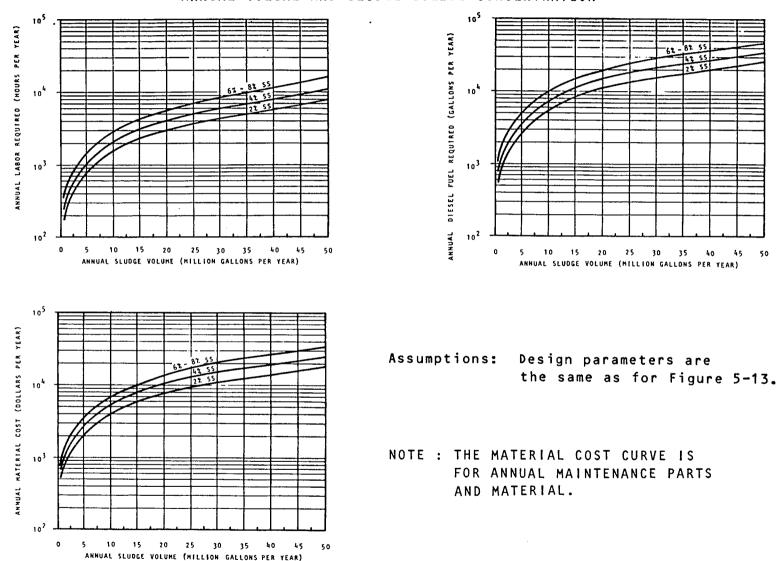
ANNUAL O&M REQUIREMENTS FOR SLUDGE DRYING BED DEWATERING AS A FUNCTION OF ANNUAL VOLUME AND SLUDGE SOLIDS CONCENTRATION
