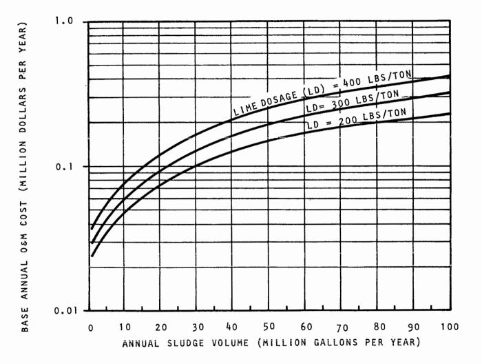
BASE ANNUAL 0&M COST OF CHEMICAL CONDITIONING WITH LIME AS A FUNCTION OF ANNUAL VOLUME AND LIME DOSAGE; SLUDGE SOLIDS CONCENTRATION = 4 PERCENT.
