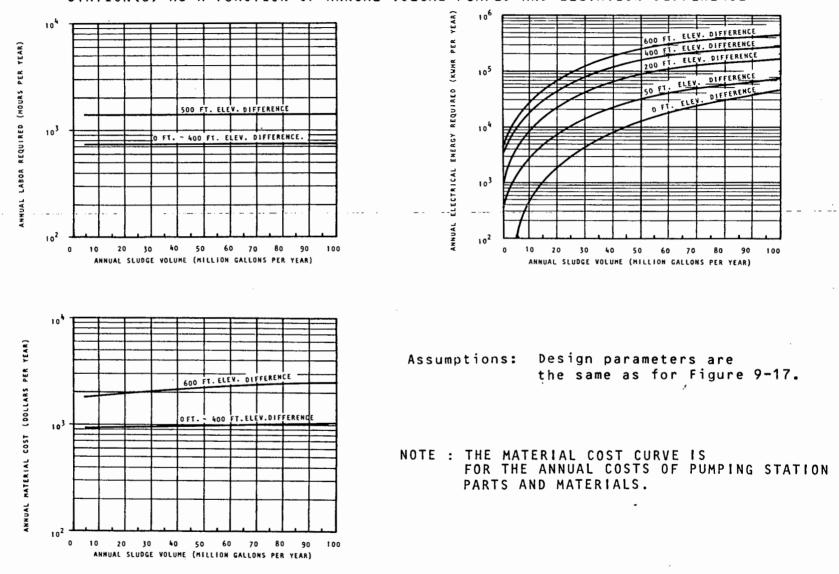
ANNUAL O&M REQUIREMENTS FOR A 1-MILE LIQUID SLUDGE TRANSPORT PIPELINE AND PUMP STATION(S) AS A FUNCTION OF ANNUAL VOLUME PUMPED AND ELEVATION DIFFERENCE
