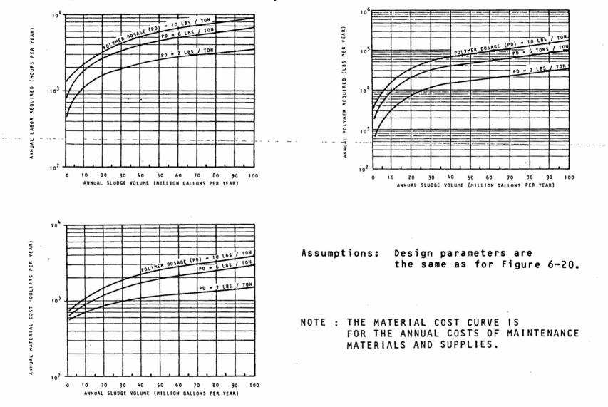
ANNUAL O&M REQUIREMENTS FOR CHEMICAL CONDITIONING WITH POLYMERS AS A FUNCTION OF ANNUAL VOLUME AND POLYMER DOSAGE; SLUDGE SOLIDS CONCENTRATION = 4 PERCENT.
