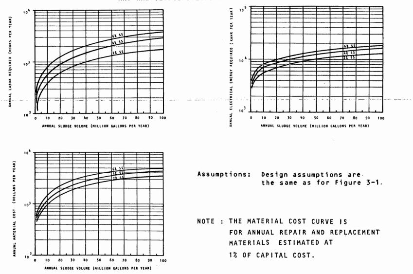
ANNUAL O&M REQUIREMENTS FOR GRAVITY THICKENING AS A FUNCTION OF ANNUAL VOLUME AND RAW SLUDGE SOLIDS CONCENTRATION
