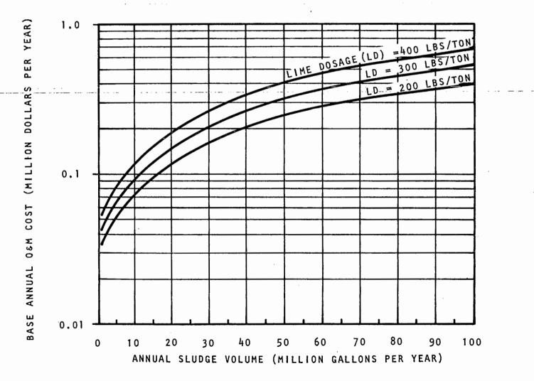
BASE ANNUAL O&M COST OF CHEMICAL CONDITIONING WITH LIME AS A FUNCTION OF ANNUAL VOLUME AND LIME DOSAGE; SLUDGE SOLIDS CONCENTRATION = 6 PERCENT.
