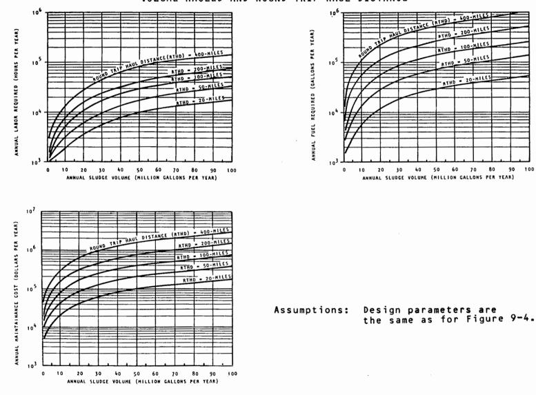
ANNUAL O&M REQUIREMENTS FOR DEWATERED SLUDGE TRUCK HAULING AS A FUNCTION OF ANNUAL VOLUME HAULED AND ROUND TRIP HAUL DISTANCE
