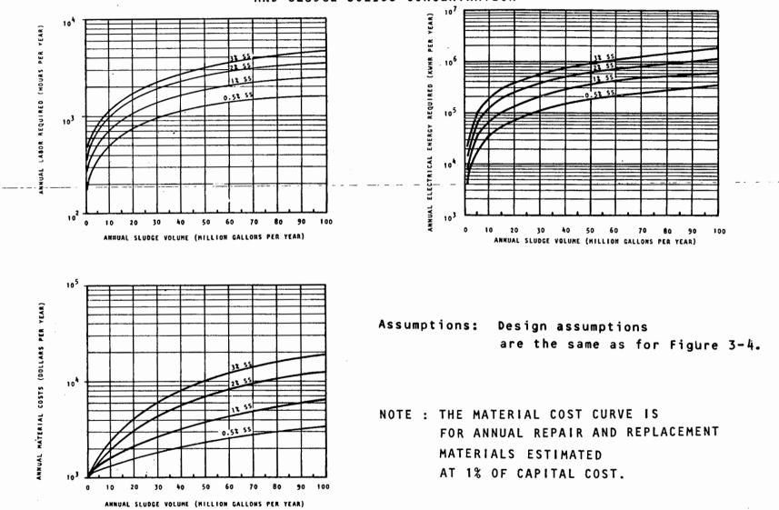
ANNUAL O&M REQUIREMENTS FOR FLOTATION THICKENING AS A FUNCTION OF ANNUAL VOLUME AND SLUDGE SOLIDS CONCENTRATION
