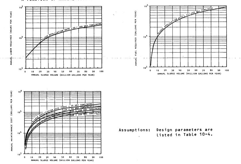
ANNUAL O&M REQUIREMENTS FOR APPLYING SLUDGE TO A DEDICATED DISPOSAL SITE AS A FUNCTION OF ANNUAL SLUDGE VOLUME APPLIED AND DRY SOLIDS APPLICATION RATE
