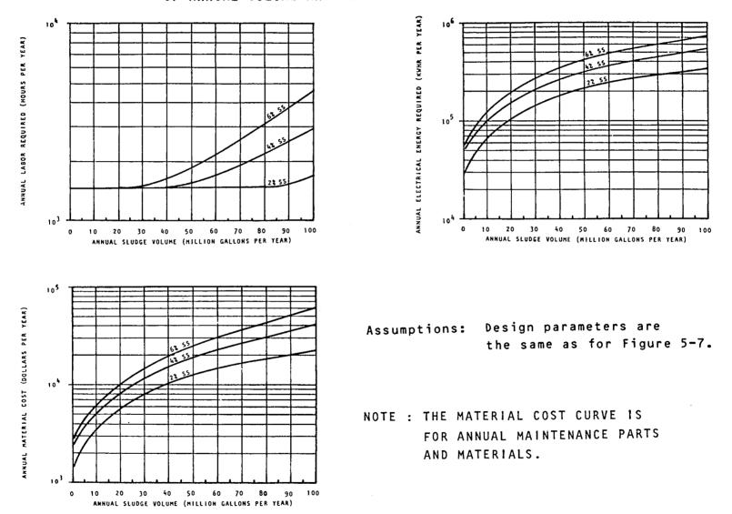
ANNUAL O&M REQUIREMENTS FOR RECESSED PLATE FILTER PRESS DEWATERING AS A FUNCTION OF ANNUAL VOLUME AND SLUDGE SOLIDS CONCENTRATION
