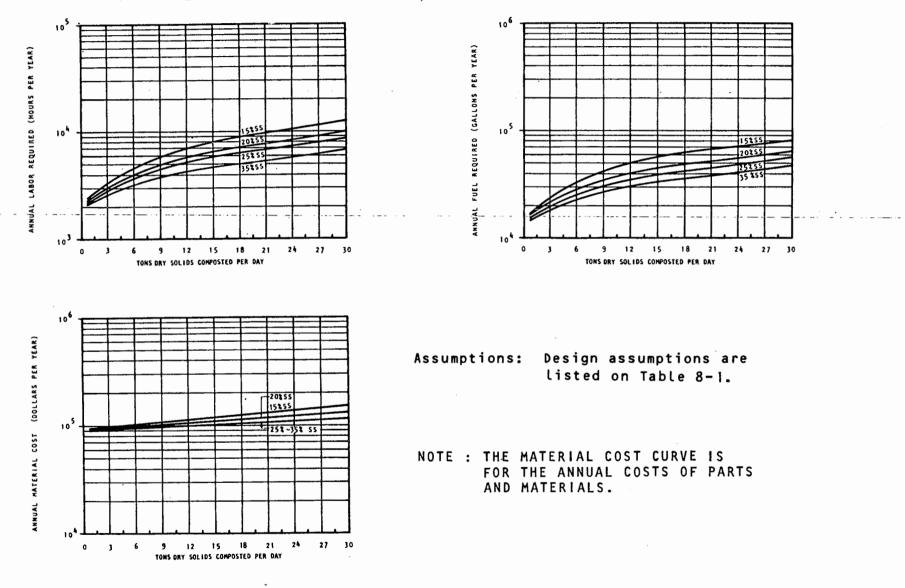
ANNUAL O&M REQUIREMENTS FOR WINDROW SLUDGE COMPOSTING AS A FUNCTION OF THE WEIGHT OF DRY SLUDGE SOLIDS COMPOSTED DAILY AND SLUDGE SOLIDS CONCENTRATION
