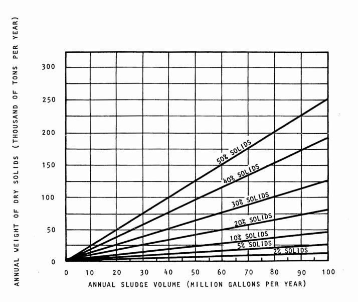
WEIGHT OF SLUDGE DRY SOLIDS CONTENT AS A FUNCTION OF WET SLUDGE VOLUME AND SOLIDS CONCENTRATION
