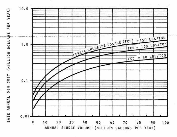
BASE ANNUAL 0&M COST OF CHEMICAL CONDITIONING WITH FERRIC CHLORIDE AS A FUNCTION OF ANNUAL VOLUME AND FERRIC CHLORIDE DOSAGE; SLUDGE SOLIDS CONCENTRATION = 6 PERCENT.
