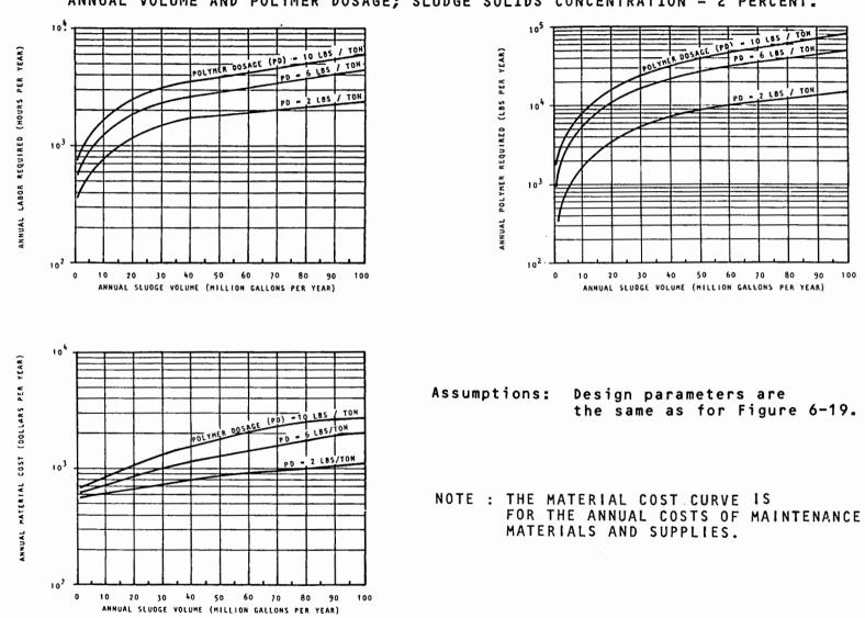
ANNUAL O&M REQUIREMENTS FOR CHEMICAL CONDITIONING WITH POLYMERS AS A FUNCTION OF ANNUAL VOLUME AND POLYMER DOSAGE; SLUDGE SOLIDS CONCENTRATION = 2 PERCENT.
