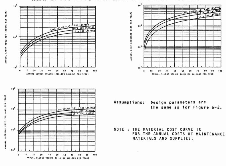
ANNUAL O&M REQUIREMENTS FOR CHEMICAL CONDITIONING WITH LIME AS A FUNCTION OF ANNUAL VOLUME AND LIME DOSAGE; SLUDGE SOLIDS CONCENTRATION = 4 PERCENT.
