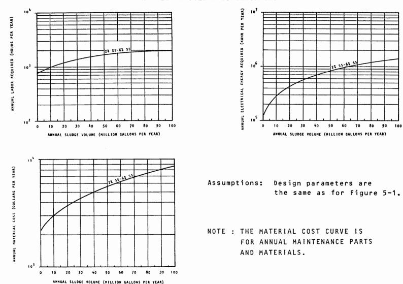
ANNUAL O&M REQUIREMENTS FOR CENTRIFUGE DEWATERING AS A FUNCTION OF ANNUAL VOLUME AND SLUDGE SOLIDS CONCENTRATION
