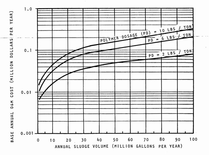
BASE ANNUAL O&M COST OF CHEMICAL CONDITIONING WITH POLYMERS AS A FUNCTION OF ANNUAL VOLUME AND POLYMER DOSAGE; SLUDGE SOLIDS CONCENTRATION = 4 PERCENT.
