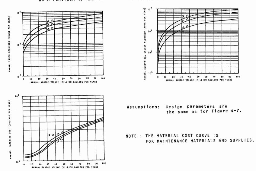
ANNUAL O&M REQUIREMENTS FOR AEROBIC DIGESTION USING DIFFUSED AERATION AS A FUNCTION OF ANNUAL VOLUME AND SLUDGE SOLIDS CONCENTRATION
