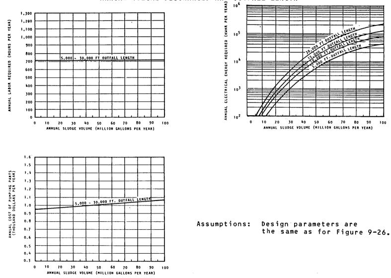
ANNUAL O&M REQUIREMENTS FOR A LIQUID SLUDGE OCEAN OUTFALL AS A FUNCTION OF ANNUAL VOLUME DISCHARGED AND OUTFALL LENGTH
