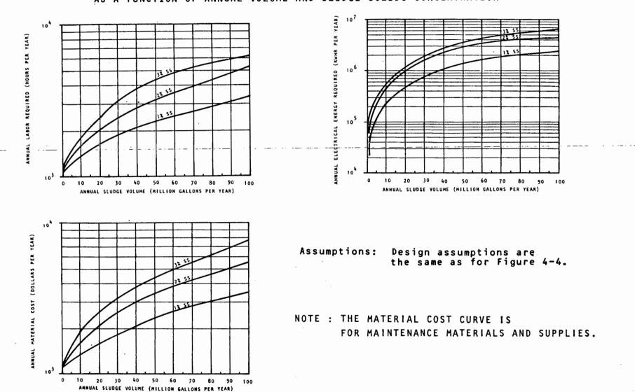
ANNUAL O&M REQUIREMENTS FOR AEROBIC DIGESTION USING MECHANICAL AERATORS AS A FUNCTION OF ANNUAL VOLUME AND SLUDGE SOLIDS CONCENTRATION
