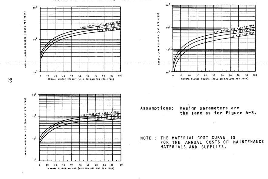
ANNUAL O&M REQUIREMENTS FOR CHEMICAL CONDITIONING WITH LIME AS A FUNCTION OF ANNUAL VOLUME AND LIME DOSAGE; SLUDGE SOLIDS CONCENTRATION ≈ 6 PERCENT.
