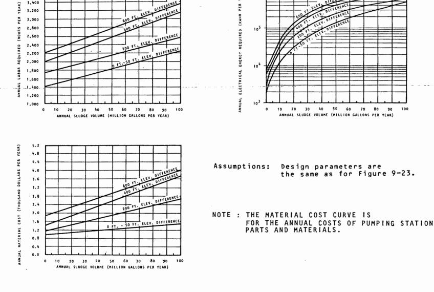
ANNUAL O&M REQUIREMENTS FOR A 10-MILE LIQUID SLUDGE TRANSPORT PIPELINE AND PUMP STATION(S) AS A FUNCTION OF ANNUAL VOLUME PUMPED AND ELEVATION DIFFERENCE
