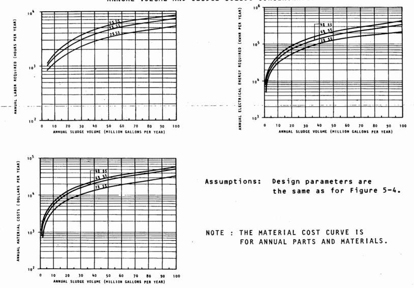
ANNUAL O&M REQUIREMENTS FOR BELT FILTER PRESS DEWATERING AS A FUNCTION OF ANNUAL VOLUME AND SLUDGE SOLIDS CONCENTRATION
