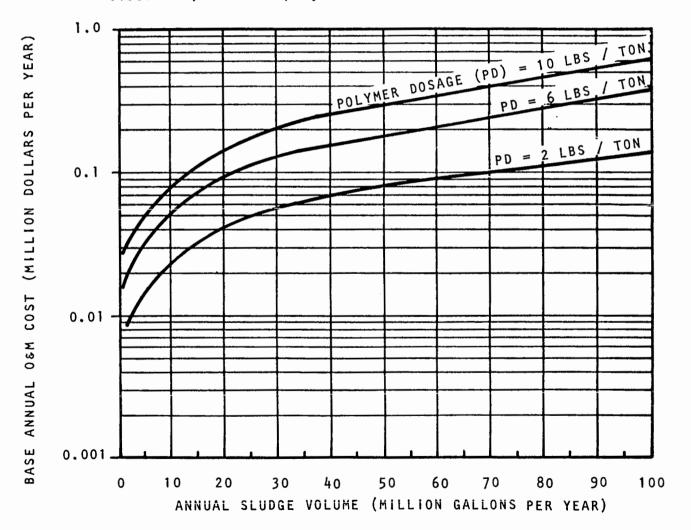
BASE ANNUAL O&M COST OF CHEMICAL CONDITIONING WITH POLYMERS AS A FUNCTION OF ANNUAL VOLUME AND POLYMER DOSAGE; SLUDGE SOLIDS CONCENTRATION = 6 PERCENT.
