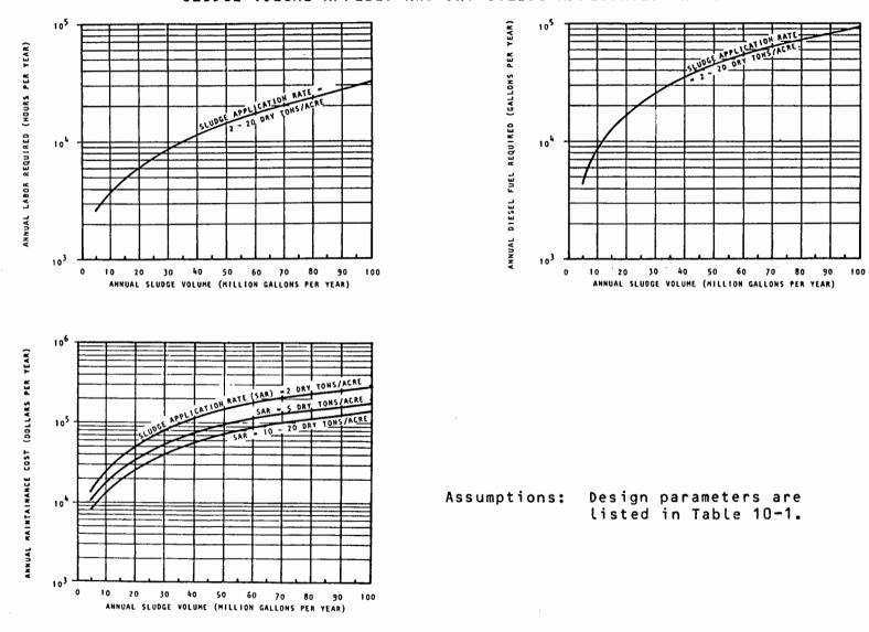
ANNUAL O&M REQUIREMENTS FOR APPLYING SLUDGE TO CROPLAND AS A FUNCTION OF ANNUAL SLUDGE VOLUME APPLIED AND DRY SOLIDS APPLICATION RATE
