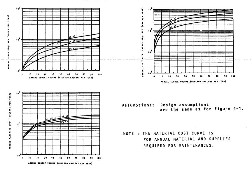
ANNUAL O&M REQUIREMENTS FOR ANAEROBIC DIGESTION AS A FUNCTION OF ANNUAL VOLUME AND SLUDGE SOLIDS CONCENTRATION
