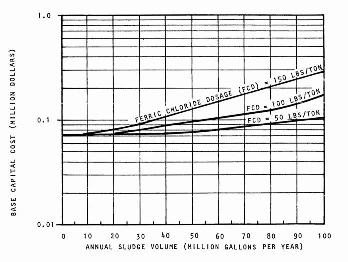
BASE CAPITAL COST OF CHEMICAL CONDITIONING WITH FERRIC CHLORIDE AS A FUNCTION OF ANNUAL VOLUME AND FERRIC CHLORIDE DOSAGE; SLUDGE SOLIDS CONCENTRATION = 6 PERCENT.
