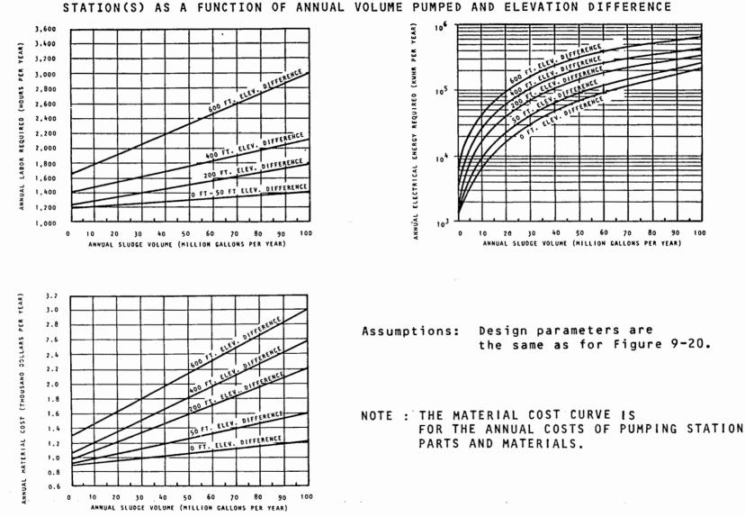
ANNUAL O&M REQUIREMENTS FOR A 5-MILE LIQUID SLUDGE TRANSPORT PIPELINE AND PUMP STATION(S) AS A FUNCTION OF ANNUAL VOLUME PUMPED AND ELEVATION DIFFERENCE
