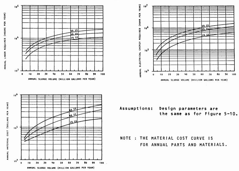
ANNUAL O&M REQUIREMENTS FOR VACUUM FILTER DEWATERING AS A FUNCTION OF ANNUAL VOLUME AND SLUDGE SOLIDS CONCENTRATION
