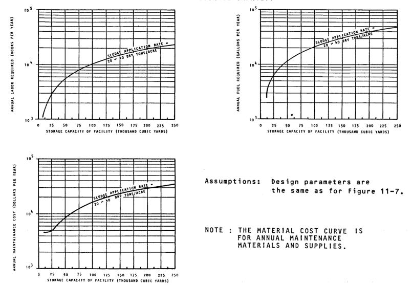
ANNUAL O&M REQUIREMENTS FOR UNCONFINED PILE DEWATERED SLUDGE STORAGE AS A FUNCTION OF FACILITY STORAGE CAPACITY
