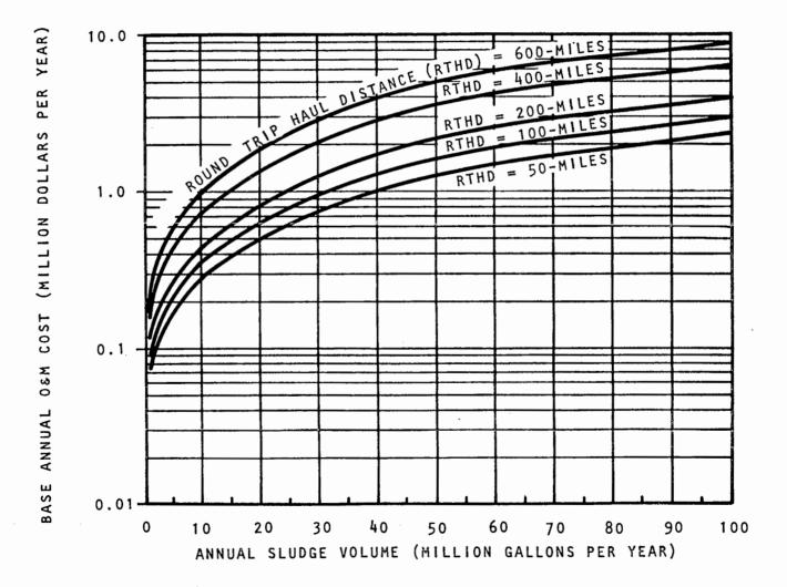
NORTHEAST REGION: BASE ANNUAL O&M COST OF LIQUID SLUDGE RAIL HAULING AS A FUNCTION OF ANNUAL VOLUME HAULED AND ROUND TRIP HAUL DISTANCE
