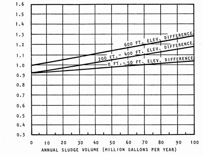
BASE ANNUAL O&M COST OF A 5-MILE LIQUID SLUDGE TRANSPORT PIPELINE AND PUMP STATION(S) AS A FUNCTION OF ANNUAL VOLUME PUMPED AND ELEVATION DIFFERENCE
