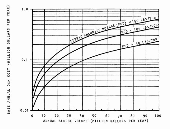
BASE ANNUAL 0&M COST OF CHEMICAL CONDITIONING WITH FERRIC CHLORIDE AS A FUNCTION OF ANNUAL VOLUME AND FERRIC CHLORIDE DOSAGE; SLUDGE SOLIDS CONCENTRATION = 4 PERCENT.
