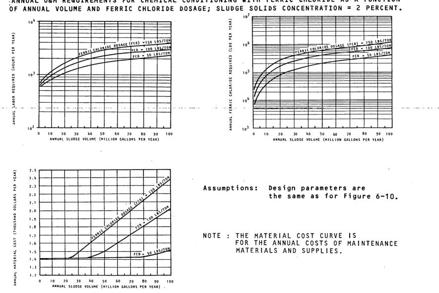
ANNUAL O&M REQUIREMENTS FOR CHEMICAL CONDITIONING WITH FERRIC CHLORIDE AS A FUNCTION
