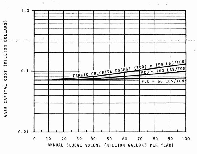
BASE CAPITAL COST OF CHEMICAL CONDITIONING WITH FERRIC CHLORIDE AS A FUNCTION OF ANNUAL VOLUME AND FERRIC CHLORIDE DOSAGE; SLUDGE SOLIDS CONCENTRATION = 4 PERCENT.
