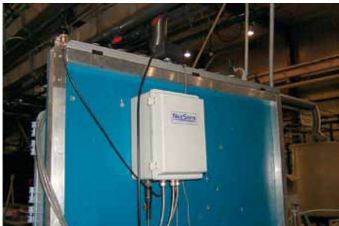
Figure 2.11 NexSens iSIC Data Acquisition System
