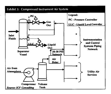
The major components of an instrument air conversion project include the compressor, power source, dehydrator, and volume tank. The following are descriptions of each of these components along with important installation considerations.
