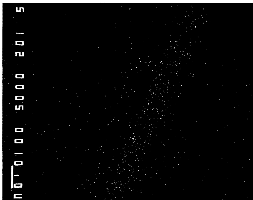
Figure 22b X-ray DOT mapping of magnesium layer.
