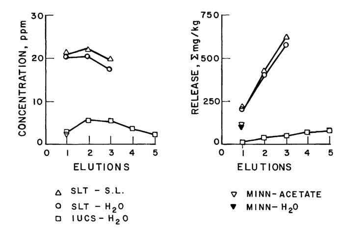
Figure 3. Napthalene concentration and release from a coal tar waste in test leachates.
