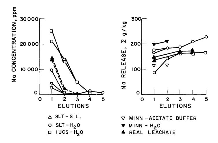
Figure 4. Na concentration and release from a  $\text{CuO-Na}_2\text{SO}_4$  sludge in test leachates.
