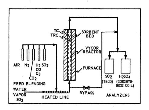
(THE BYPASS IS LOCATED AFTER THE WATER VAPOR + SO3 ARE ADDED.)
