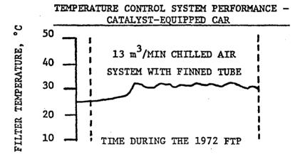
above 32°C during the steep acceleration portion of the driving cycle. It should be noted that the system is designed to prevent temperature excursions above 32°C, not to maintain that temperature during the course of the entire run.
