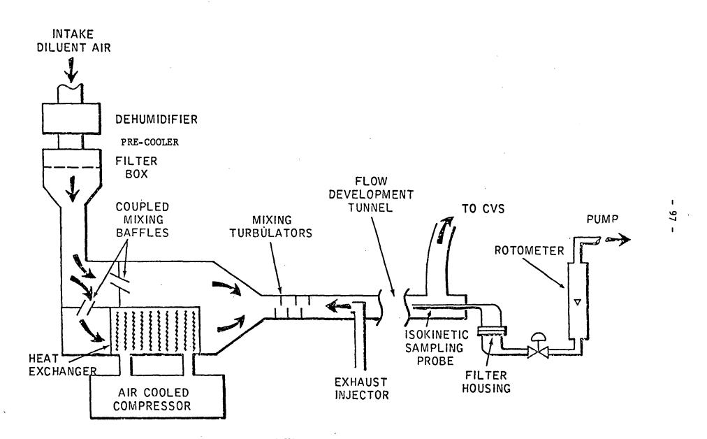
The overall function of this system is to allow the collection of particulate matter from an isokinetically sampled portion of diluted exhaust which has been cooled to 32°C by dilution with chilled, dehumidified, filtered air. The function of each of the components in accomplishing this objective is described below.
