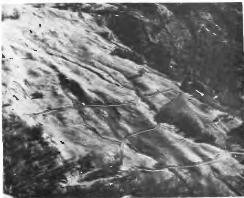
Figure V.5.—An example of soil creep and slump-earthflow processes on forest lands in northern California. The entire slope is undergoing creep deformation, but note the discrete failure (slump-earthflow) marked by the steep headwall scarp at top center and the many small slumps and debris avalanches triggered by surface springs and road construction.
