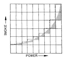
Figure 2. Smoke versus power output of typical naturally aspirated engines.
