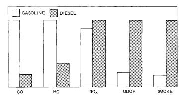
Figure 1. Relative levels of pollutants emitted by gasoline- and diesel-powered vehicles.
