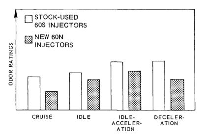
Figure 7. Effect of injector type on odor.
