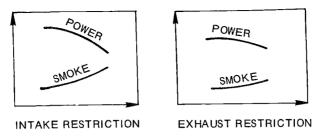
Figure 5. General effect of intake and exhaust restriction on smoke and power.
