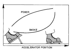
Figure 6. Smoke and power as affected by accelerator position.
