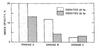
Figure 4. Effect of engine derating on exhaust smoke from three moderate- to high-smoke engines.
