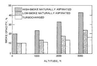
Figure 3. General effect of altitude on hot smoke production by diesel engines.
