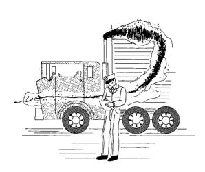
Another way in which the drive and only the driver can reduce odor is to minimize idle time and light-load operation. Unburned fuel and products of combustion from some engines condense in the exhaust, particularly during warmup or shortly after engine startup, and a more intense odor may result. A good rule is to start the en-
