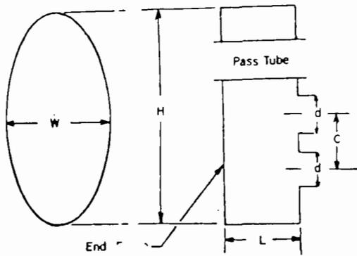
Figure 18. Flow-Reversing Chamber With Pass Tube and End Plate. C — Distance Between Centers of Inlet and Outlet Tubes; H — Height of Chamber; L — Length of Chamber; W — Width of Chamber; and d — pipe Diameter
