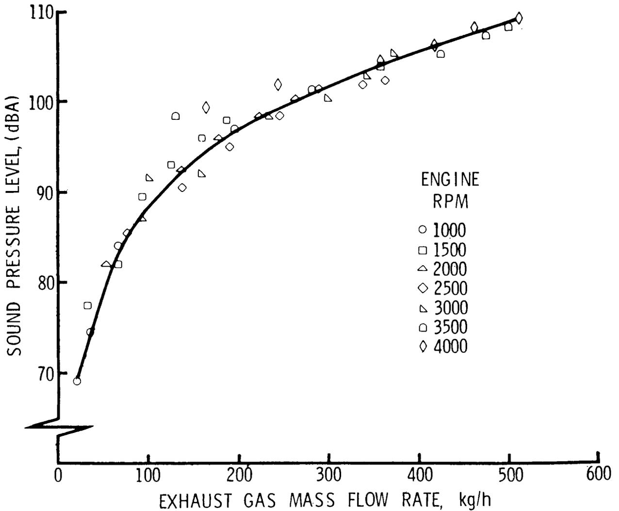
Figure 3. Radiated Exhaust Noise Versus Exhaust Gas Mass Flow Rate for a V-8 Engine.
