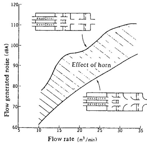
Fig. 12 Reduction of flow generated noise by horn type extension pipe of test muffler for vehicles
