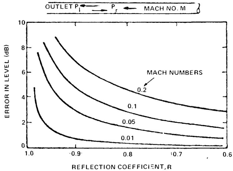
Figure 5. Radiated Sound Pressure Level Error Due to Neglect of Mean Flow,  $P_r = R \cdot P_e^{i\theta}$ . Radiated Sound Pressure Level Calculated Neglecting Mean Flow is Low by the Amount Given Here as Error
