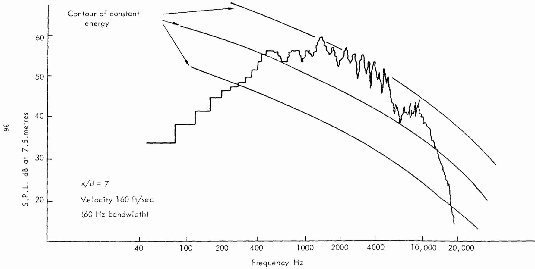
FIG. 5. SPECTRAL CONTENT OF FLOW NOISE
