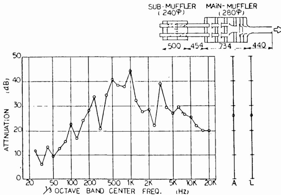
FIG-10 EXAMPLE OF ACOUSTIC ATTENUATION OF MUFFLER
