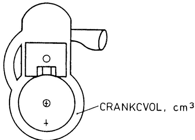
Fig.2 Crankshaft position shown at bottom dead centre, B.D.C. - note all transfer ducts are open, and the volume under the piston is then the crankcase clearance volume, measured in  $\text{Cm}^3$ . If SV is the swept volume per cylinder,  $\text{Cm}^3$  then -
