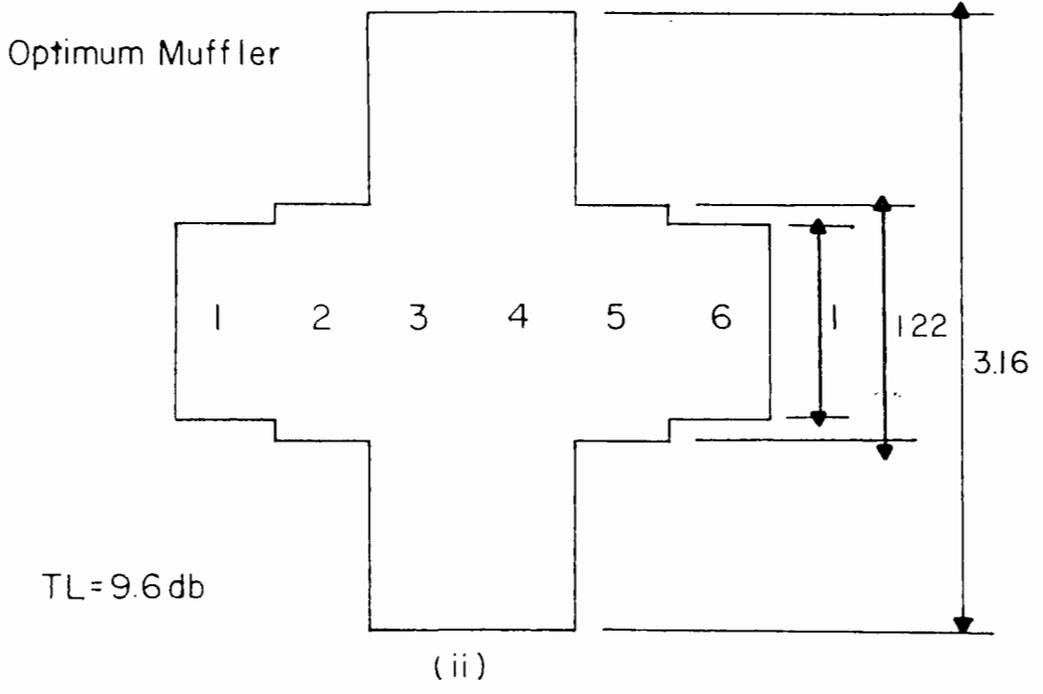
FIG.(5-a) Six Segment Reactive Muffler
