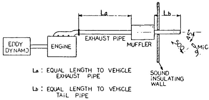
FIG-28 DIAGRAM OF EXHAUST NOISE TEST ON A ENGINE BENCH
