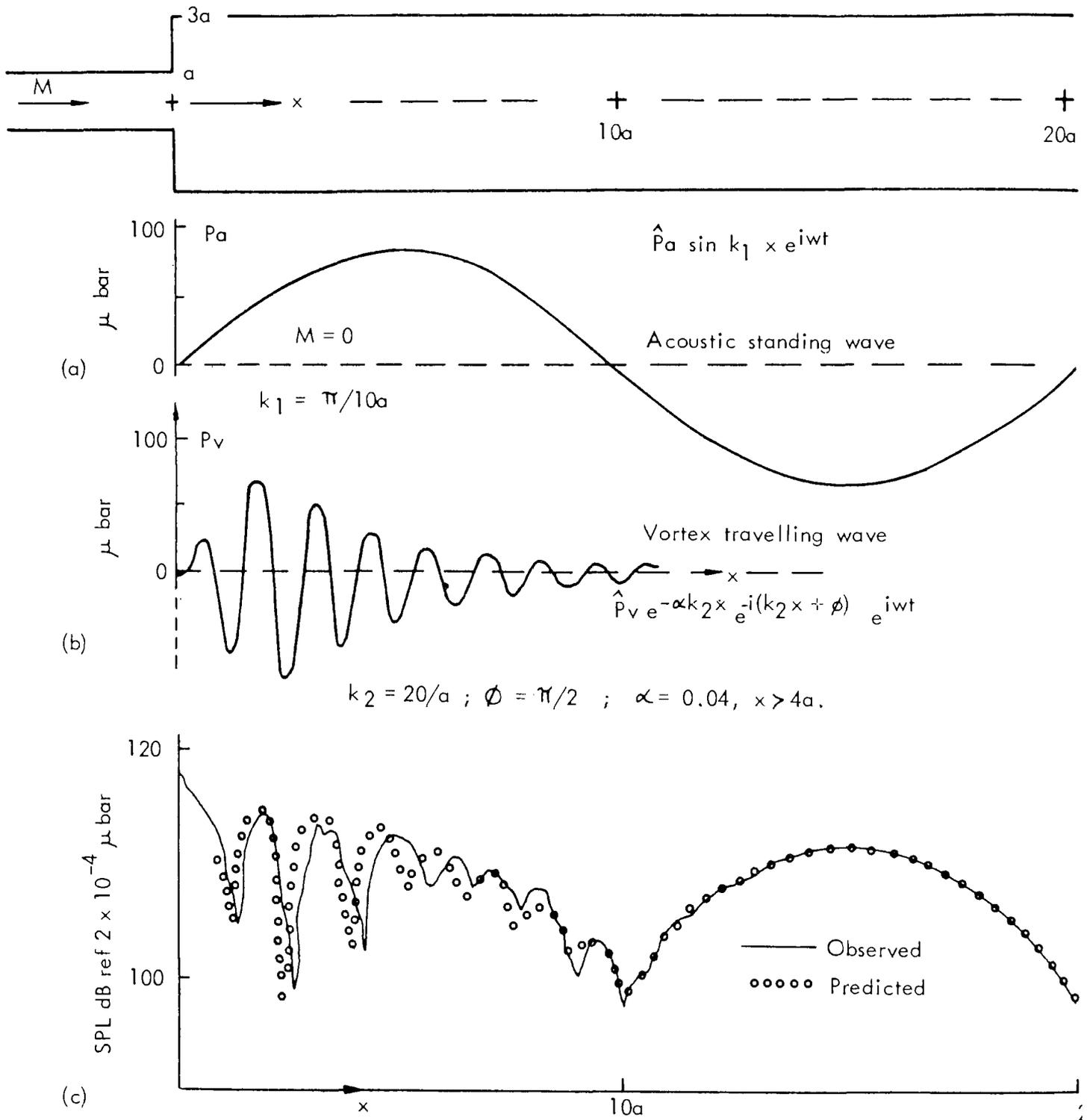
FIG. 11 SOUND PRESSURE LEVEL AFTER A DUCT EXPANSION  $M = 0.1$  ;  $f = 1250\text{Hz}$
