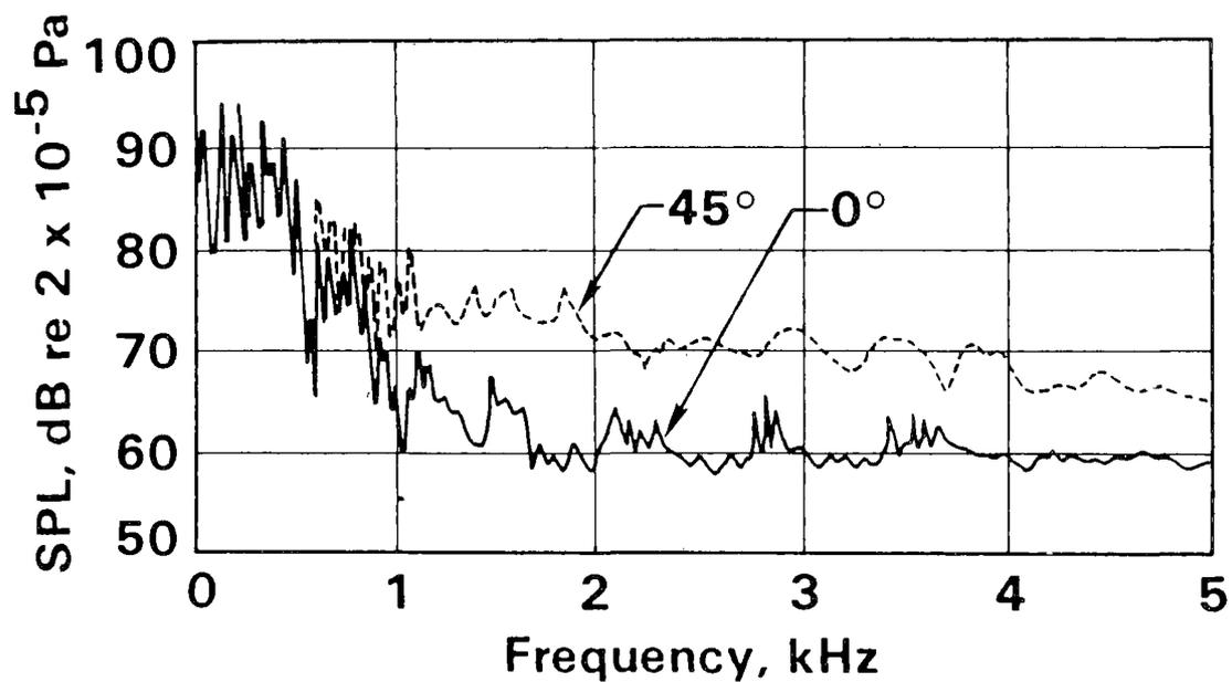
Figure 6. Exhaust Noise Spectra at 0° and 45° from the Tailpipe Axis and 1.5 m from the End of the Tailpipe.
