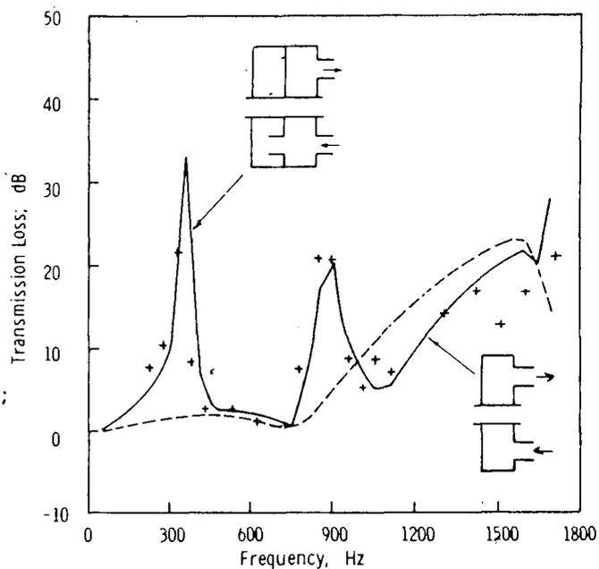
Figure 23. Transmission loss characteristics for SI-CO muffler chambers: - - - flow-reversing chamber only - predicted; — flow-reversing chamber and resonator - predicted; and + is the measured data for the flow-reversing chamber and resonator
