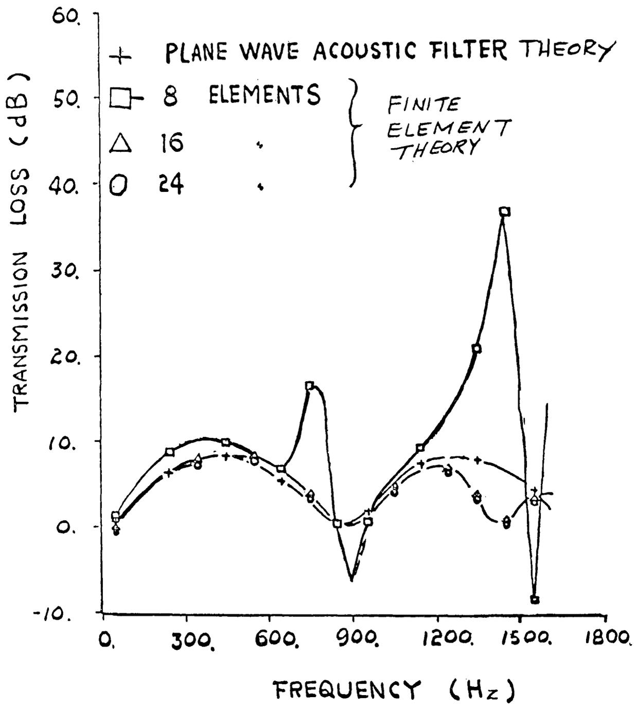
Figure 17. Transmission Loss of Simple Expansion Chamber,  $\ell = 8.0$  in.,  $m = 5$  in.
