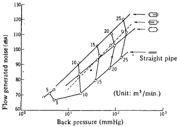
Fig. 9 Flow generated noise of expansion type mufflers
