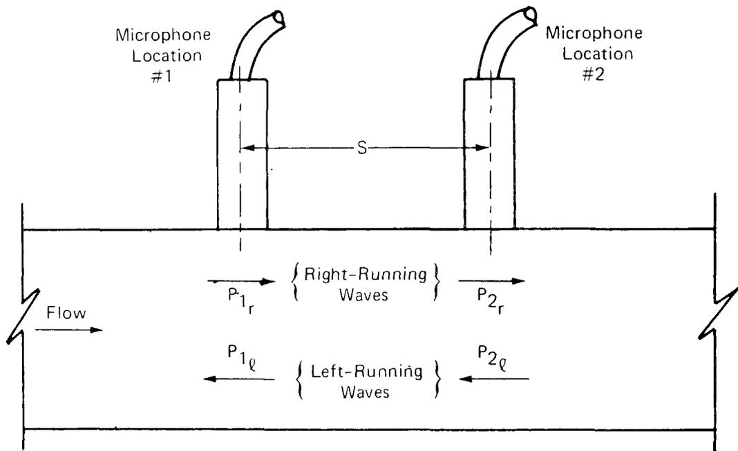
Figure 8. Microphone Configuration and Notation.
