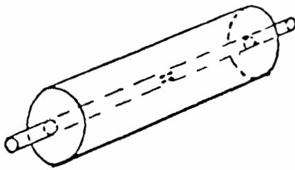
Figure 1c. Single Chamber Resonator
