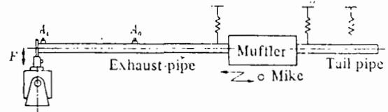
Fig. 15 Testing system of radiated noise from exhaust system
