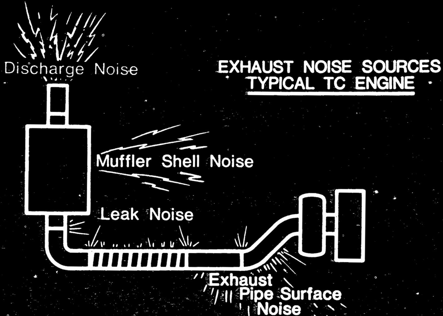
**Discharge + Muffler + Leak + Pipe noises = Exhaust Noise**
