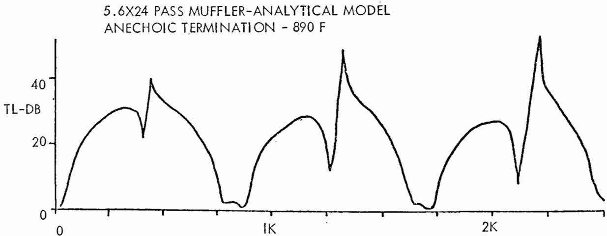
Figure 15. Analytical and Experimental Results for a Pass Muffler.
