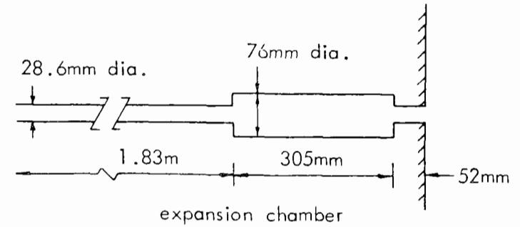
FIG. 13 SINGLE EXPANSION CHAMBER PERFORMANCE CONSTANT VOLUME VELOCITY SOURCE LINEAR ACOUSTIC ANALYSIS
