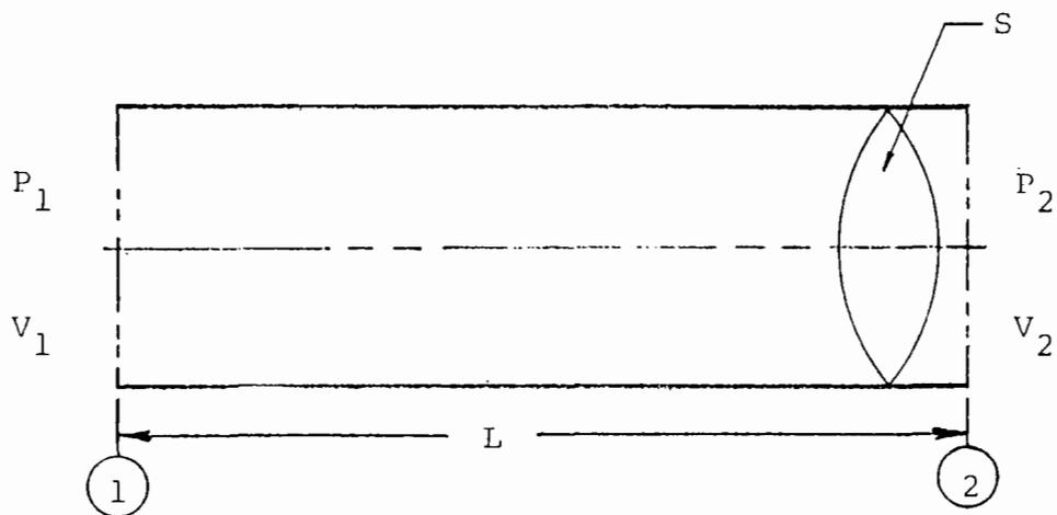
Figure 2. Straight pipe of length  $L$  with acoustical variables  $P_1$  and  $V_1$  at the pipe entrance, and  $P_2$  and  $V_2$  at the pipe exit.
