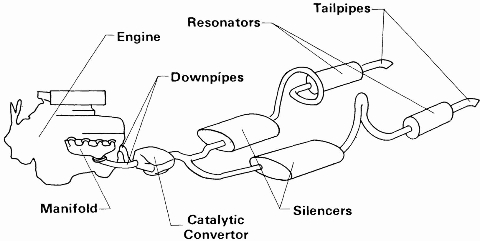
Figure 1. Components of an Engine Exhaust System.
