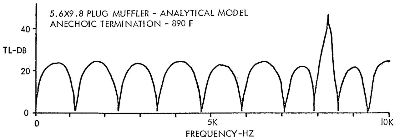
Figure 16. Analytical and Experimental Results for a Plug Muffler.
