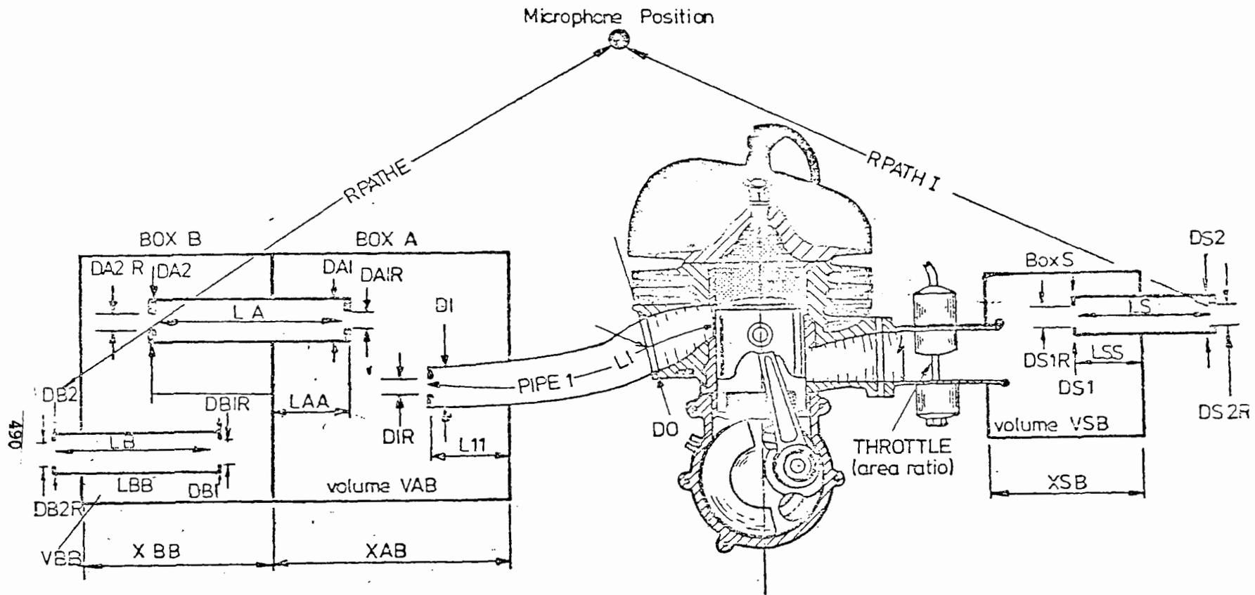
Program: G.P.B. 3 EXHAUST AND INTAKE SILENCING BOX PARAMETERS REQUIRED FOR PROGRAM
