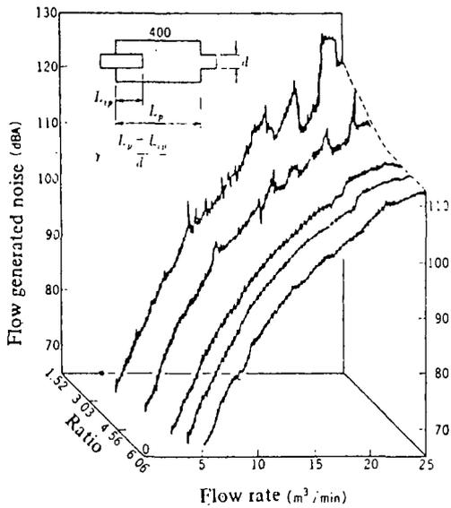
Fig. 8 Effect of the gap of inlet and outlet expansion pipe to flow generated noise
