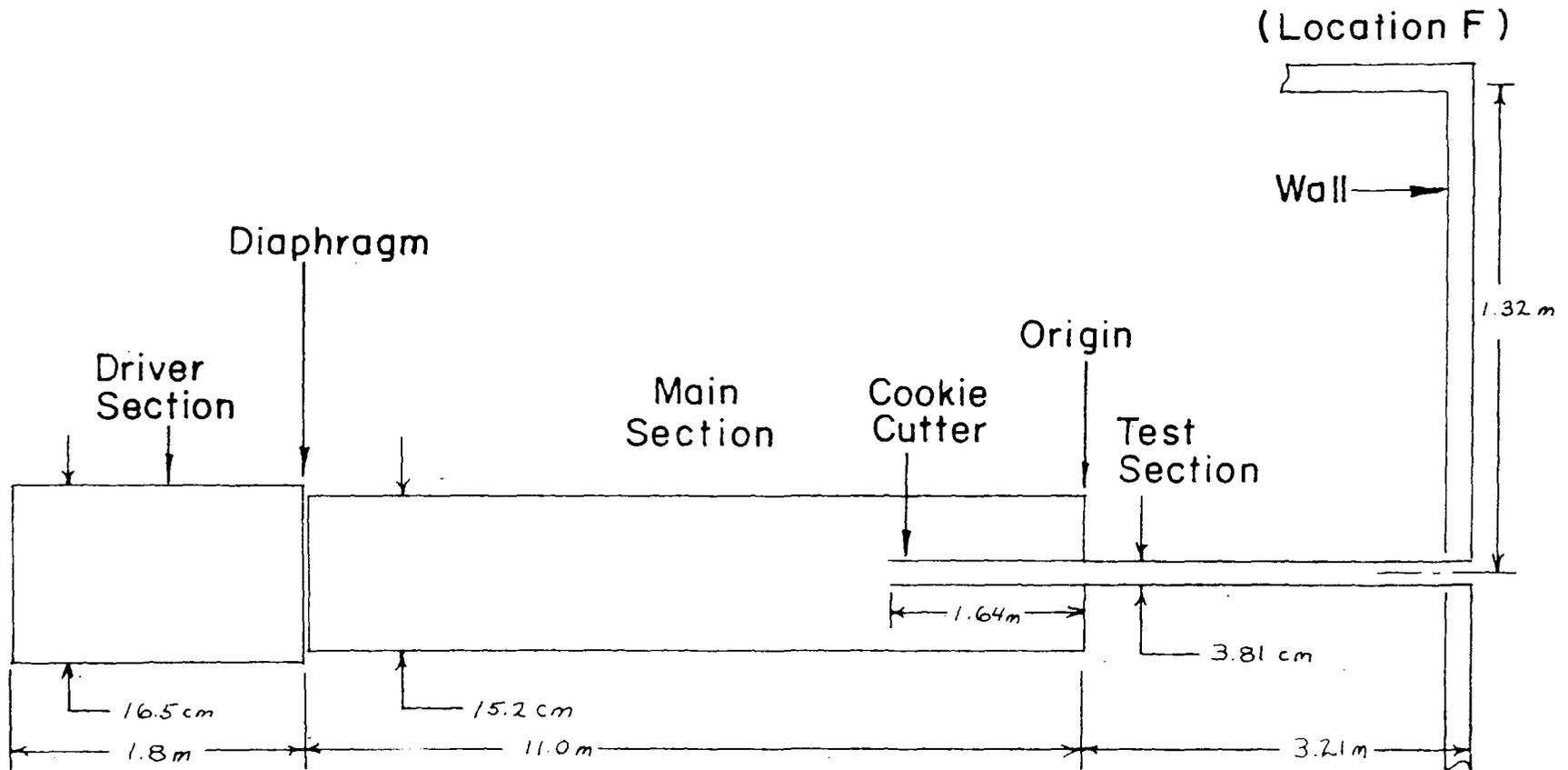
FIGURE 4 GALCIT SIX INCH SHOCK TUBE
