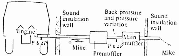
Fig. 19 Experimental layout for the test of exhaust system noise of vehicle
