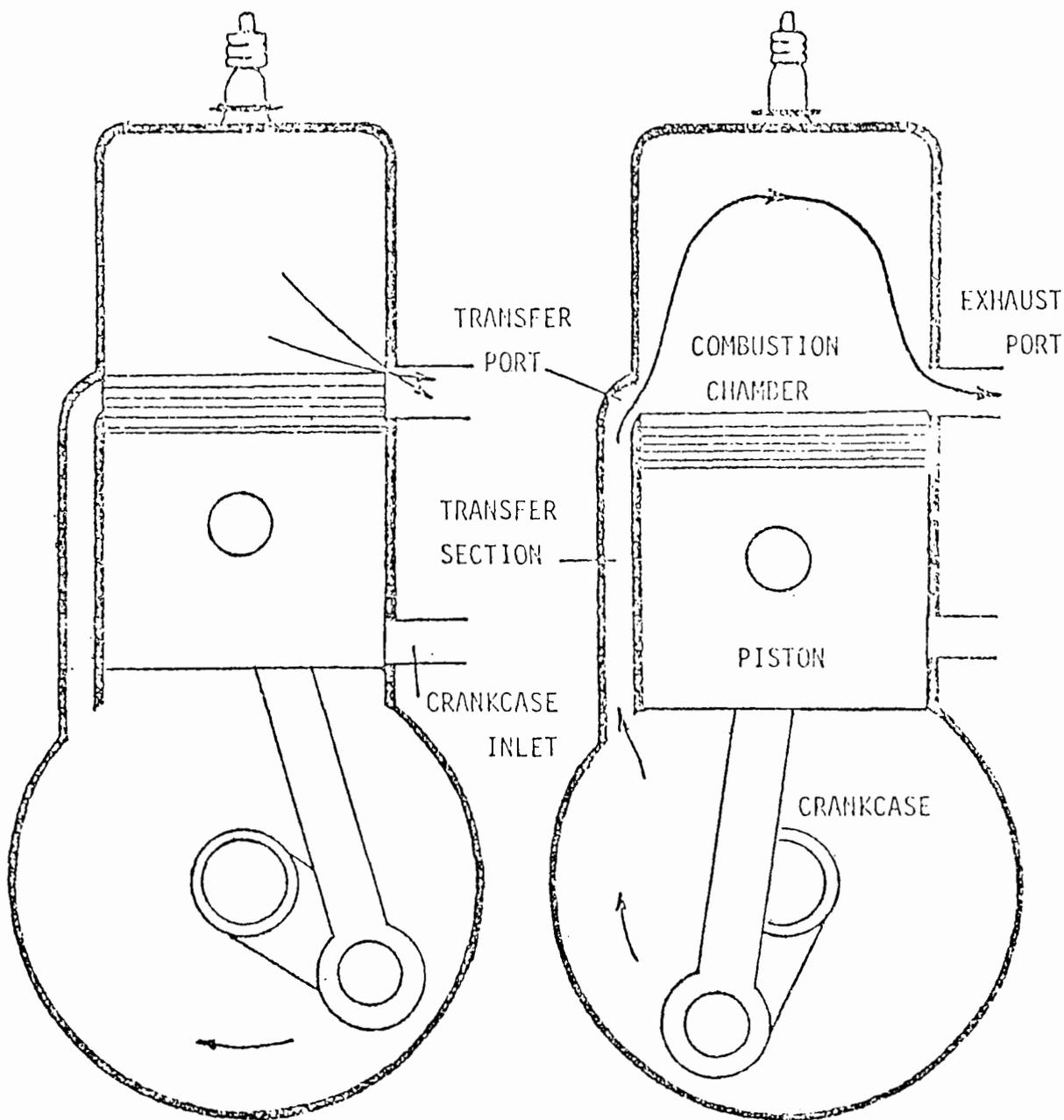
SCHEMATIC DIAGRAM OF TWO STROKE ENGINE OPERATION
