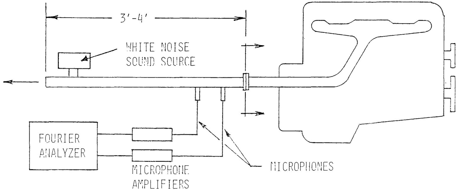
Figure 8. Measurement of engine source impedance.
