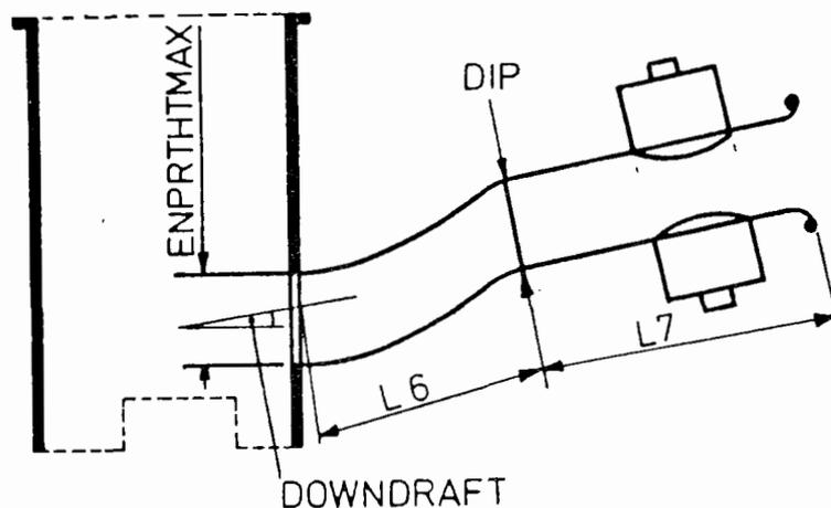
Fig.7 Section through inlet tract for piston-port induction system.
