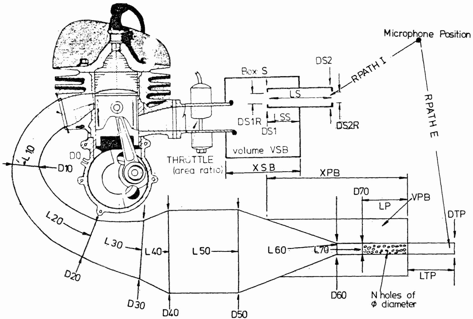
EXHAUST AND INTAKE SILENCING BOX PARAMETERS REQUIRED FOR PROGRAM FILE GPB 6 (moto -cross motorcycle), FOR PROGRAM FILE GPB 7 (for road racing no intake silencer S)
