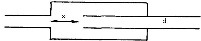
FIG. 6. FLOW NOISE GENERATION IN AXIAL CHAMBERS.
