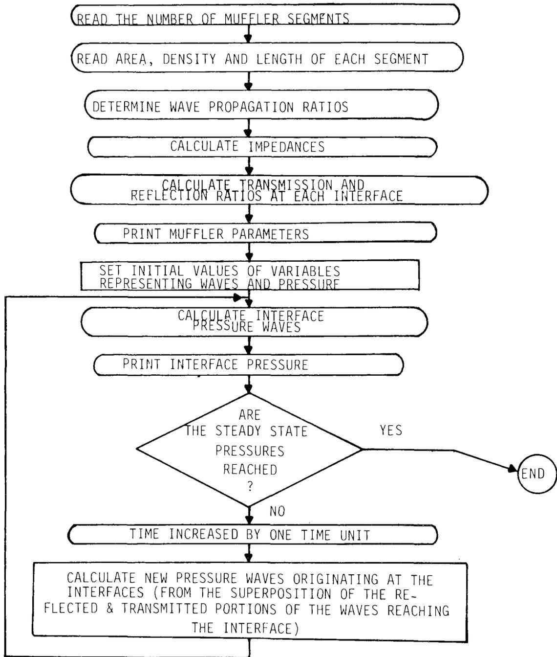
Fig. 2 Block diagram of analysis program
