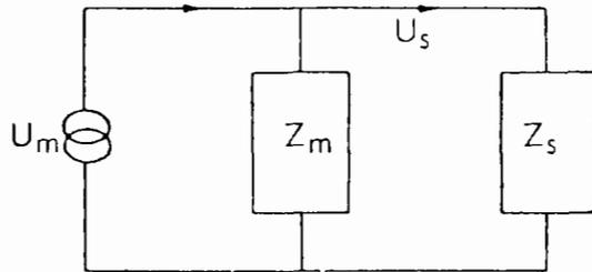
Figure 12 Acoustic model of engine and exhaust system
