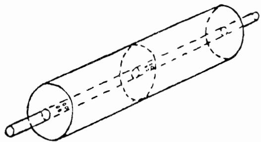
Figure 1d. Double Chamber Resonator
