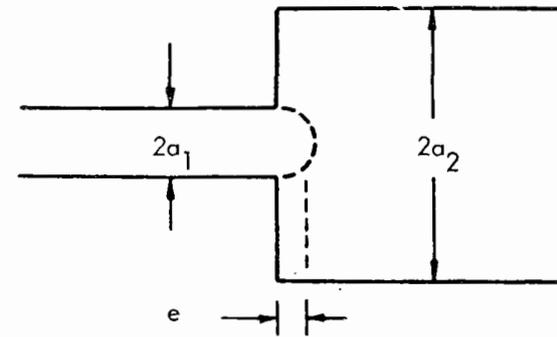
FIG. 3. END CORRECTION FOR EXPANSION OR CONTRACTION.
