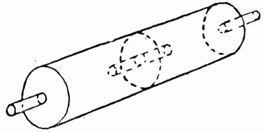
Figure 1b. Double Expansion Chamber With Internal Connecting Tubes
