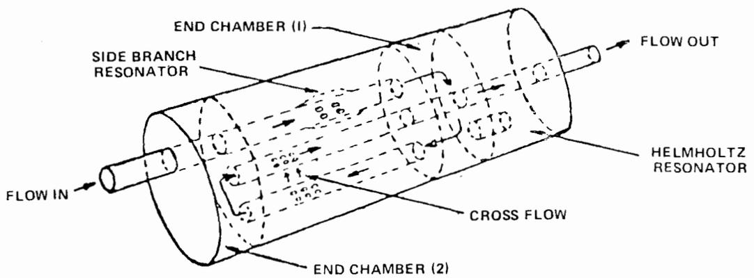
Figure 2. Typical Reverse – Flow Automobile Muffler
