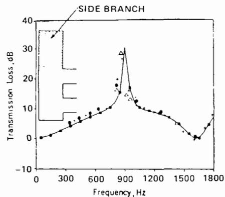
Figure 21. Transmission Loss for SI-CO Flow-Reversing Chamber ( $L = 2.0$  in.,  $H = 9.0$  in.,  $W = 4.75$  in.). Open Square—Predicted by Theory. Plus—Measured Without Flow; Open Triangle—Measured Without Flow (End Plate Vibration Eliminated); Circle—Measured With Flow at 110 ft/sec.
