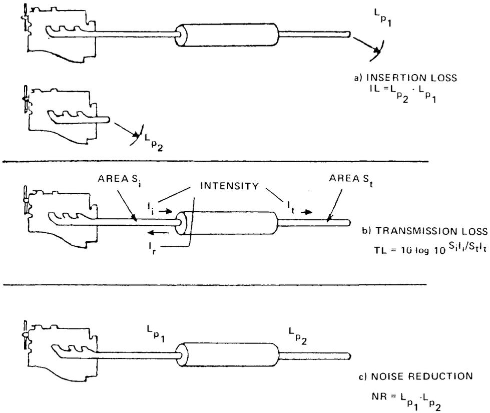
Figure 4. Definitions of Muffler Performance
