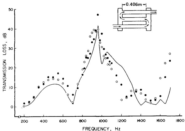
Figure 26. Transmission loss characteristics for combination of SI-CO and CI-SO flow reversing chambers; — is predicted; o is measured without flow and • is measured with a flow speed of 32 m/s
