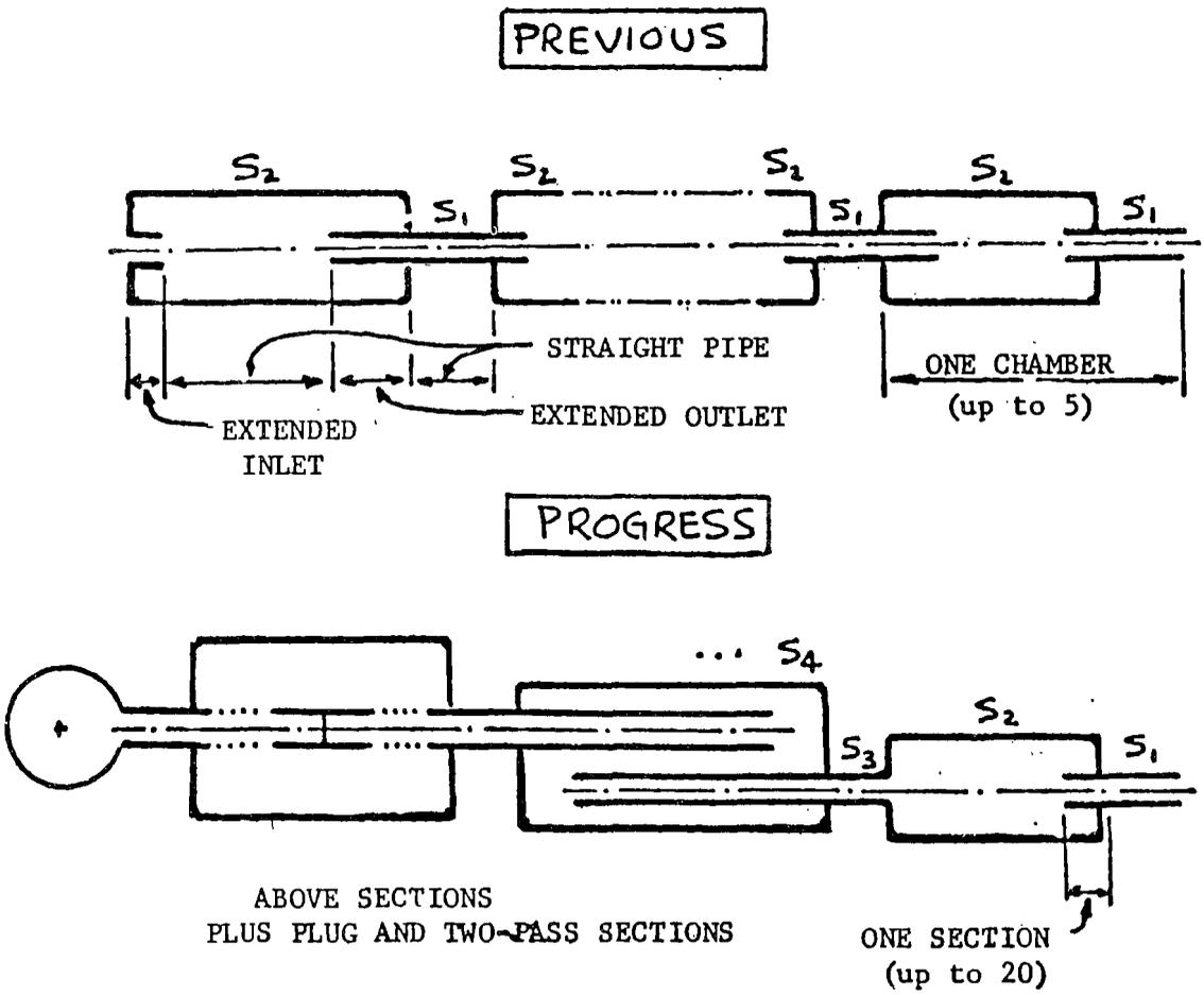
Figure 7. EXTENSIONS TO NASA MUFFLER DESIGN COMPUTER PROGRAM.
