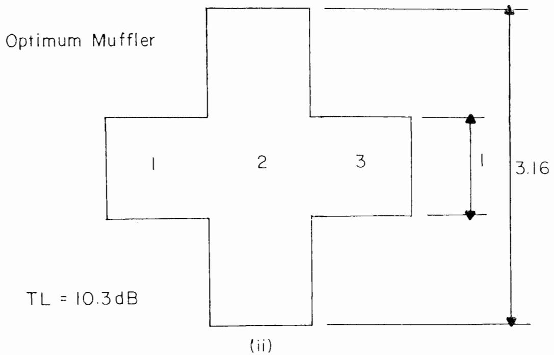
FIG.(4) Three Segment Reactive Muffler
