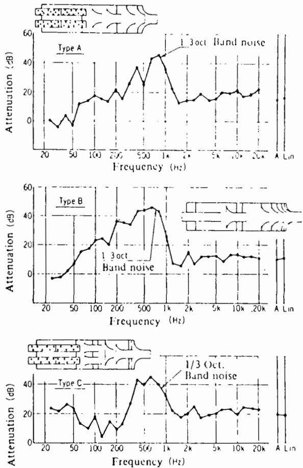
FIG-9 Acoustic attenuation of various test mufflers
