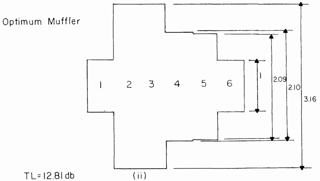
FIG (5-b) Six Segment Reactive Muffler
