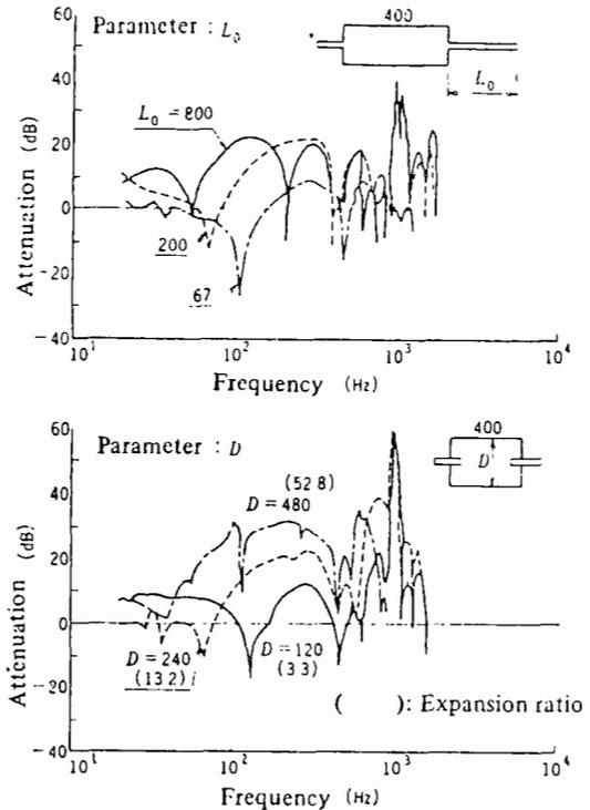
Fig. 3 Attenuation of muffler expansion chamber type
