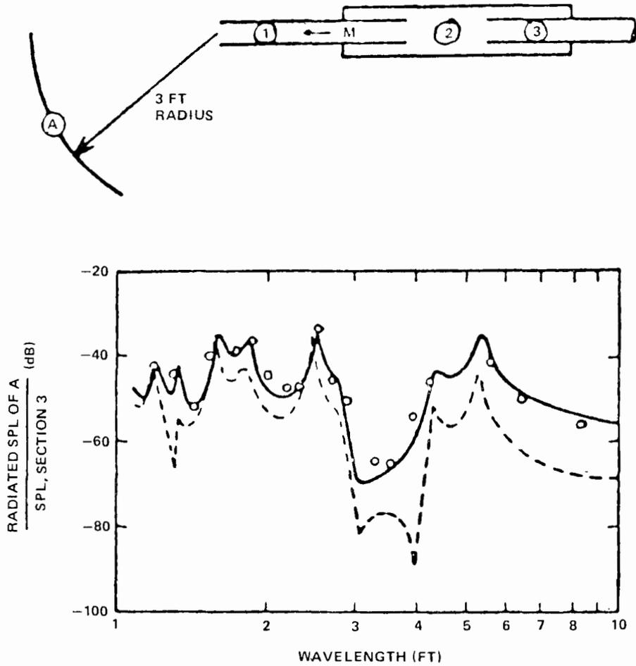
Figure 6. Influence of Mean Gas Flow on Effectiveness of Silencer. o, Measured values: — Calculated,  $M = 0.15$ ; ---, Calculated,  $M = 0.0$ .
