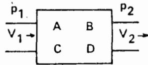
Figure 11. Four Pole Representation of Muffler Element
