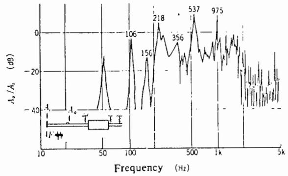
Fig. 16 Vibration response of exhaust system (Random excitation)
