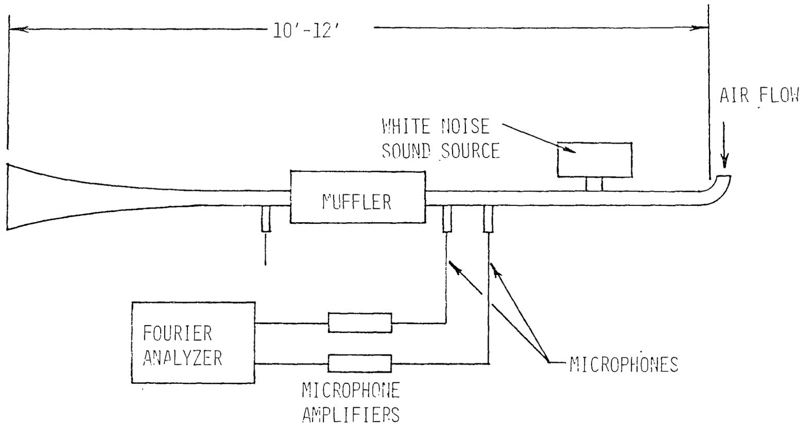
Figure 5. Measurement of muffler characteristics.
