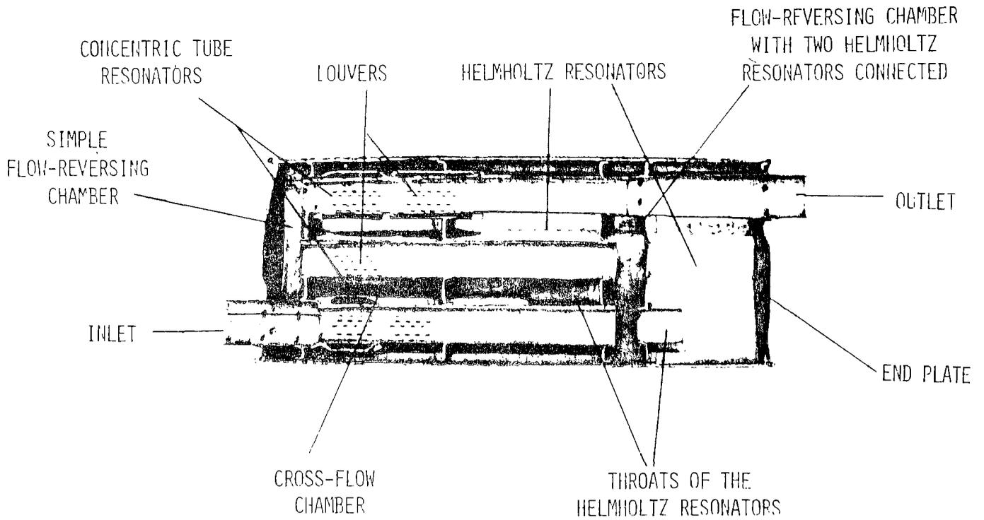
Figure 3 - Photograph showing cross section of common US reverse - flow automobile muffler with different parts indicated
