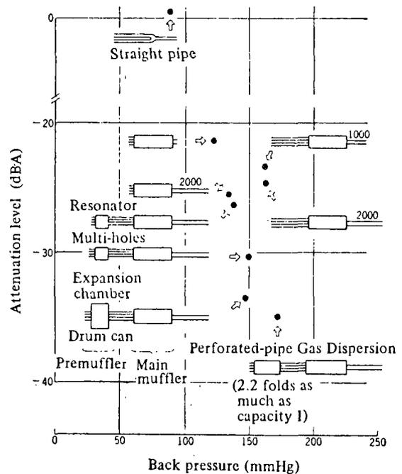
Fig. 22 Relation of exhaust noise reduction and back pressure of various exhaust system arrangements
