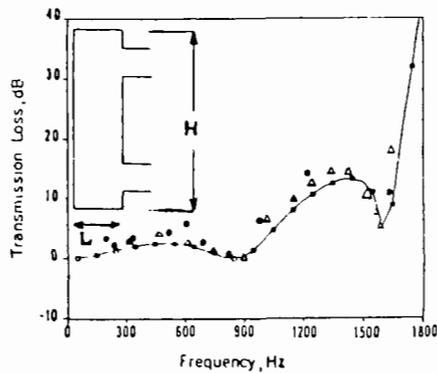
Figure 20. Transmission Loss for SI-SO Flow-Reversing Chamber ( $L = 2.0$  in.,  $H = 9.0$  in.,  $W = 4.75$  in.). Open Square—Predicted by Theory for No Flow Condition. Open Triangle—Measured Without Flow. Circle—Measured With Flow at 110 ft/sec.
