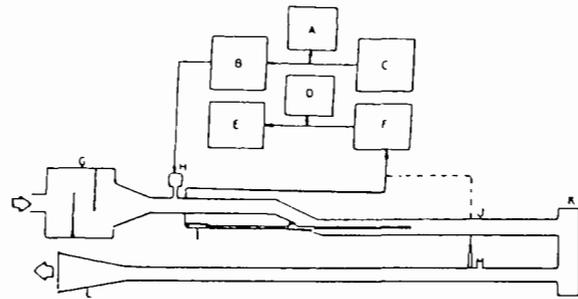
Figure 19. Experimental System for Measuring the Transmission Loss. A — Frequency Counter; B — Amplifier; C — Frequency Oscillator; D — Oscilloscope; E — Level Recorder; F — Spectrometer; G — Plenum Chamber; H — Acoustic Driver; I — Microphone Probe; J — Standing Wave Tube; K — Flow-Reversing Chamber; L — Anechoic Termination; and M — Microphone Port.
