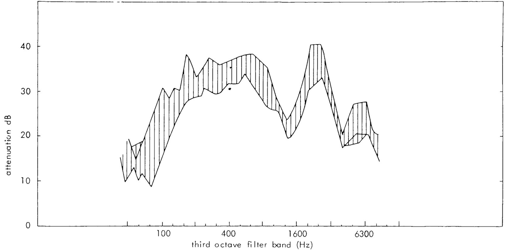
FIG. 16 AVERAGE MEASURED INSERTION LOSS, FULL LOAD TORQUE 8 SPEEDS,  $1000 < N < 2350$  rpm . Hatching indicates range of variation.
