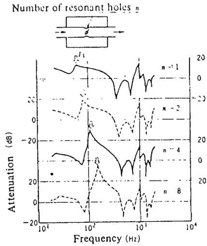
Fig. 4 Effect of number of resonant holes
