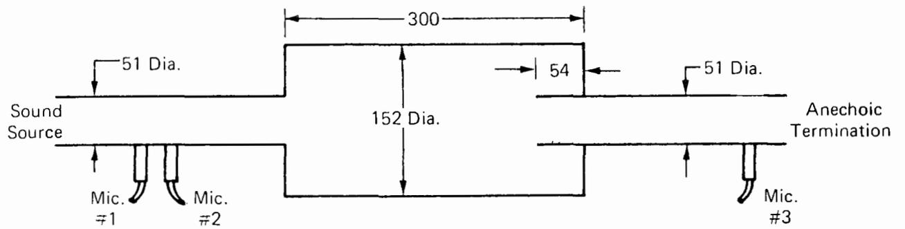
Figure 11. Expansion Chamber Silencer (dimensions in mm).
