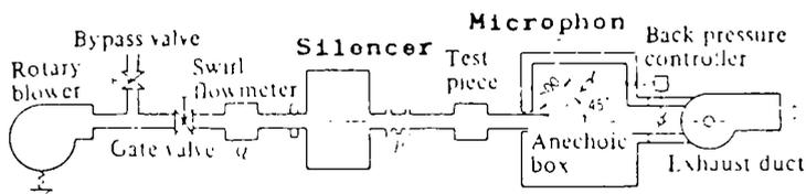
FIG-13 Experimental layout for flow generated noise
