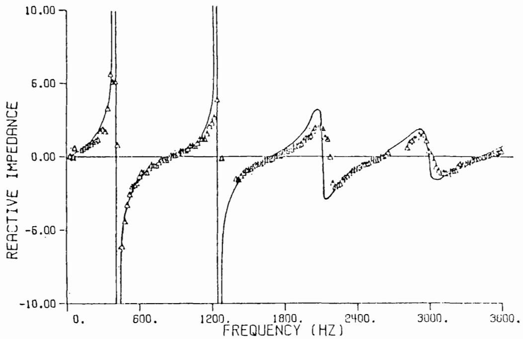
Figure 6. Resistive and reactive tail pipe impedances; solid line=theory; symbols=experiment.
