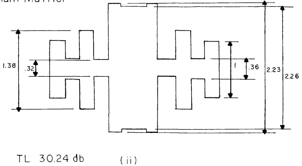
FIG.(6-a) Twelve Segment Reactive Muffler
