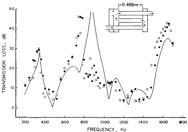
Figure 27. Transmission loss characteristics for combination of CI-SO and SI-SO flow reversing chambers with two resonators; — is predicted; o measured without flow; and • is measured with a flow speed of 32 m/s
