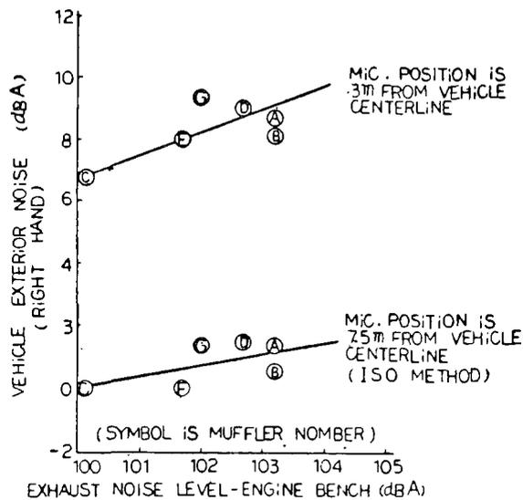
FIG-30. INFLUENCE OF EXHAUST NOISE TO VEHICLE EXTERIOR NOISE
