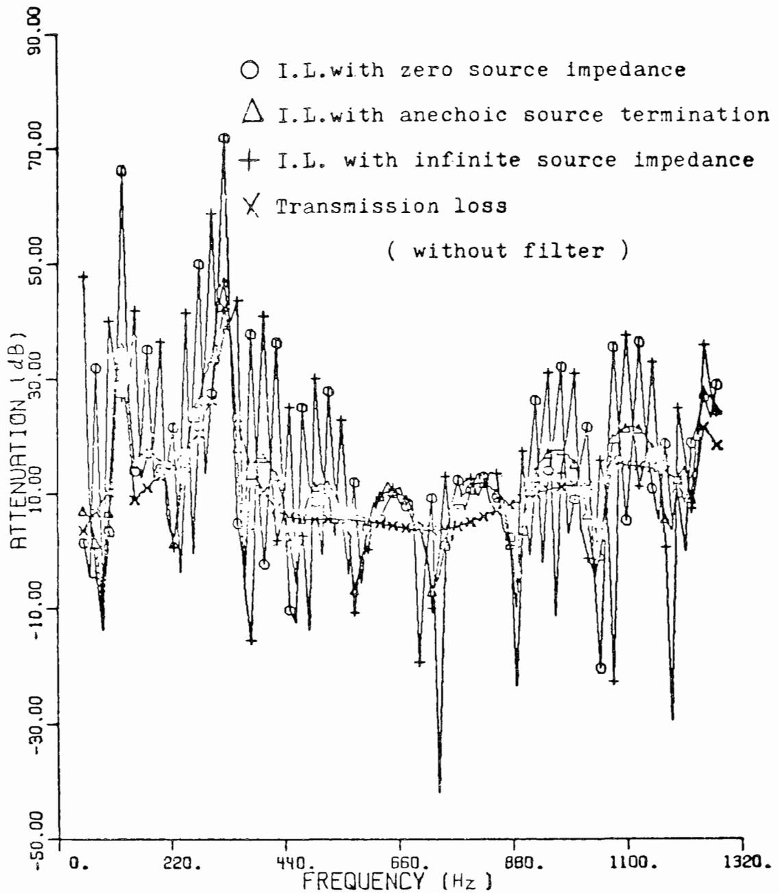
Figure 31. Theoretical Insertion Losses and Transmission Loss for Engine Exhaust Muffler System with Actual Exhaust Temperature Profile at Firing Frequency 100 Hz
