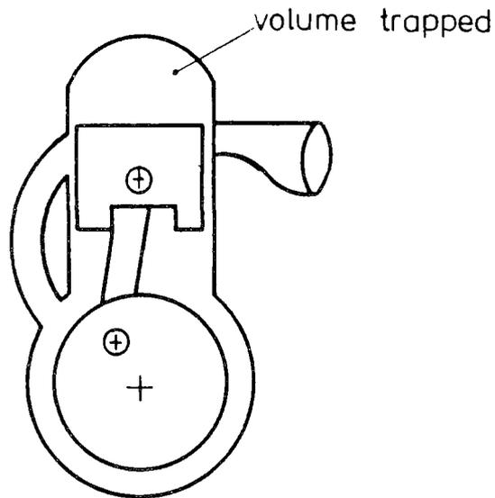
Fig.1 Crankshaft position shown at exhaust closing position, the trapping position, usually EXHSOPEN deg BTDC.
