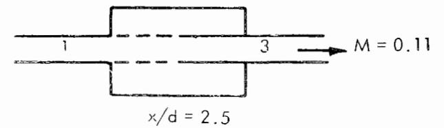
FIG. 10. SUPPRESSION OF FLOW-ACOUSTIC COUPLING BY A BRIDGE PERFORATE.
