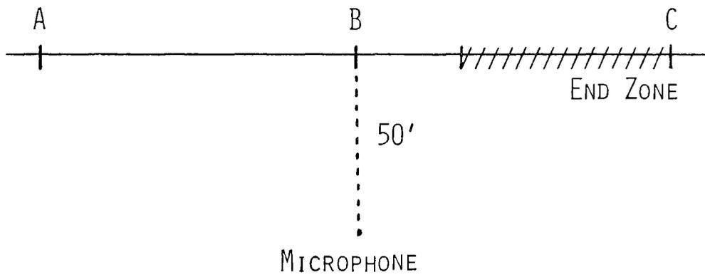
Fig. 2 Schematic Diagram of Drive-By Test Per SAE-366b
