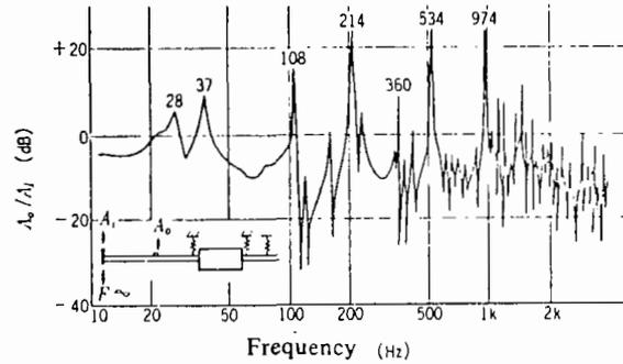
Fig. 17 Vibration response of exhaust system (Sinusoidal excitation)
