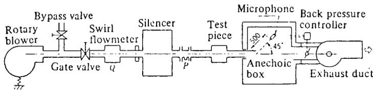
Fig. 6 Experimental layout for flow generated noise
