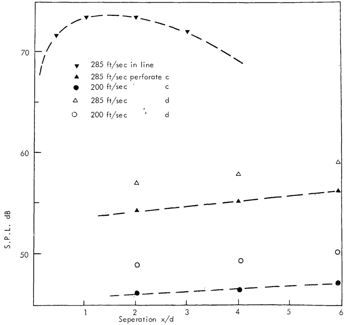
FIG. 7. FLOW NOISE REDUCTION BY PERFORATES.
