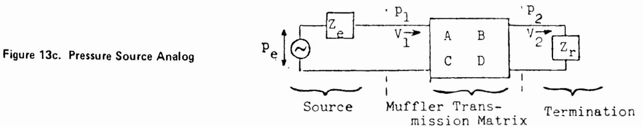
Figure 13c. Pressure Source Analog
