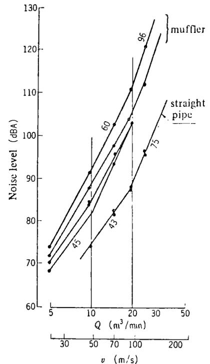
Fig. 7 Flow generated noise level under various mufflers
