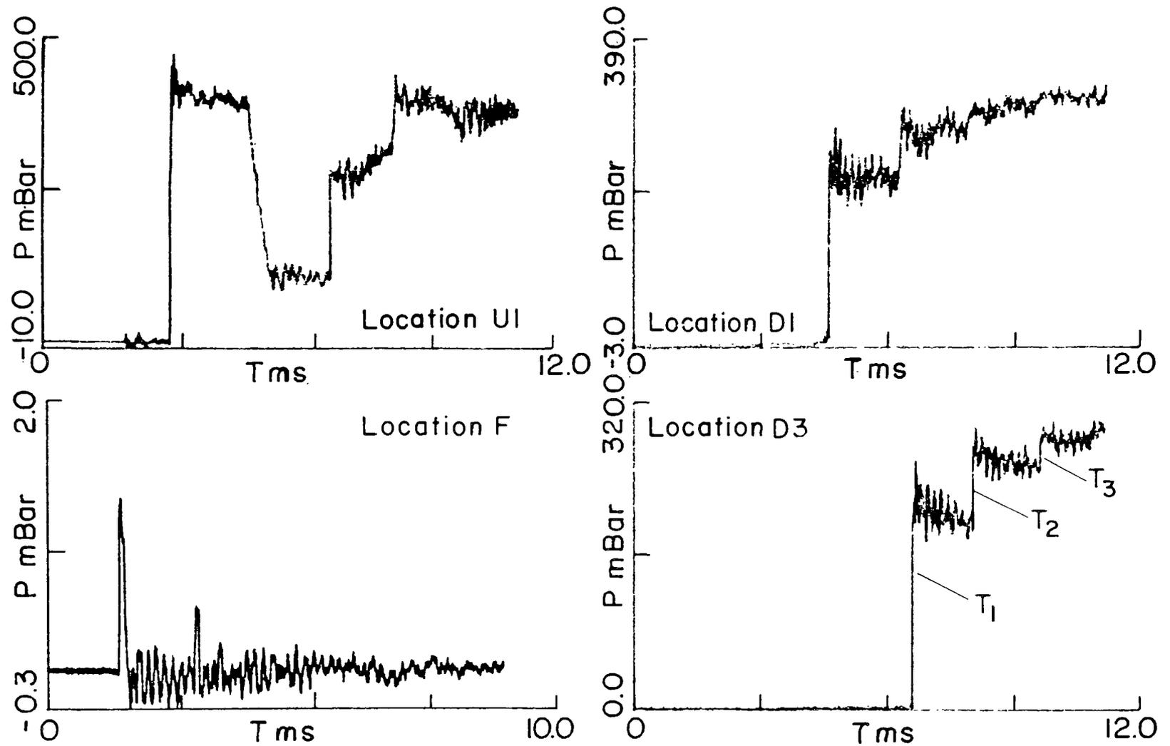
FIGURE 12 PRESSURE HISTORIES OF SHOCK PROPAGATION THROUGH EXPANSION CHAMBER, B.  $M_s = 1.17$ , SHOCK TUBE
