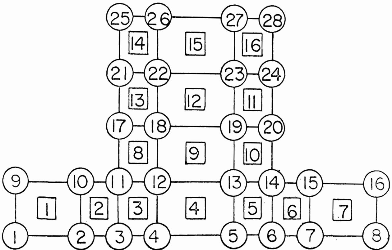
Figure 16. Simple Expansion Chamber Showing Division Into 16 Finite Elements and 28 Node Points
