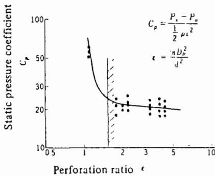
Fig. 14 Static pressure coefficient vs. perforation ratio
