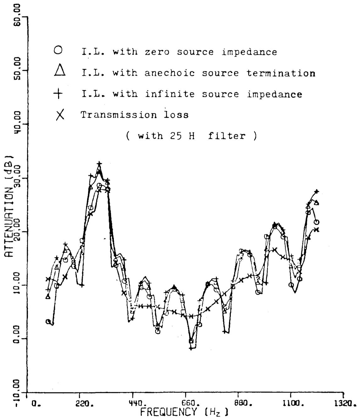
Figure 32. Theoretical Insertion Losses and Transmission Loss for Engine Exhaust Muffler System at Elevated Temperature at Firing Frequency 70 Hz
