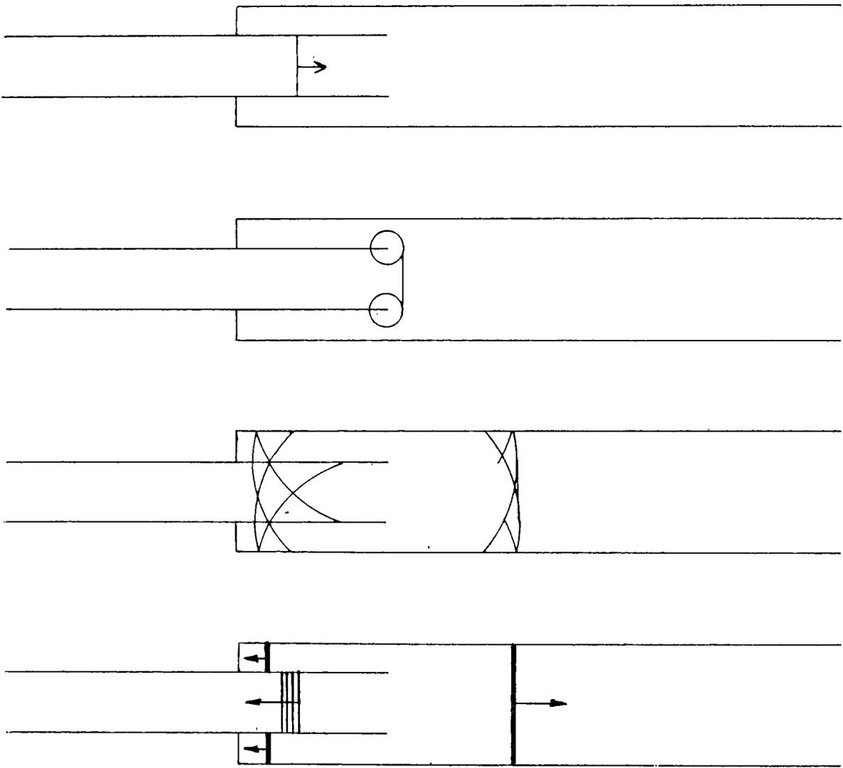
FIG. II SHOCK INTERACTION WITH AN EXTENDED INLET
