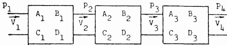
Figure 12. Series Connection of Transmission Matrices
