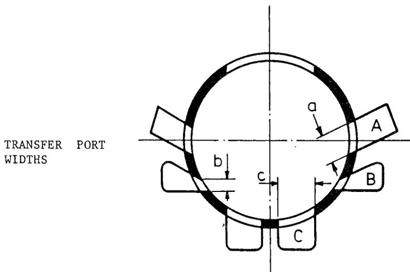
Fig.6 Plan Section through transfer ports
