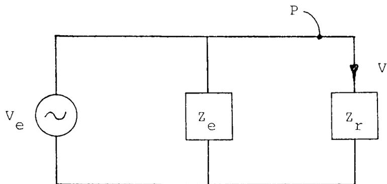
Figure 4. Model for engine and exhaust manifold without exhaust system.
