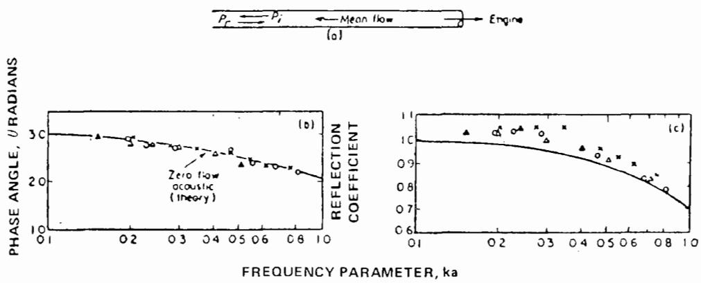
Figure 14. Reflection of Sound. (a) Exhaust Tail Pipe,  $P_r = R \cdot P_i e^{i\theta}$ . (b) Phase Angles vs. Frequency Parameter. (c) Reflection Coefficient Vs. Reflection Parameter. —, Theoretical Zero Flow Acoustic; o,  $M = 0.078$ ;  $\Delta$ ,  $M = 0.11$ ; x,  $M = 0.17$ .
