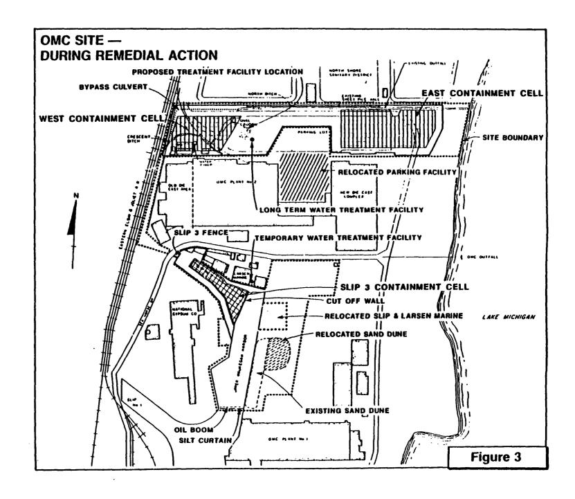
sediments will be placed in the West Containment Cell. Extracted PCBs will be disposed of off-site in accordance with all applicable Federal and State laws. The average PCB concentration in the West containment cell will be 90 ppm.
