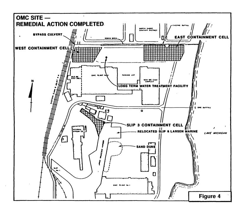
On-site containment cells will have significantly lower average PCB concentrations than the cells envisioned in the 1984 ROD. These Toxic Substances Control Act (TSCA) compliant cells have been designed with strict engineering standards and will be managed by the OMC trustee with oversight by U.S. EPA and IEPA. Every 5 years, the integrity of the cells will be assessed.
