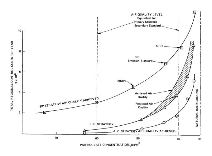
standard geometric deviation, the Federal standards become 85 and 65  $\mu g/m^3$  annual arithmetic average (primary and secondary, respectively).\* The 60 and 40  $\mu g/m^3$  concentrations in Figure 3 correspond roughly to these primary and secondary ambient particulate standards when the 25  $\mu g/m^3$  increment for omitted sources is added.
