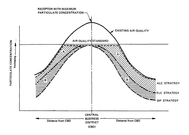
Area A shows the air quality improvement gained in going from ALC to ELC and Area B shows that gained in going from ELC to SIP. As shown above, each of these jumps (from ALC to ELC, and from ELC to SIP) may increase costs by a factor of 2 or more.
