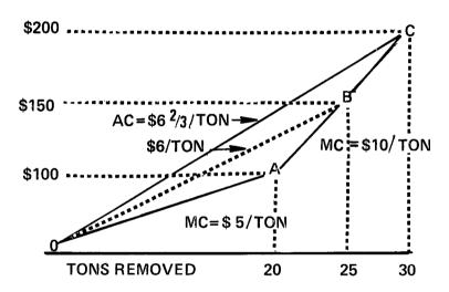
removed at a total cost of \$100. The control method employed and its removal efficiency are represented by point A. Removal efficiency of this device (operated at full power) is calculated as the ratio of tons removed to uncontrolled tons emitted by the source times 100. Point C has a similar interpretation.
