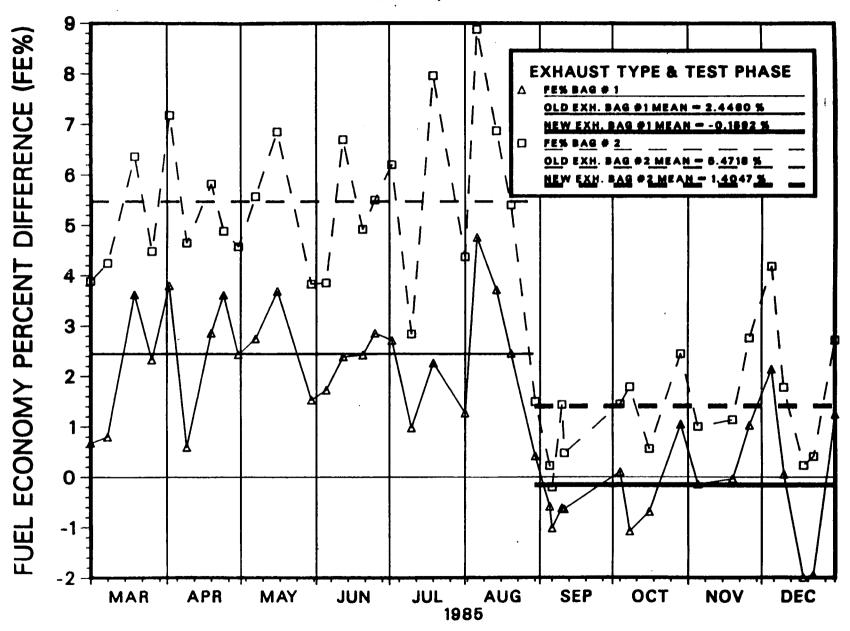
FE%=[(CARB. BAL. FE - METERED FE)/(METERED FE)]\*100 CVS 24C, DYNO D004
