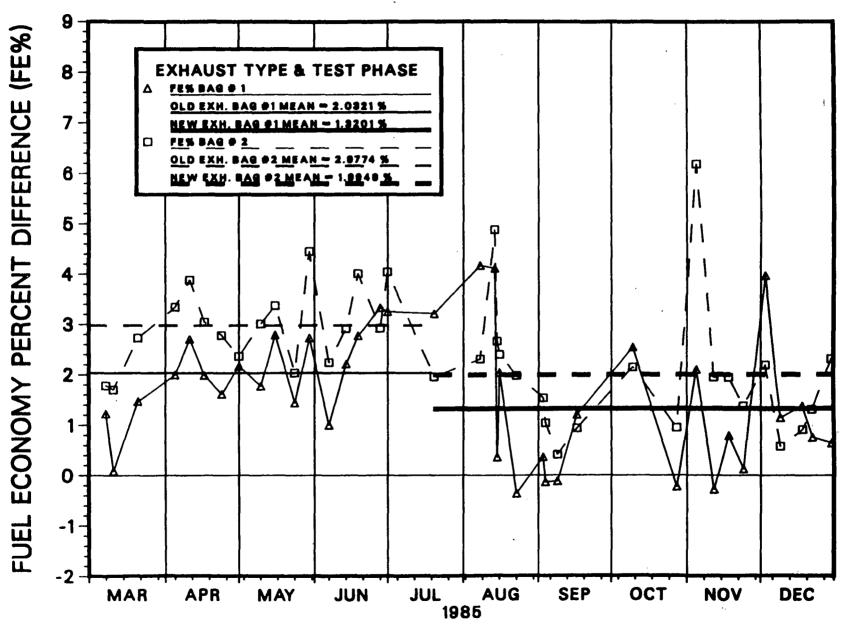
FE%=[(CARB. BAL. FE - METERED FE)/(METERED FE)]\*100 CVS 22C, DYNO D002
