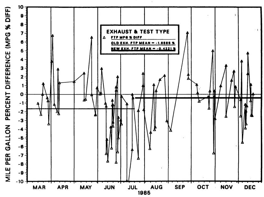
MPG % DIFF=[(MFR MPG - EPA MPG)/(EPA MPG)]\*100 CVS 21C, DYNO D001
