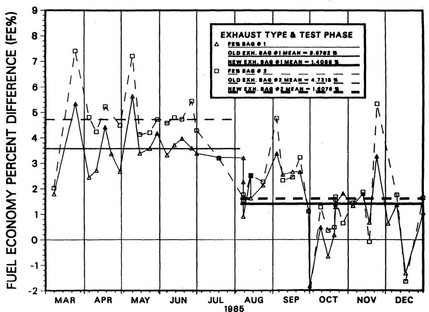
FE%=[(CARB. BAL. FE - METERED FE)/(METERED FE)]\*100 CVS 23C, DYNO D003
