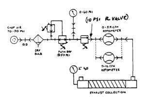
The leak check procedure will consist of pressurizing the assembly with a shop air source which has a rotometer in line. Pressurize the exhaust collection hose to  $2^n\mathrm{H}_2\mathrm{O}$  positive pressure (negative pressure leakage will only be additional dilution air). The approximate flow (measured by a rotometer) needed to maintain  $2^n\mathrm{H}_2\mathrm{O}$  will then be defined as system leakage.
