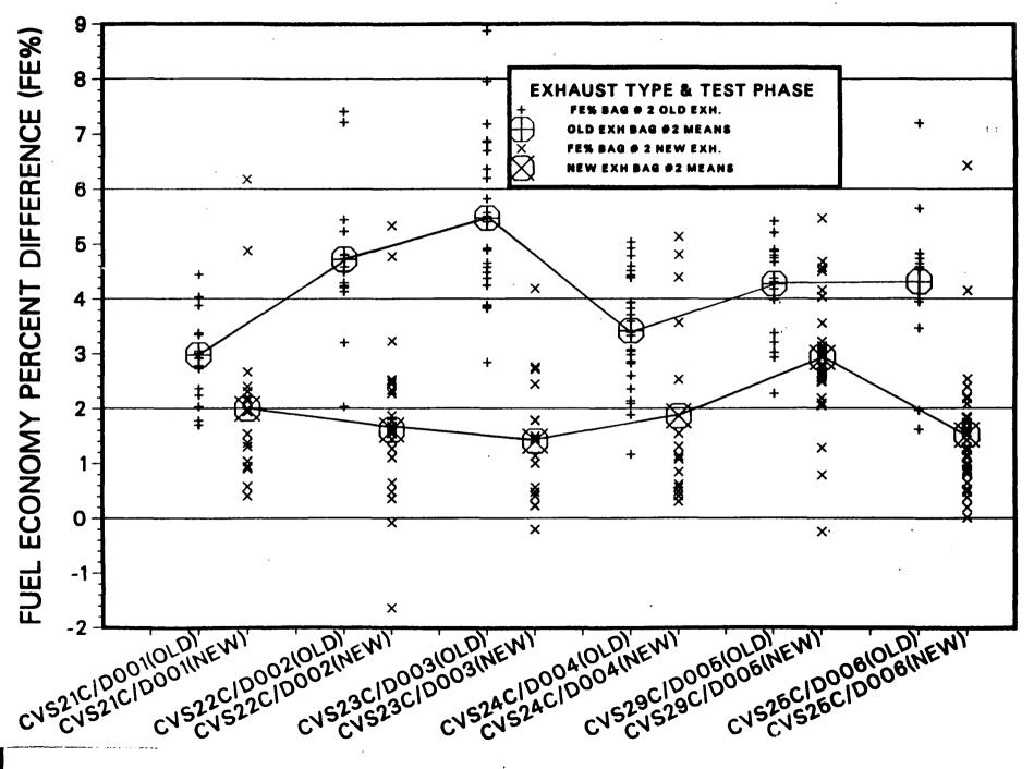
FE%=[(CARB. BAL. FE - METERED FE)/(METERED FE)]\*100 CVS 21C, DYNO D001
