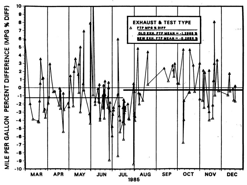
MPG % DIFF=[(MFR MPG - EPA MPG)/(EPA MPG)]\*100 CVS 29C, DYNO D005
