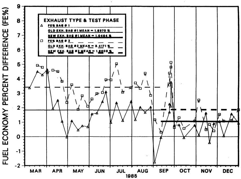
FE%=[(CARB. BAL. FE - METERED FE)/(METERED FE)]\*100 CVS 29C, DYNO D005
