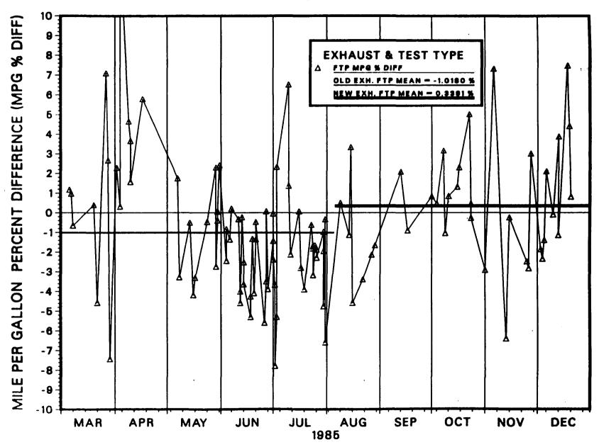
MPG % DIFF=[(MFR MPG - EPA MPG)/(EPA MPG)]\*100 CVS 22C, DYNO D002
