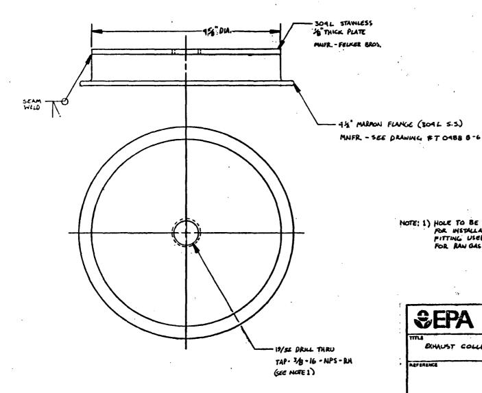
NOTE: 1) HOLE TO BE DRILLED & TAPRED FOR INSTALLATION OF THERMOLOUPLE FITTING USED AS ACCESS ROINT FOR RAW GAS SAMPLE PROBE.
