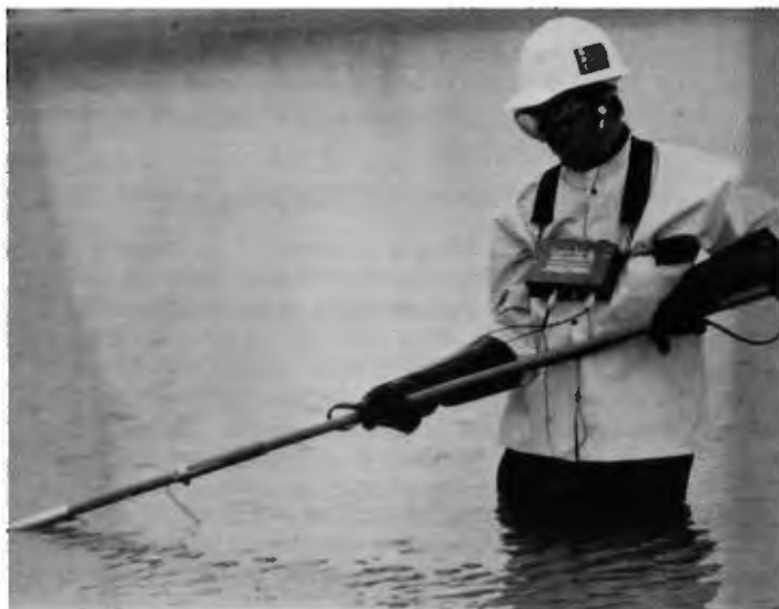
Figure 2 Manual Leak Location Equipment Consisting of an Electrode Probe and Electronics Unit
