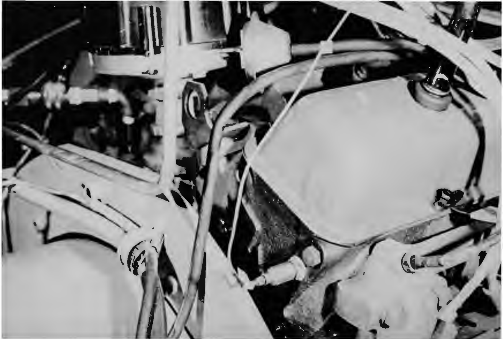
FIGURE 5-9 - Accelerometer Attached to Right Rear Cylinder Head of 350 CID Engine with Axis Parallel to Engine Crankshaft
