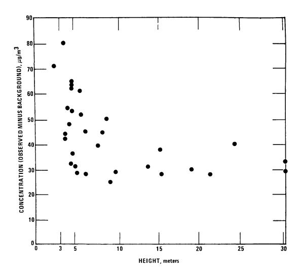
Figure 3.2 Decay of adjusted concentration versus height for sites with "high" local activity
