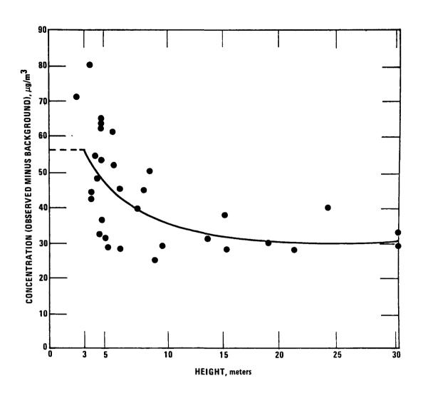
Figure 3.3 Plot of relationship between adjusted concentration and height of monitor
