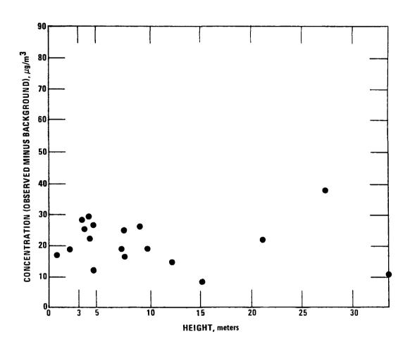
Figure 3.1 Constancy of adjusted concentration versus height for sites with "low" local activity
