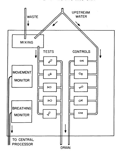
Figure 1. A monitoring unit for industrial use, showing how the test fish are exposed to waste diluted with upstream water and the control fish are exposed to upstream water alone.
