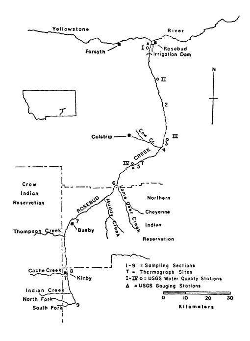
Figure 1. Map of Rosebud Creek showing sampling sections, gauging stations, and thermograph locations.
