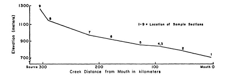
Figure 2. Longitudinal profile of Rosebud Creek.
