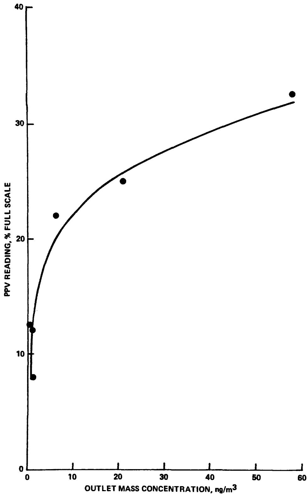
Figure 5. Relative PPV reading versus outlet mass concentration for ESP.
