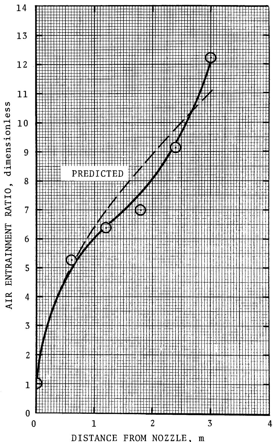
Figure 6. Measured and predicted entrainment ratio.
