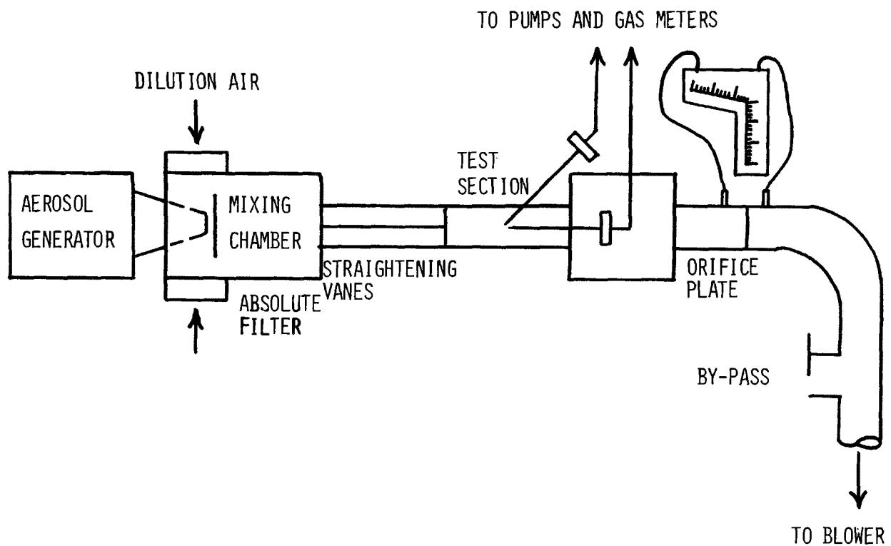
Figure 5. Experimental system to determine inertial sampling bias.
