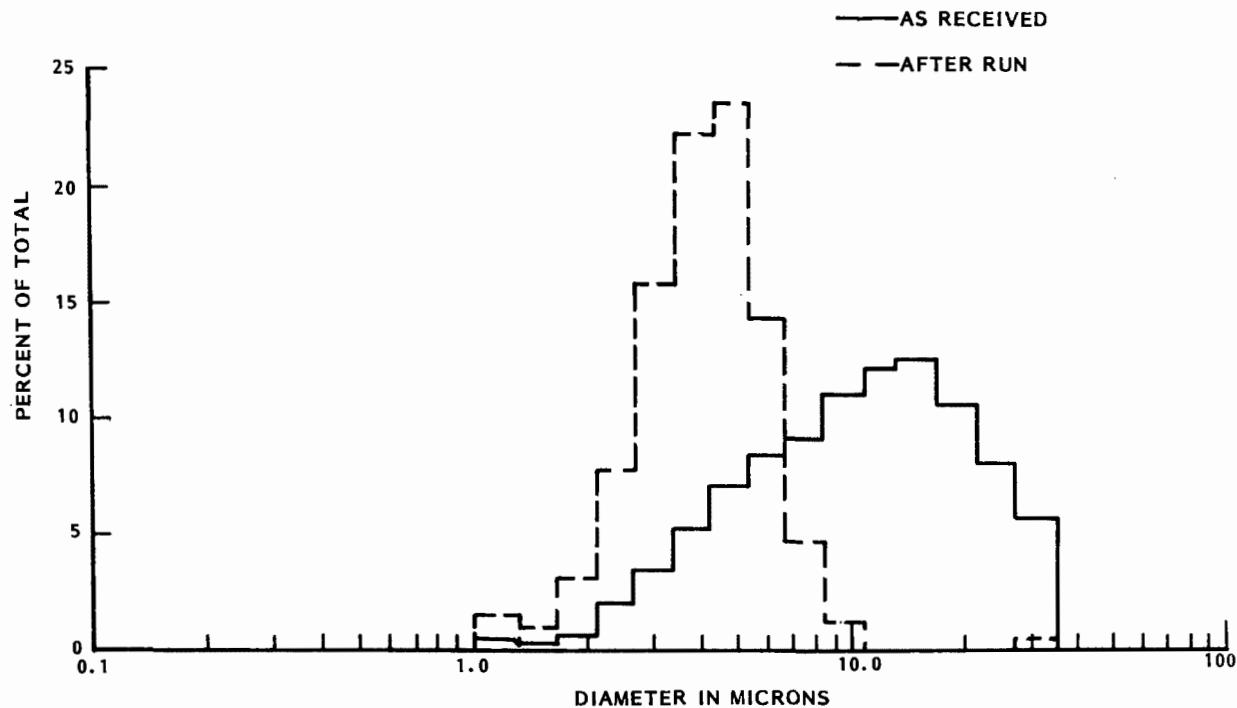
Figure 11. Coulter counter analysis of fly ash 1; — as received, - - after run using 100 micron orifice.
