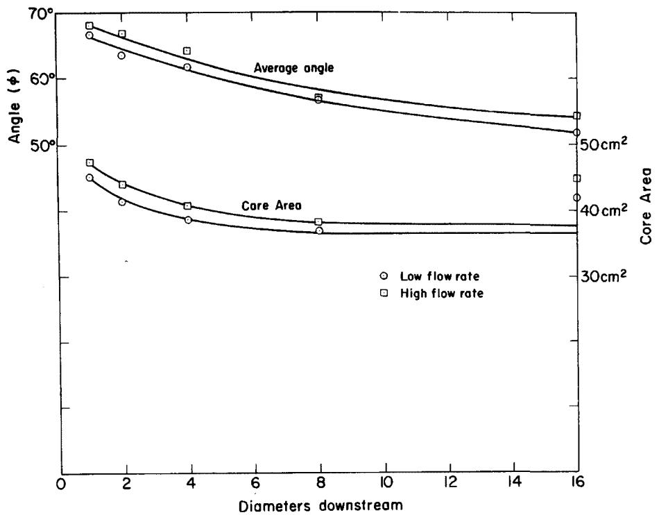
Figure 9. Decay of the angle  $\theta$  and core area along the axis of the duct.
