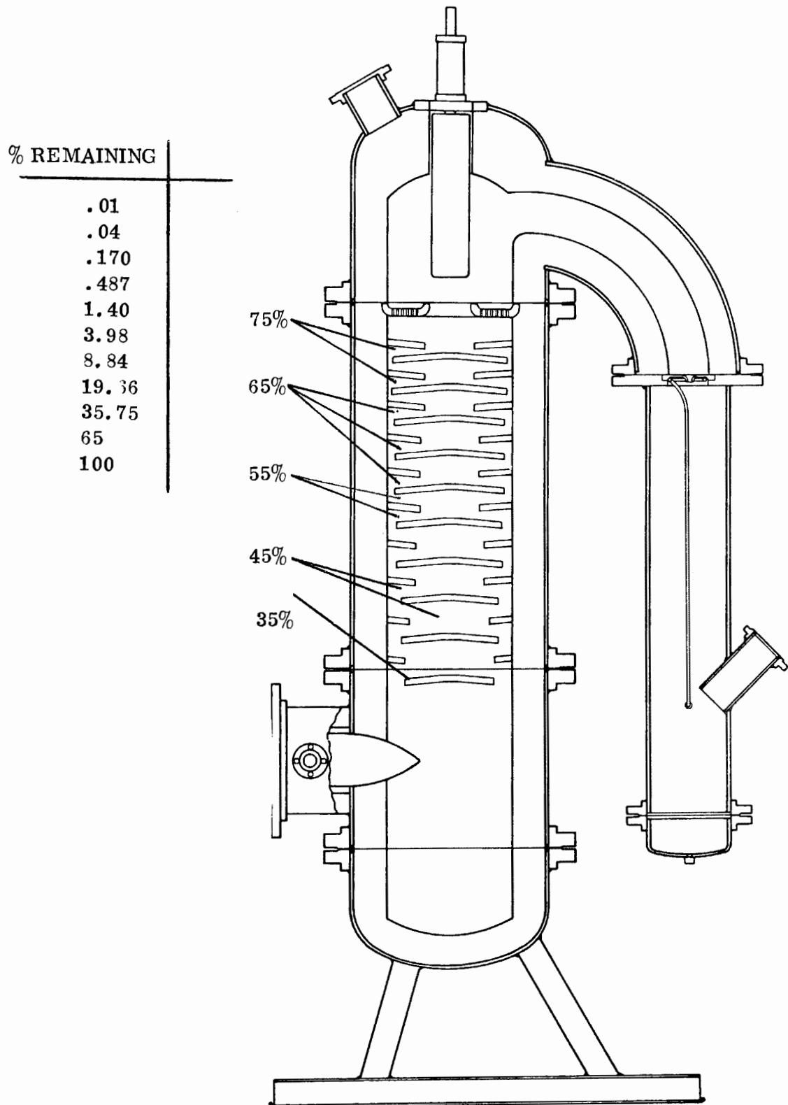
Figure 8. Schematic of present scrubber design showing calculated efficiency of each subunit and % fly ash remaining after passing each subunit.
