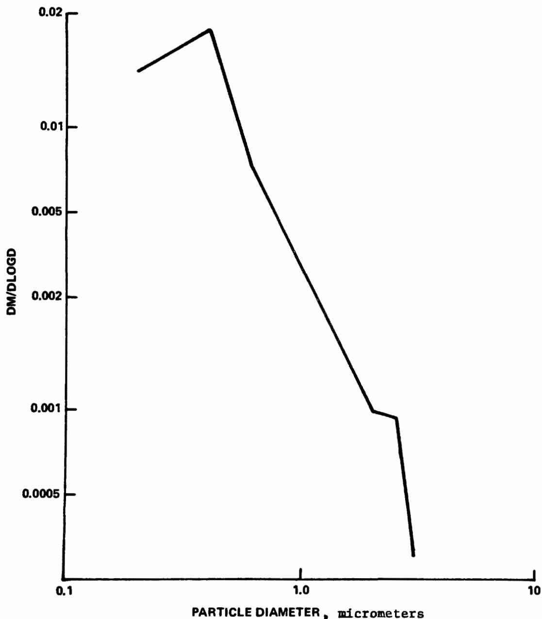
Figure 4. Scrubber outlet particle size distribution for ESP scrubber experiments.
