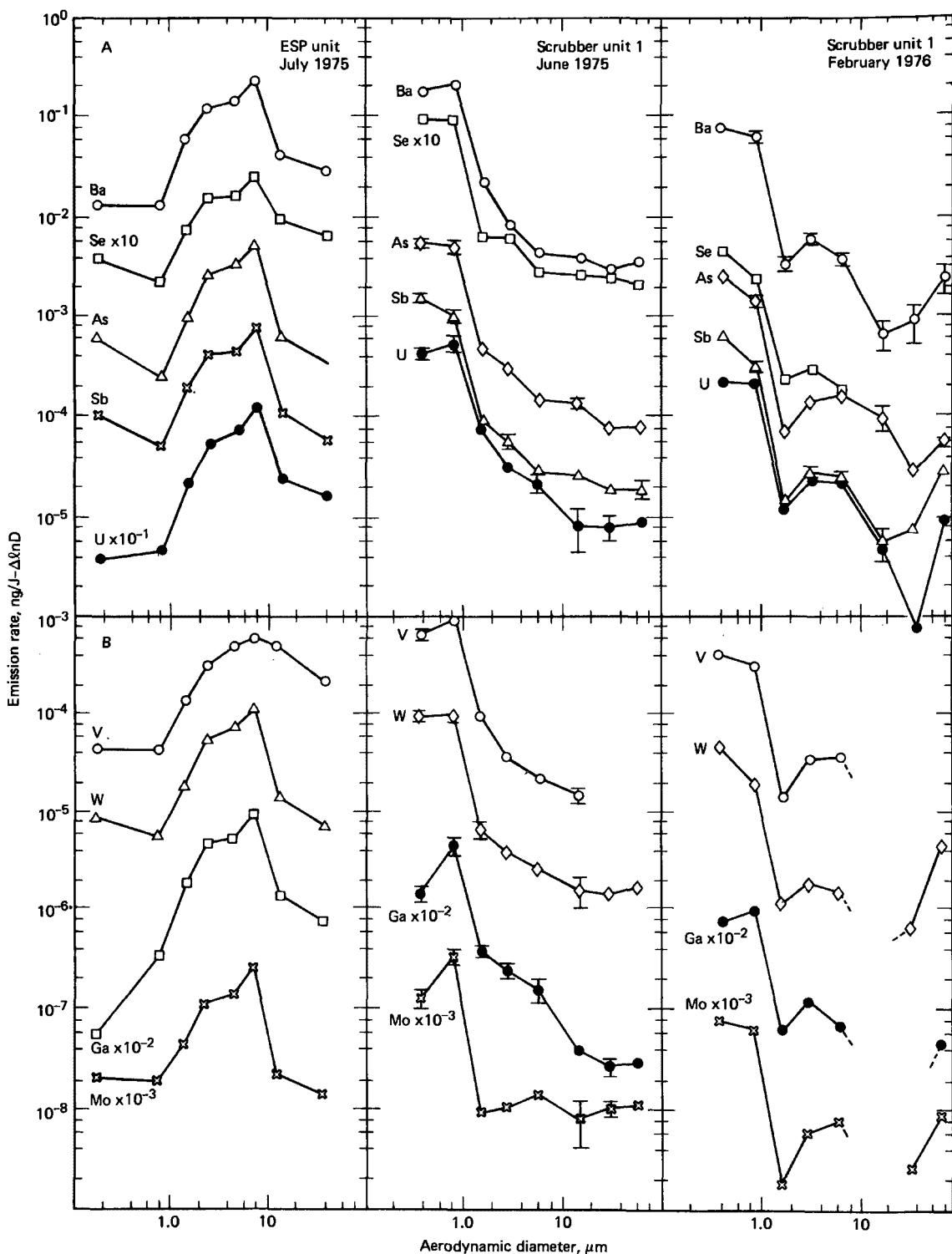
**Figure 5.** Particle-size distributions of elements emitted from power units equipped with a cold-side ESP and a venturi wet scrubber. The concentration data of individual elements are expressed as emission rate per joule of heat input to the boiler to allow comparison of the two units. The data are normalized to log size intervals (D=particle diameter).
