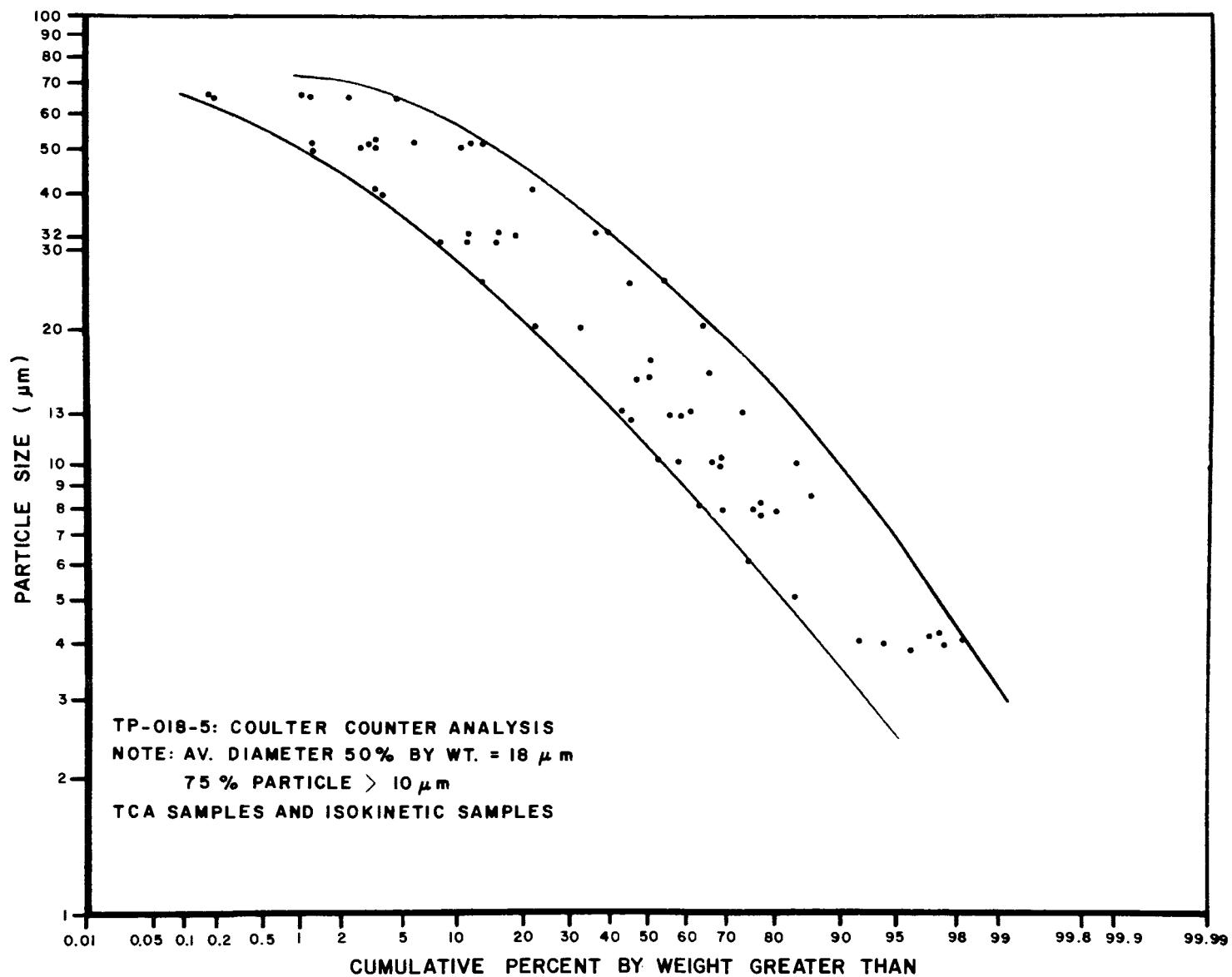
Figure 5. Cyclone Penetration Particulate Size Penetration Data (Coulter Counter Analysis) TP-018-5
