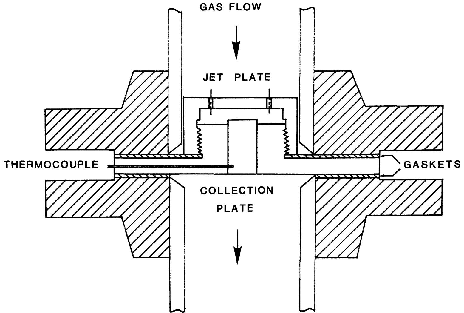
Figure 1. HTP single stage impactor.
