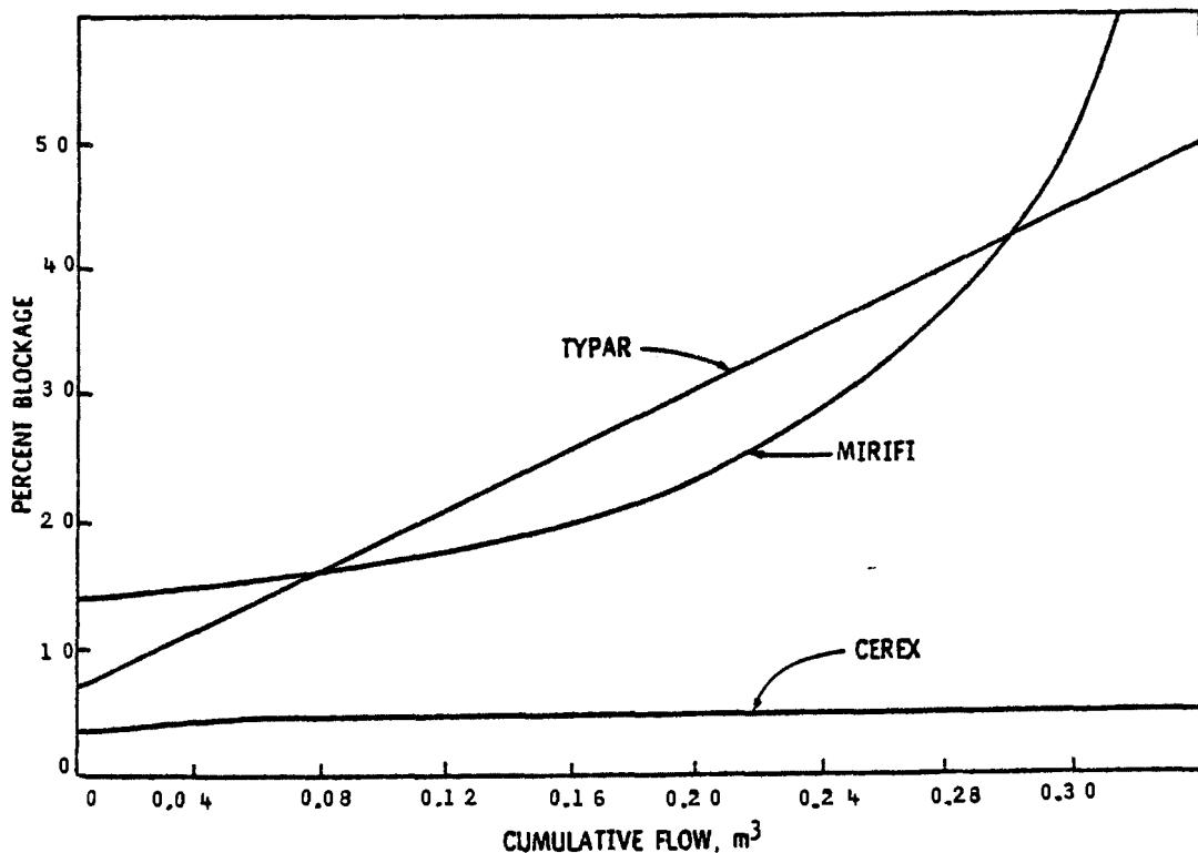
Figure 3. Blockage of fabric due to Hoytville clay in water.
