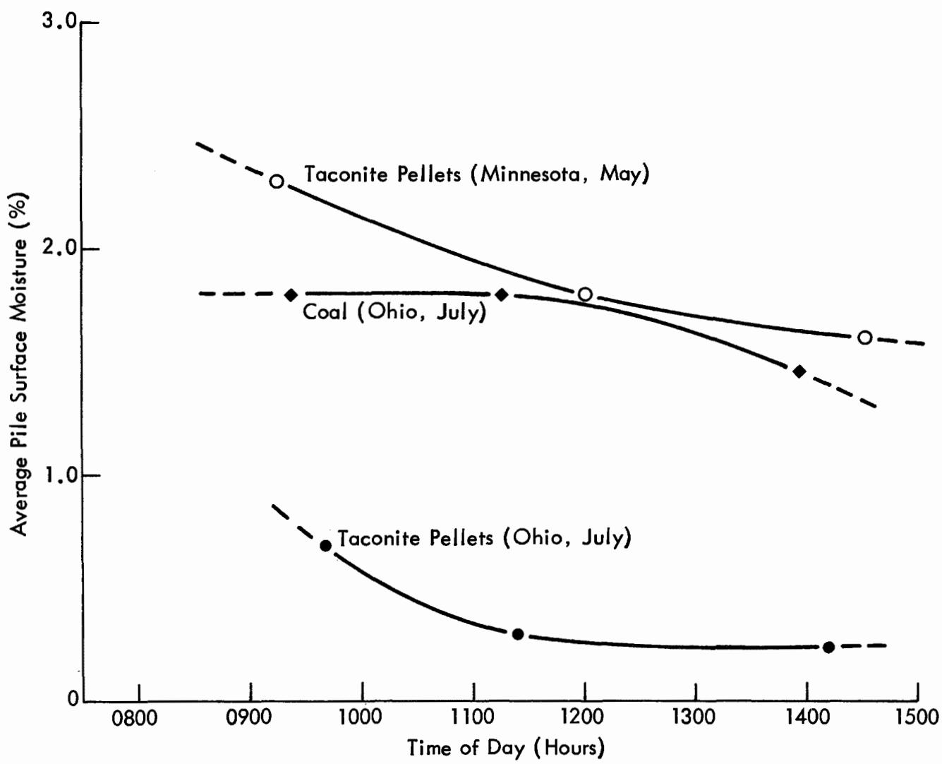
Figure 2. Observed storage pile surface moisture versus time of day.
