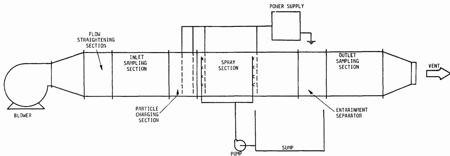
Figure 7. Experimental apparatus for studying charged spray section of SCAT scrubber.
