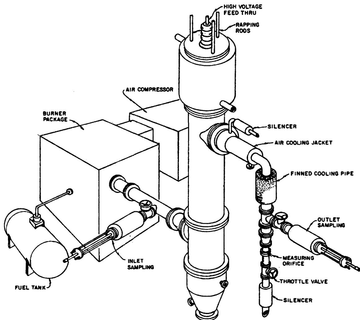
Figure 1. HTHP-ESP SYSTEM
