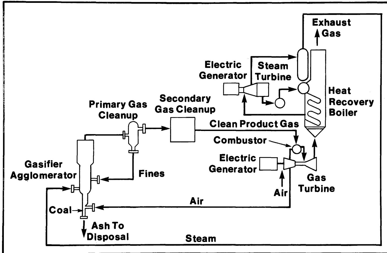
Figure 2. Westinghouse Single-Stage Coal Gasification Combined Cycle System
