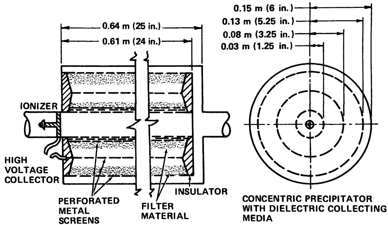
Figure 6. Second prototype electrostatic precipitator for collecting diesel particulate.
