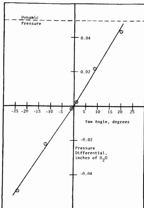
Figure 4. Five-hole pitot tube sensitivity to yaw angle.<sup>20</sup>
