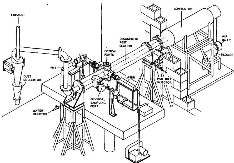
Figure 12. Sketch Of The Atmospheric Combustor Exhaust Simulator (ACES) Facility
