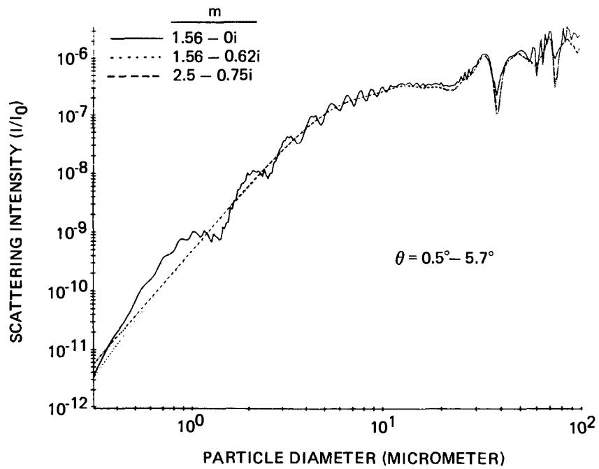
Figure 8. Calculated Mie Scattering Response Curve At Small-Angle Near-Forward Direction and  $\lambda = 0.647 \mu\text{m}$
