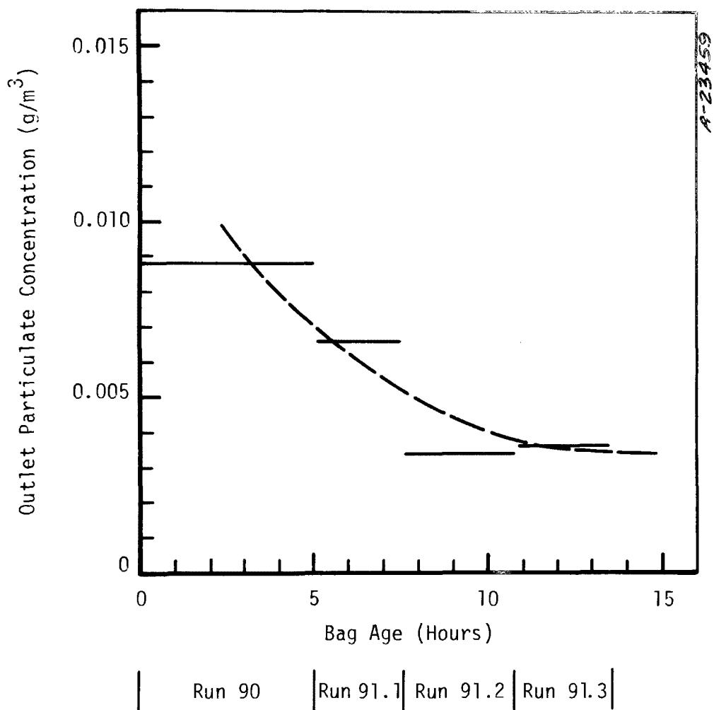
Figure 7. Acurex ceramic bag filter -- bag no. 5 particulate penetration history.
