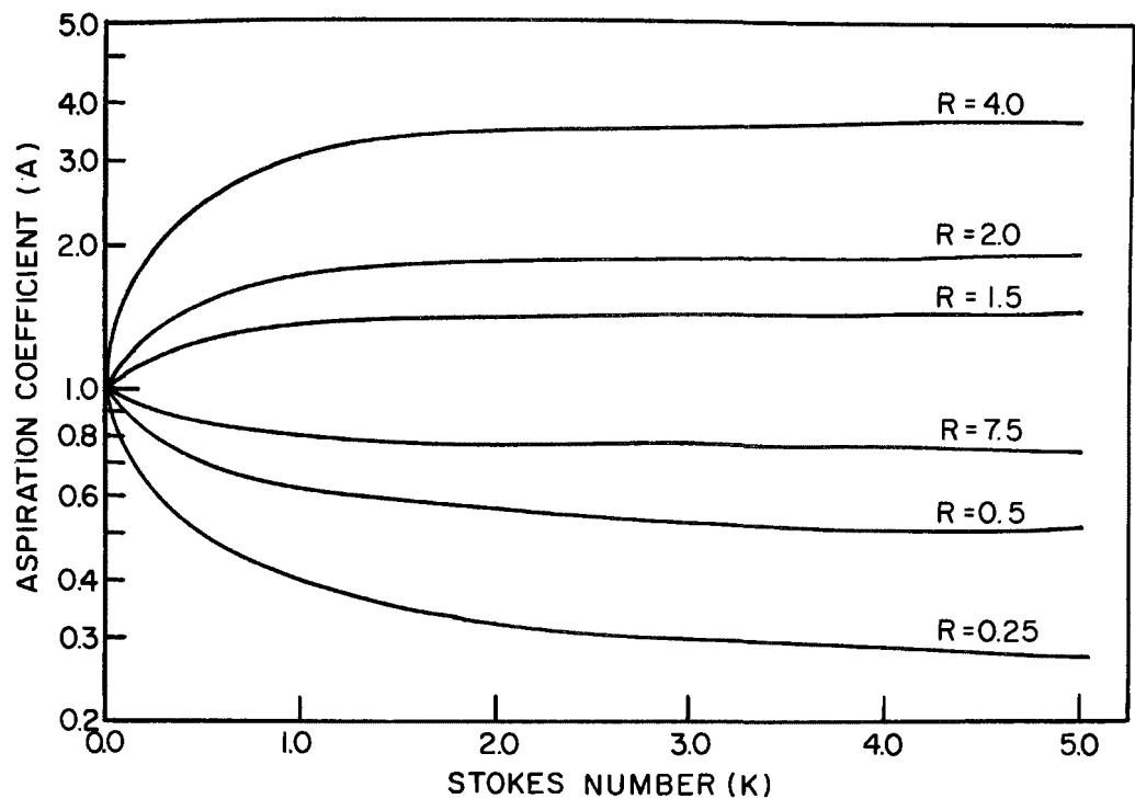
Figure 1. Sampling efficiency as a function of Stokes number (K) and velocity ratio ( $R = V_o/V_i$ ).<sup>8,9</sup>
