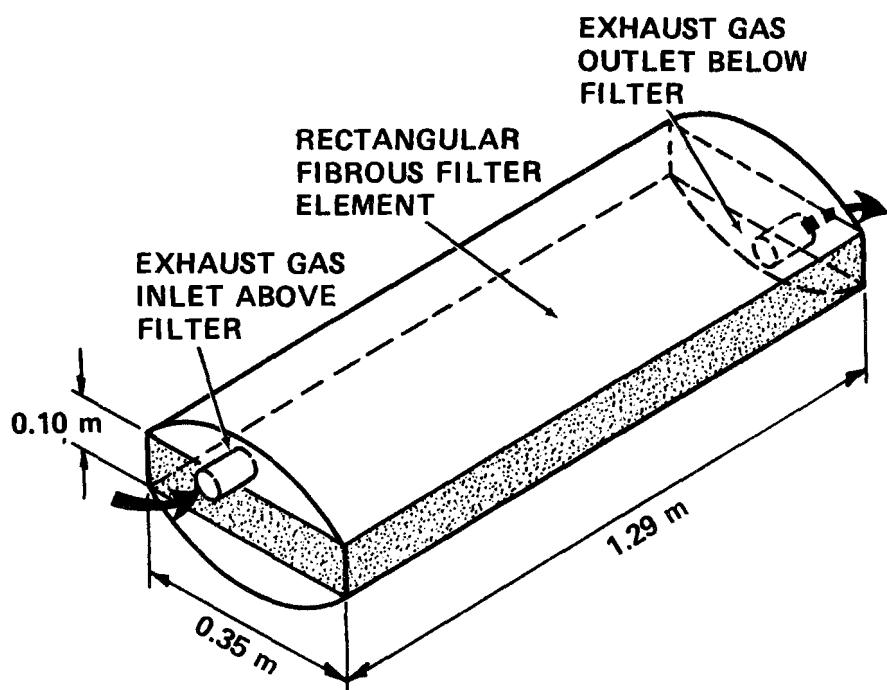
Figure 3. Prototype fibrous filter.
