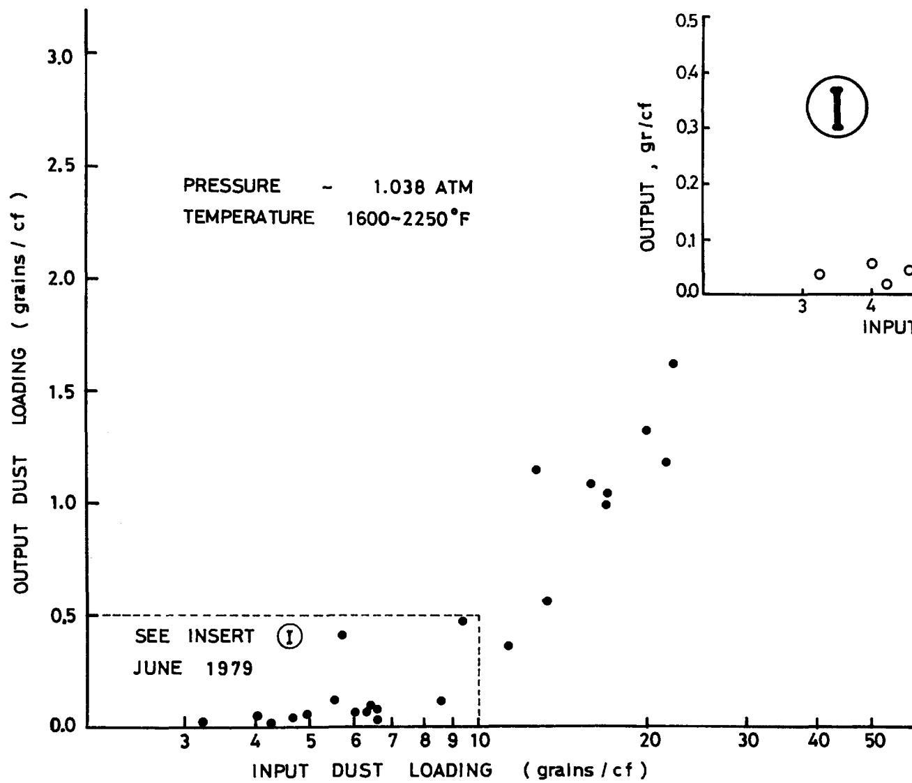
FIGURE 6 CYCLONE PERFORMANCE BASED ON OUTPUT DUST LOADING
