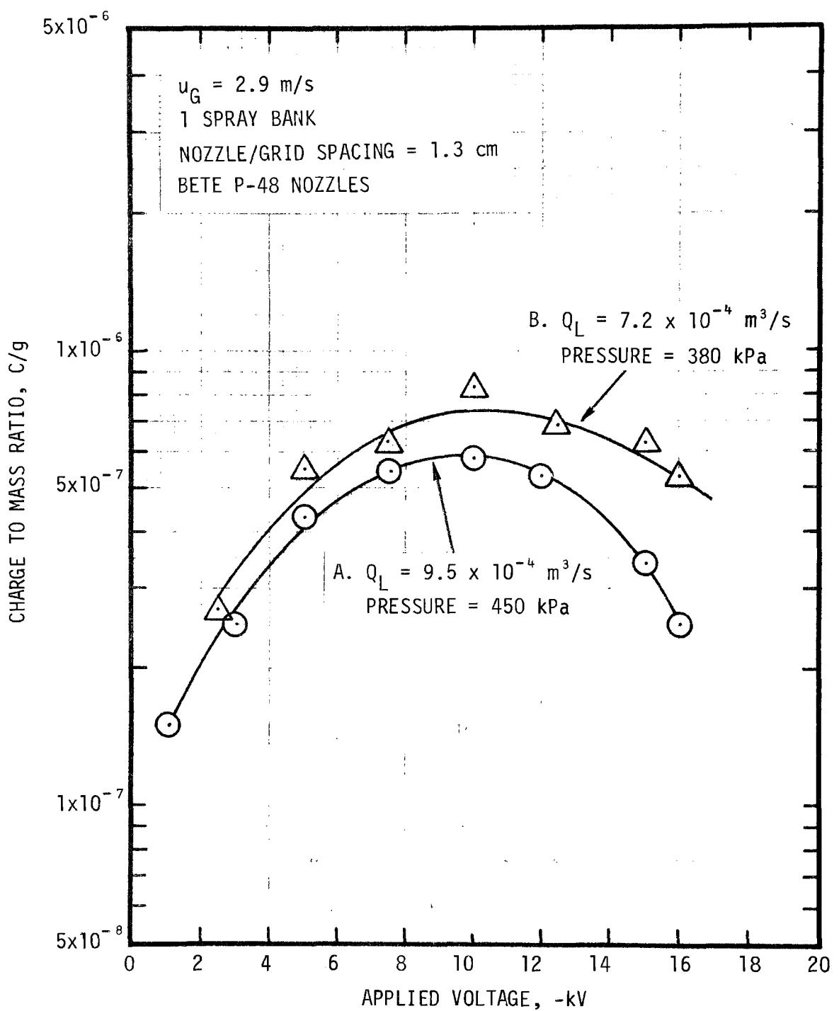
Figure 8. Measured charge level on drops.
