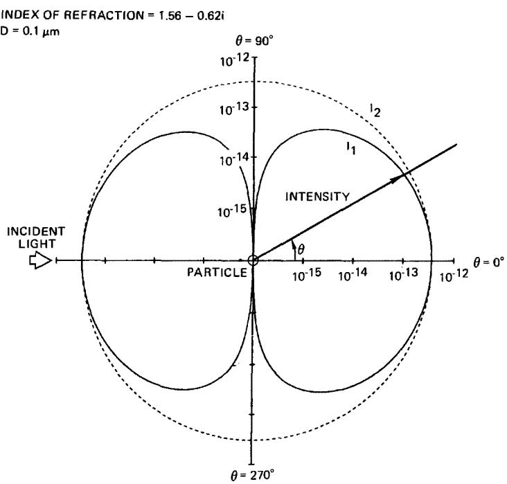
Figure 2. Typical Rayleigh Scattering Intensity Pattern ( $\lambda = 0.647 \mu\text{m}$ )
