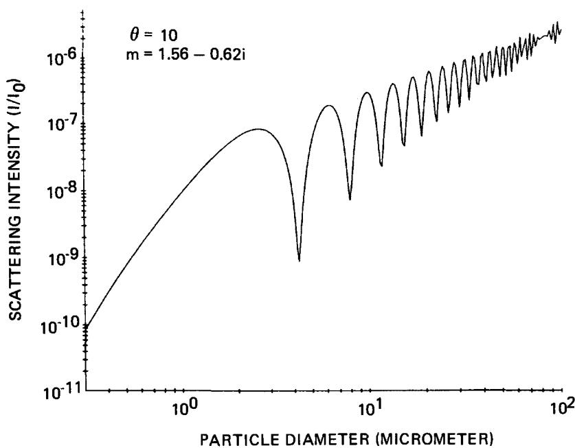
Figure 5. Typical Oscillatory Response Curve of Mie Scattering With Respect to Particle Size ( $\lambda = 0.647 \mu\text{m}$ )
