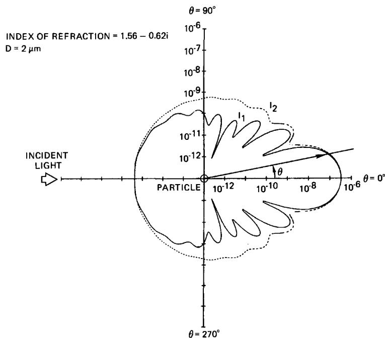
Figure 3. Typical Mie Scattering Intensity Pattern From An Absorbing-Sphere ( $\lambda = 0.647 \mu\text{m}$ )
