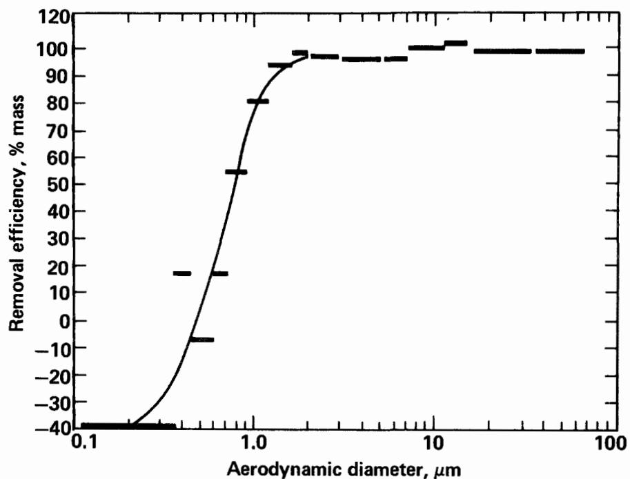
Figure 1. Removal efficiency vs particle-size curve determined for a high-energy, venturi wet scrubber.
