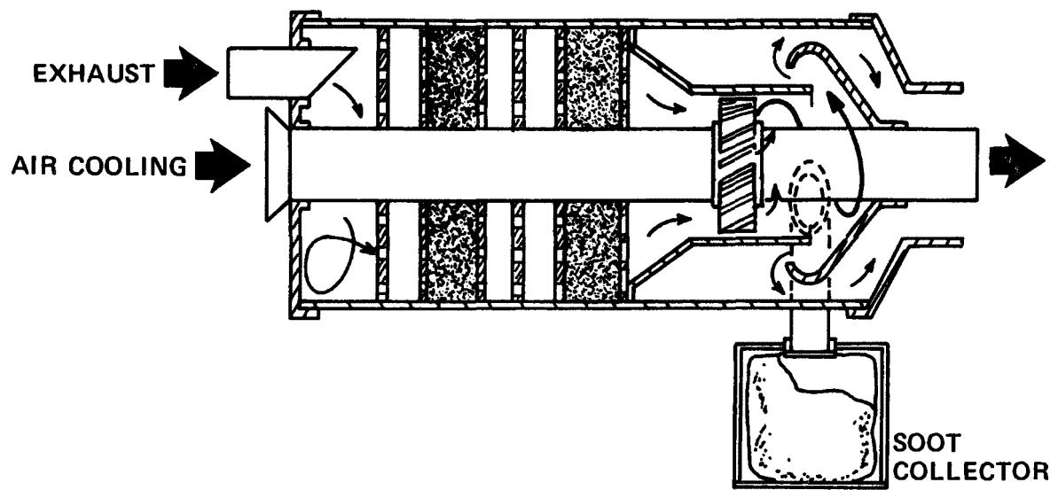
Figure 2. Aut-ainer filter with cyclone soot collector.
