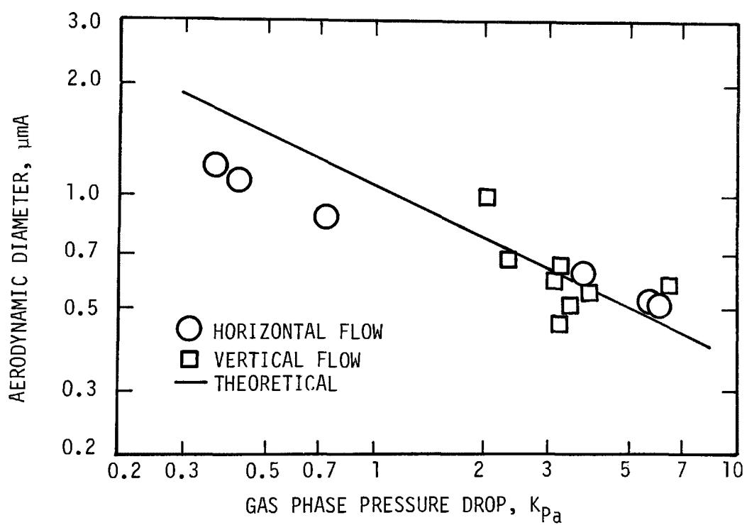
Figure 4. Comparison of particle collection characteristics of the A.P.T. Dry Scrubber with the A.P.T. cut/power relationship.
