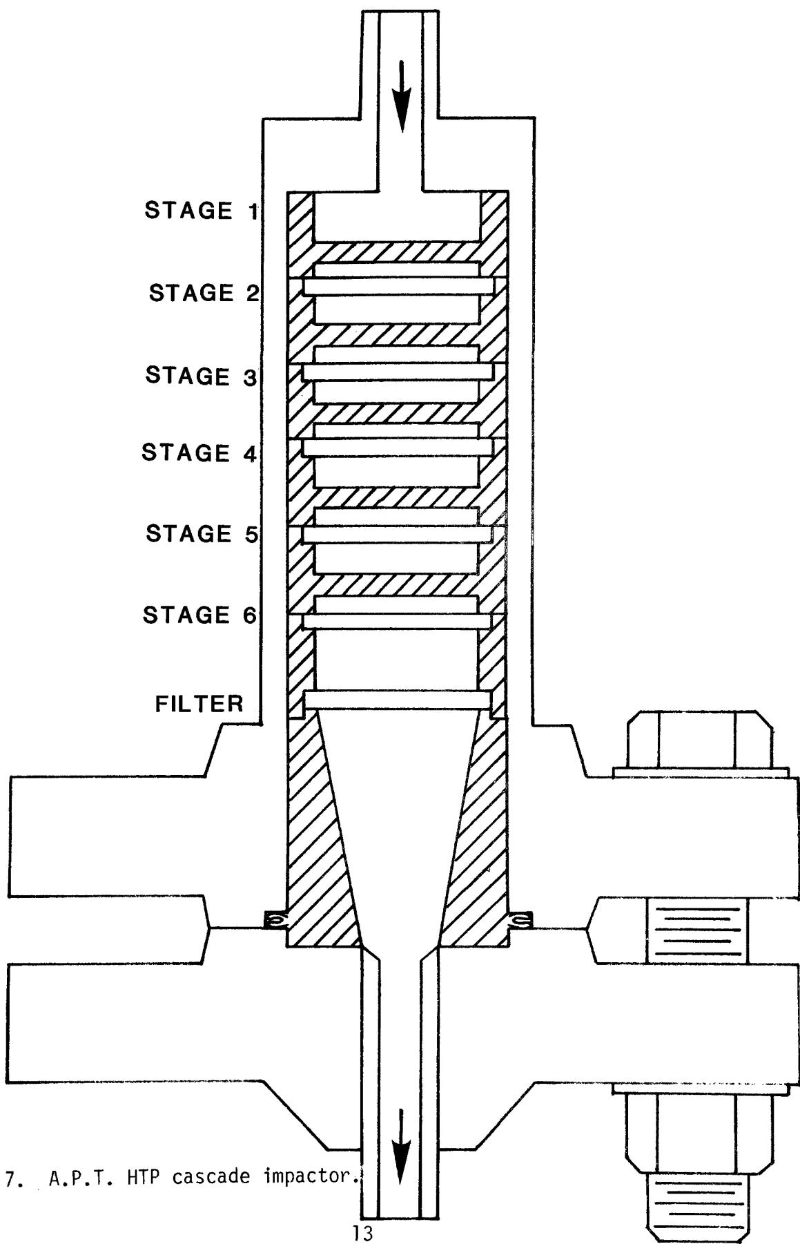
Figure 7. A.P.T. HTP cascade impactor.
