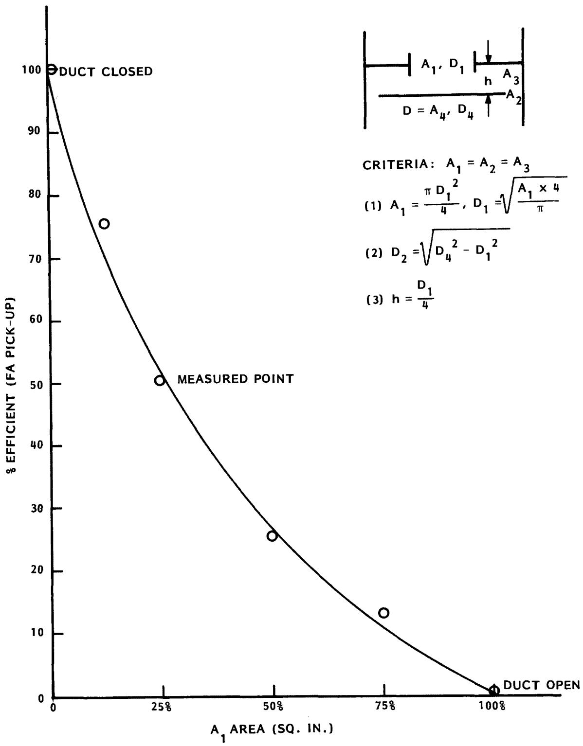
Figure 7. Curve of % efficiency of fly ash pickup vs hole-plate-space area developed from original data from bench scrubber.
