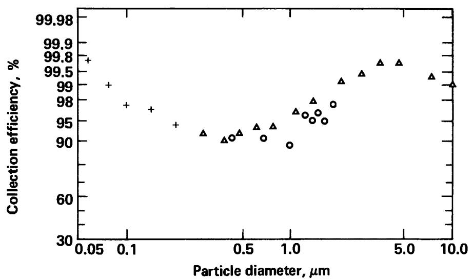
**Figure 2.** Removal efficiency vs particle-size curve of a cold-side ESP reported in McCain et al. *J. Air Pollut. Contr. Assoc.* 25, 117-21 (1975). Reprinted with permission; copyright 1975 Air Pollution Control Association.
