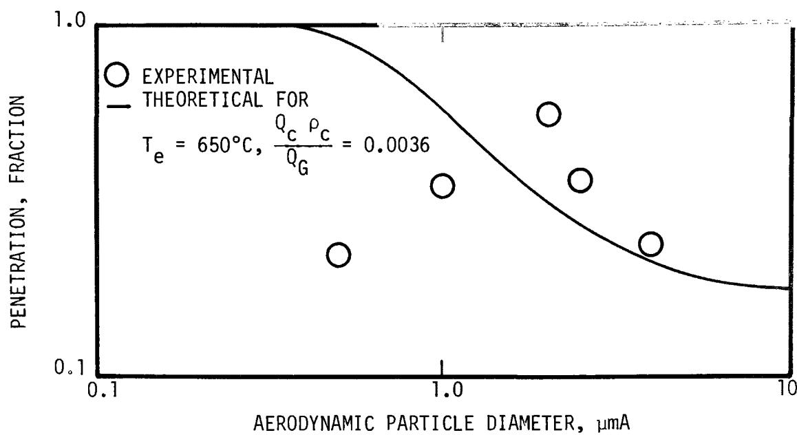
Figure 5. Particle penetration with nickel collectors.
