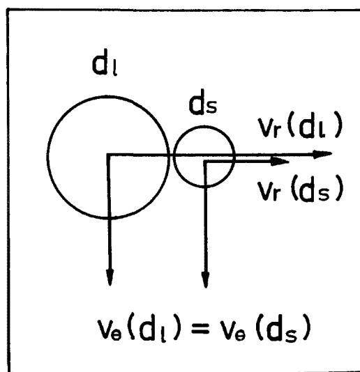
FIGURE 1. COLLISION DUE TO DIFFERENT RADIAL VELOCITIES OF PARTICLE
