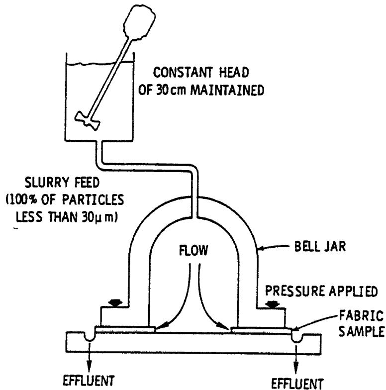
Figure 4. Laboratory Instrument used to evaluate in-plane flow of slurries through fabrics.
