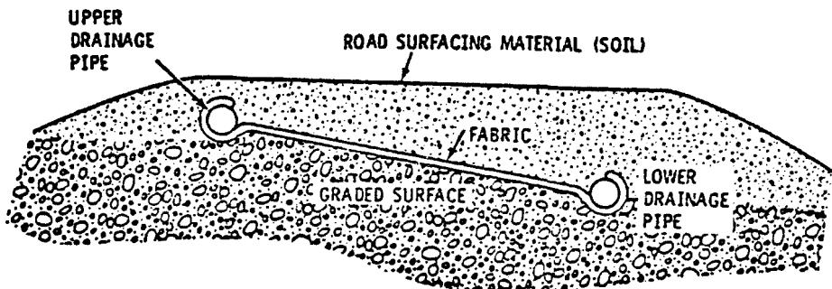
Figure 5. Self-watering road for emission control. Water is pumped from the lower drainage pipe to the upper drainage pipe externally.
