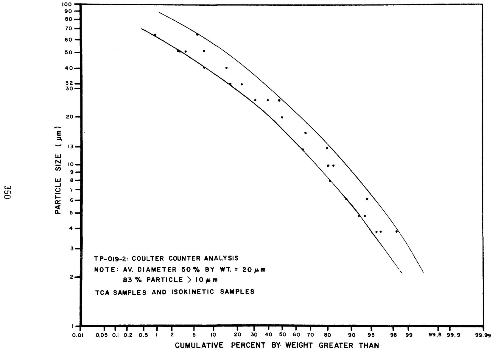
Figure 6. Cyclone Penetration Particulate Size Distribution Data
