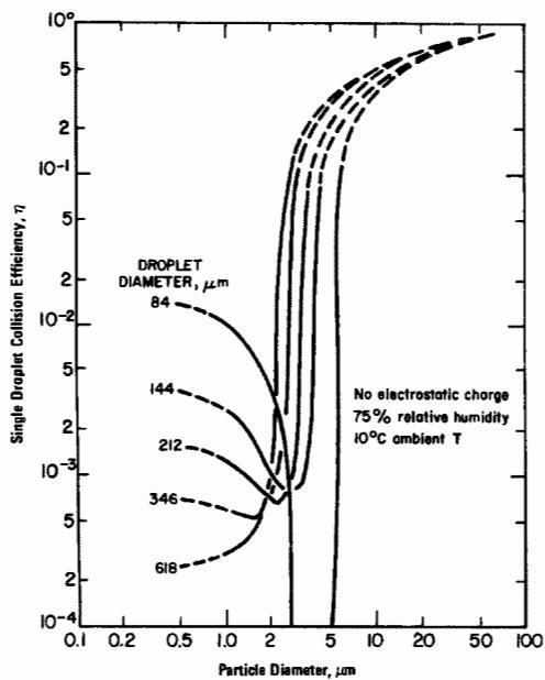
**Figure 2a.** Effect of droplet diameter on collision efficiency.
