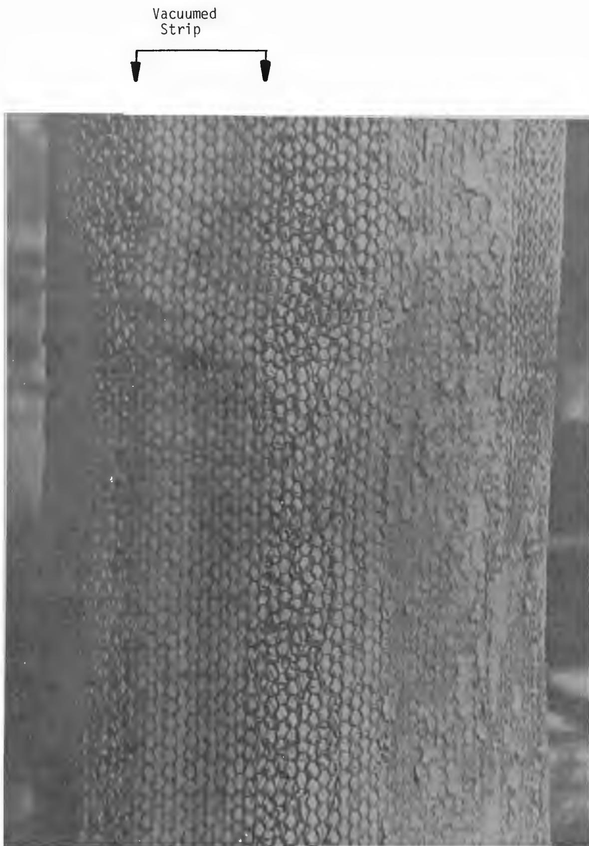
Figure 9. Ceramic filter bag (No. 3) closeup of vacuumed strip.
