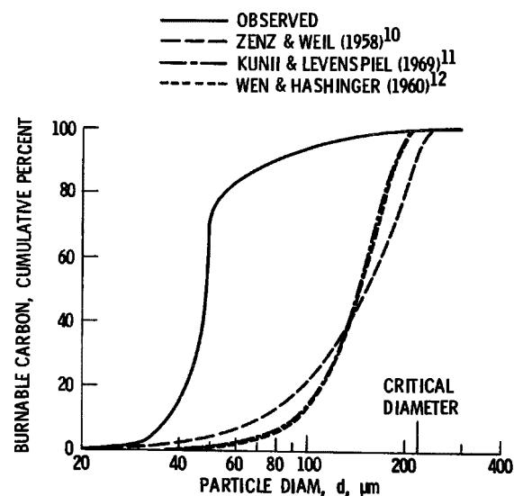
Figure 11 Comparison of calculated and observed size distribution of entrained burnable carbon. All calculations use the model of Horio, et al. (1977)<sup>7</sup> but with different elutriation correlations.
