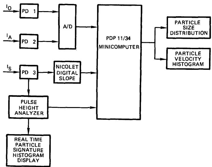
Figure 11. Block Diagram of SANFS Experiment Data Acquisition System
