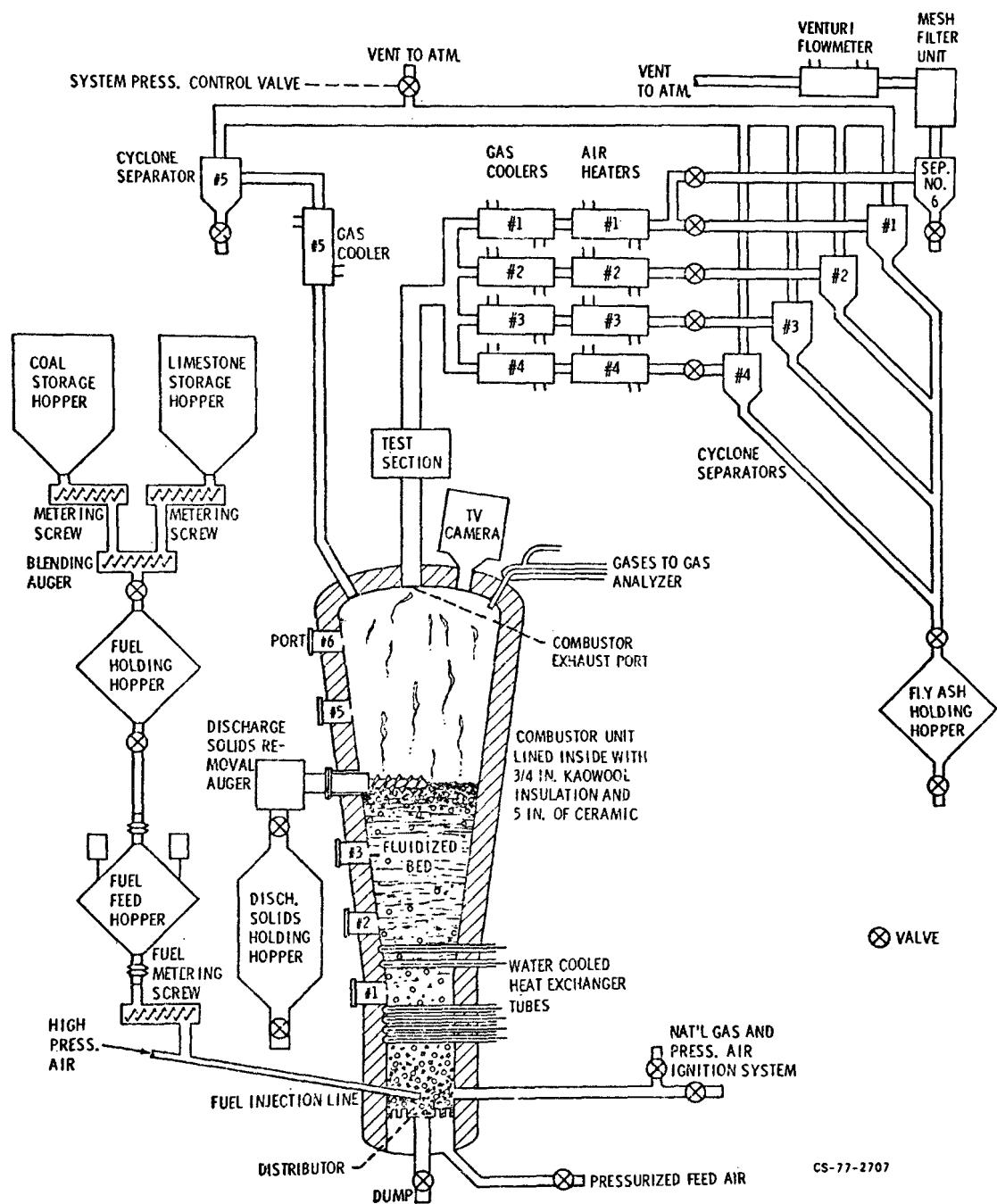
Figure 1 Schematic of LeRC pressurized fluidized bed combustor.
