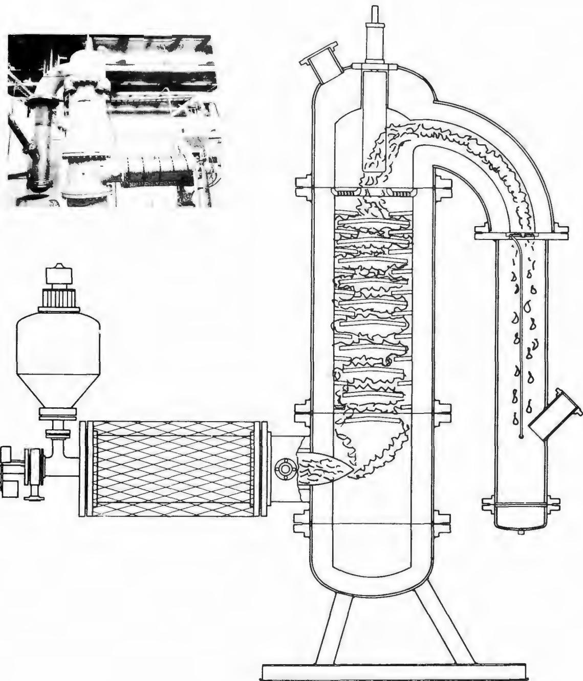
**Figure 1.** Overall view and schematic cross section of "Sticky Wall Process" hot gas clean-up test apparatus. Oil burner and fly ash feeder on extreme right of the photograph feed hot, dirty gas through horizontal pipe into centrifugal separator in lower portion of vertical cylinder where large particles are removed. Turbulent gases then pass upward among labyrinth of glass coated ceramic discs and exit through water-cooled orifice and scrubber. Excess drains into reservoir at bottom of unit.
