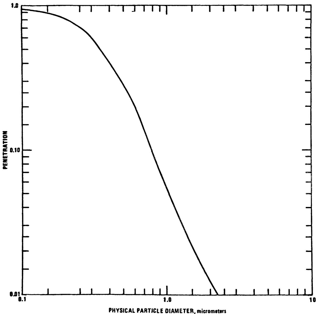
Figure 2. Penetration versus particle diameter for scrubber with pressure drop = 23 cm H<sub>2</sub>O, density - 2.4 g/cm<sup>3</sup>
