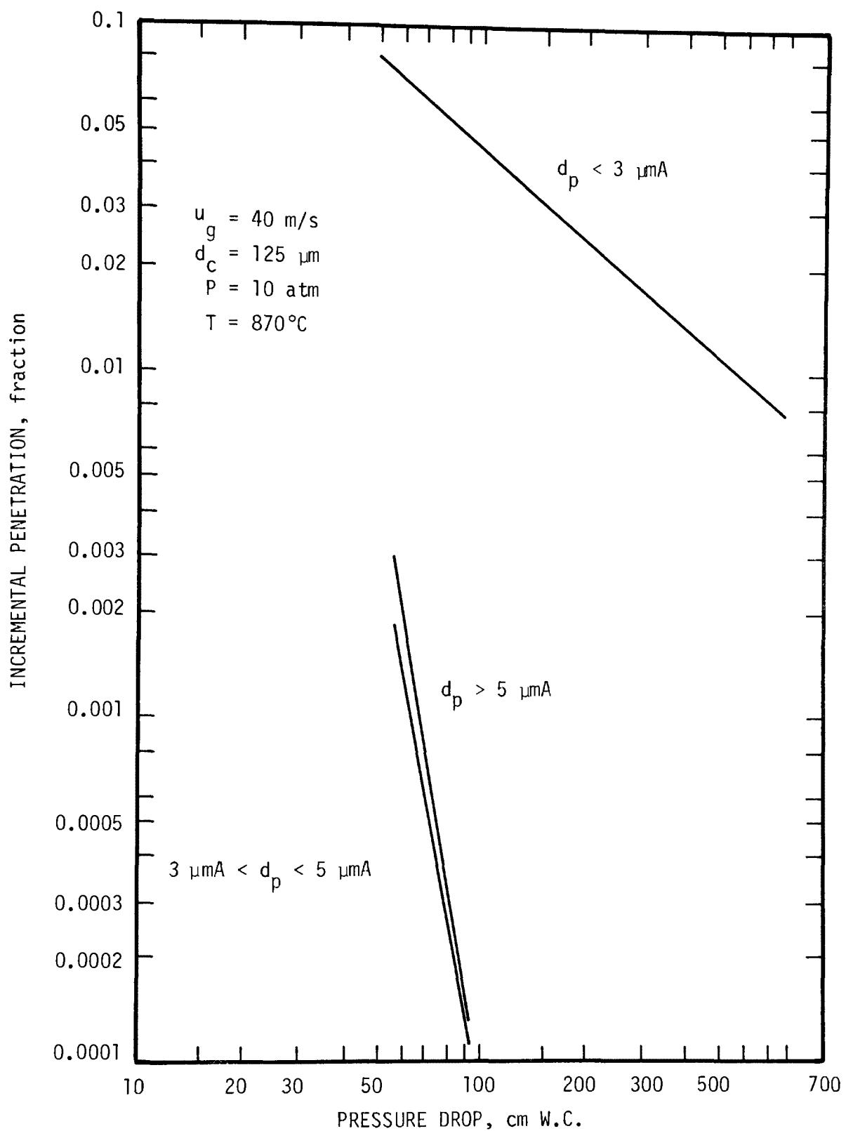
Figure 7. Predicted penetration for three size increments.
