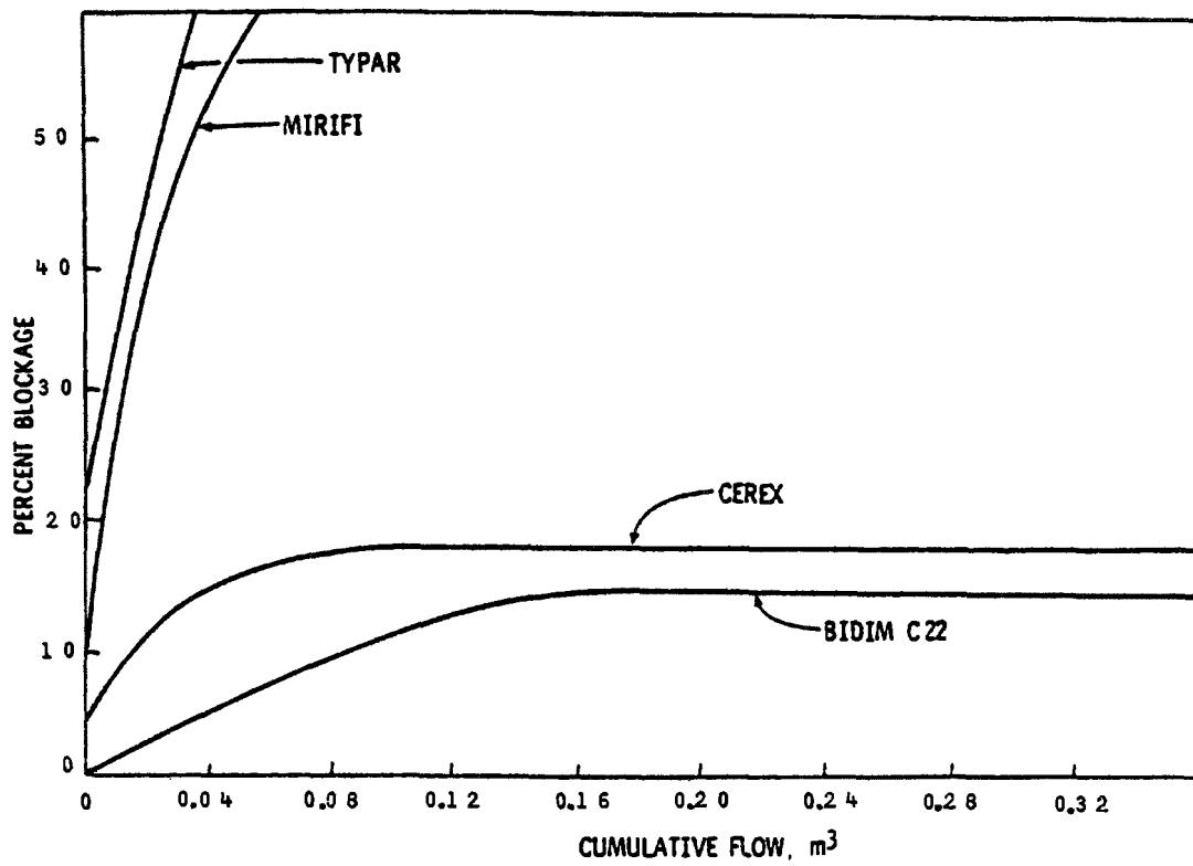
Figure 2. Blockage of fabric due to bentonite clay in water.
