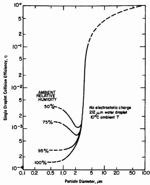
**Figure 2b.** Effect of relative humidity on collision efficiency.
