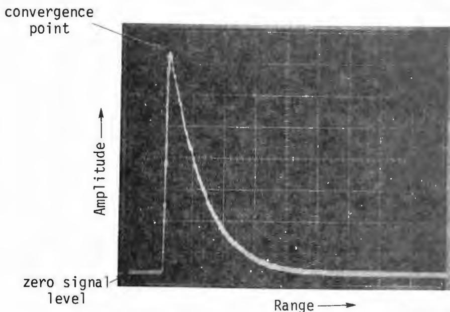
Figure 1 Linear Channel Video Signal
