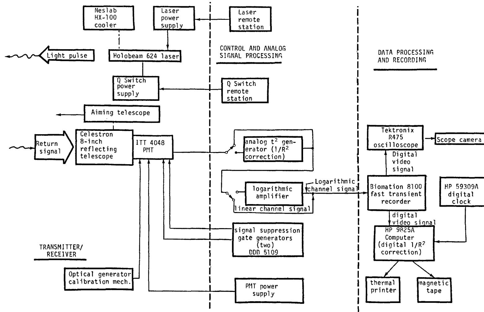
Figure 4 Schematic diagram of the Omega-i Lidar system
