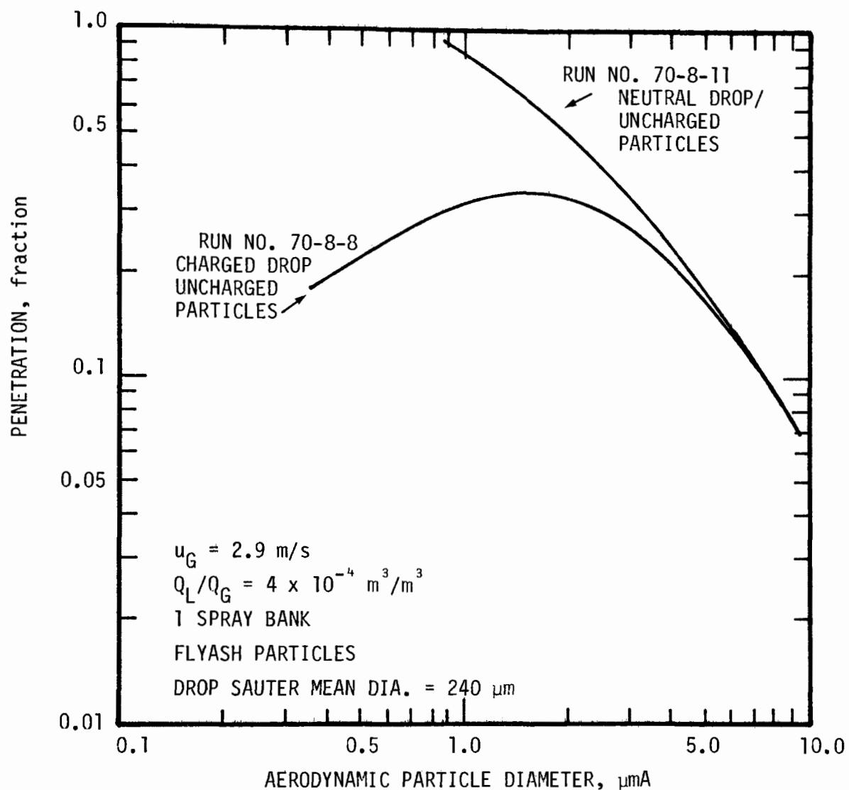
Figure 9. Experimental penetration of the SCAT scrubber.
