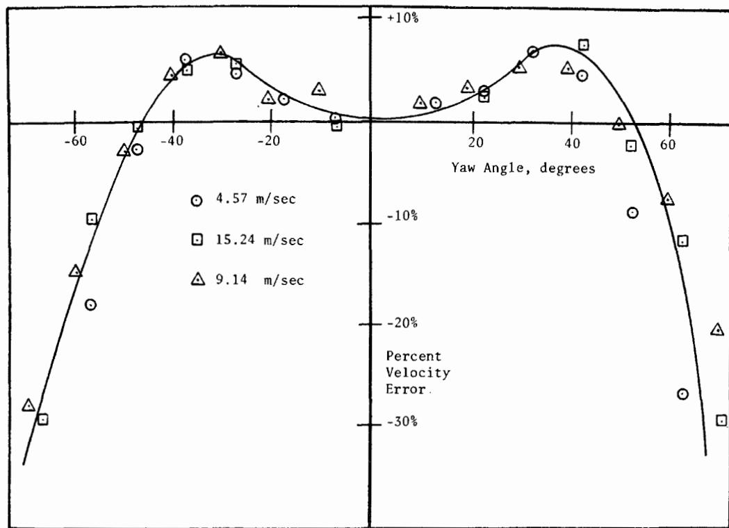
Figure 3. Velocity error vs. yaw angle for an S-type pitot tube.<sup>20</sup>
