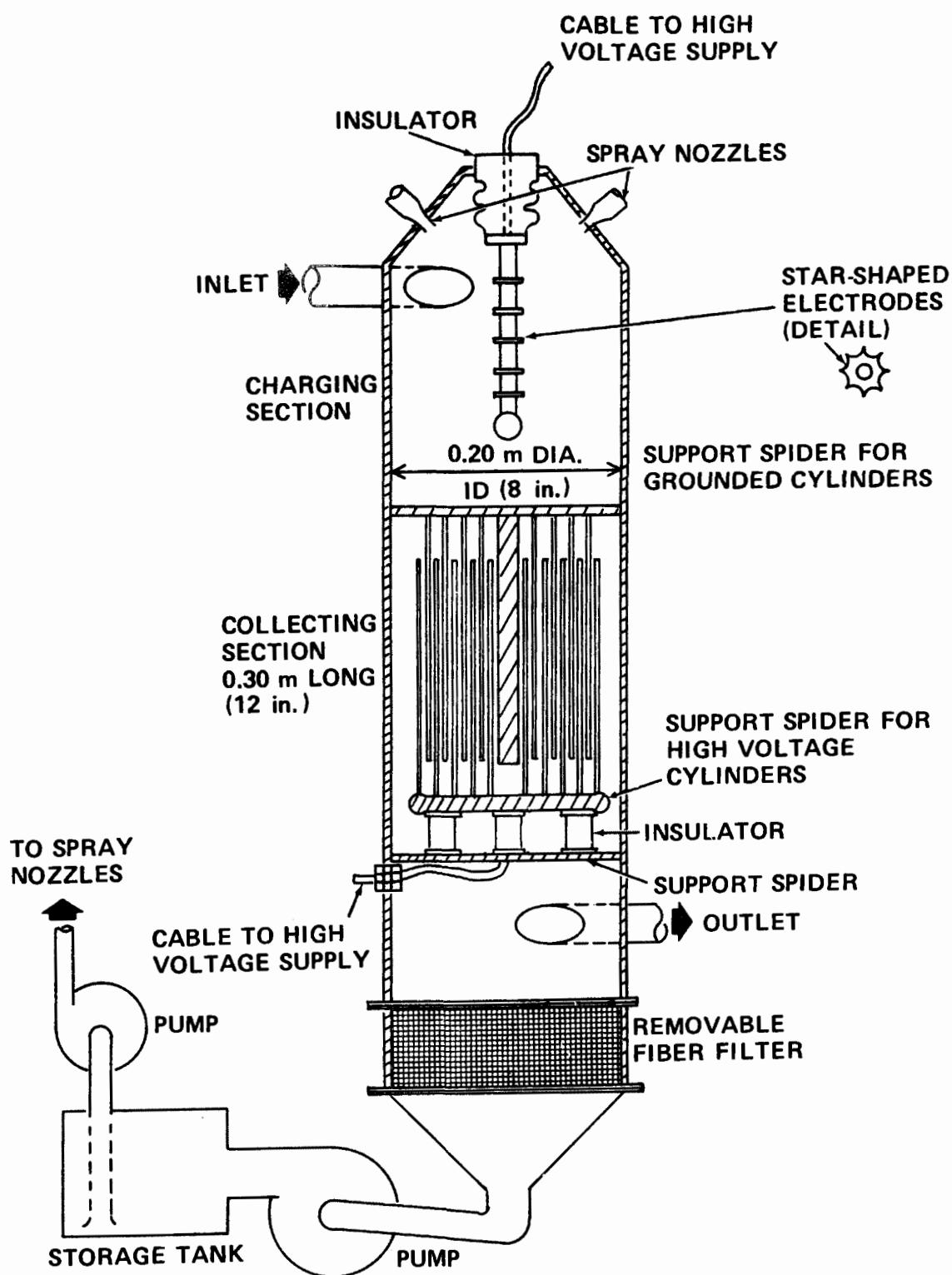
Figure 5. First prototype electrostatic precipitator for collecting diesel particulate.
