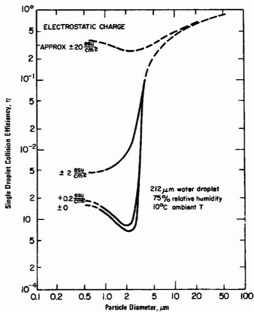
**Figure 2c.** Effect of electrostatic charge on collision efficiency.
