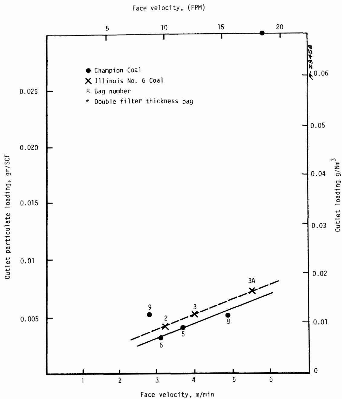
Figure 6. Acurex HTHP bag filter outlet loading vs. face velocity (averaged over first 6 hours of exposure).
