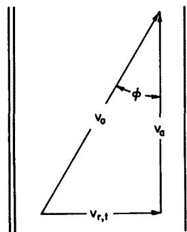
Figure 2. Velocity components in a swirling flow field.
