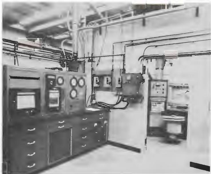
Figure 9. Operator's console with both operating controls and some experimental data collection capability.
