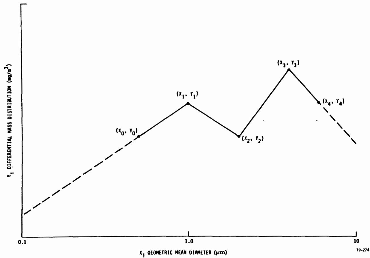
Figure 2 Linear interpolation of particle size distribution.
