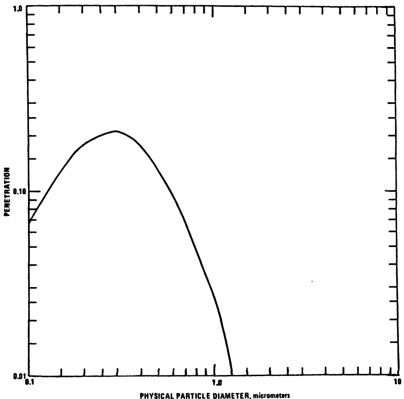
Figure 3. Graded penetration curve for ESP scrubber system - ESP penetration = 0.0771 scrubber, pressure drop = 23 cm H<sub>2</sub>O.
