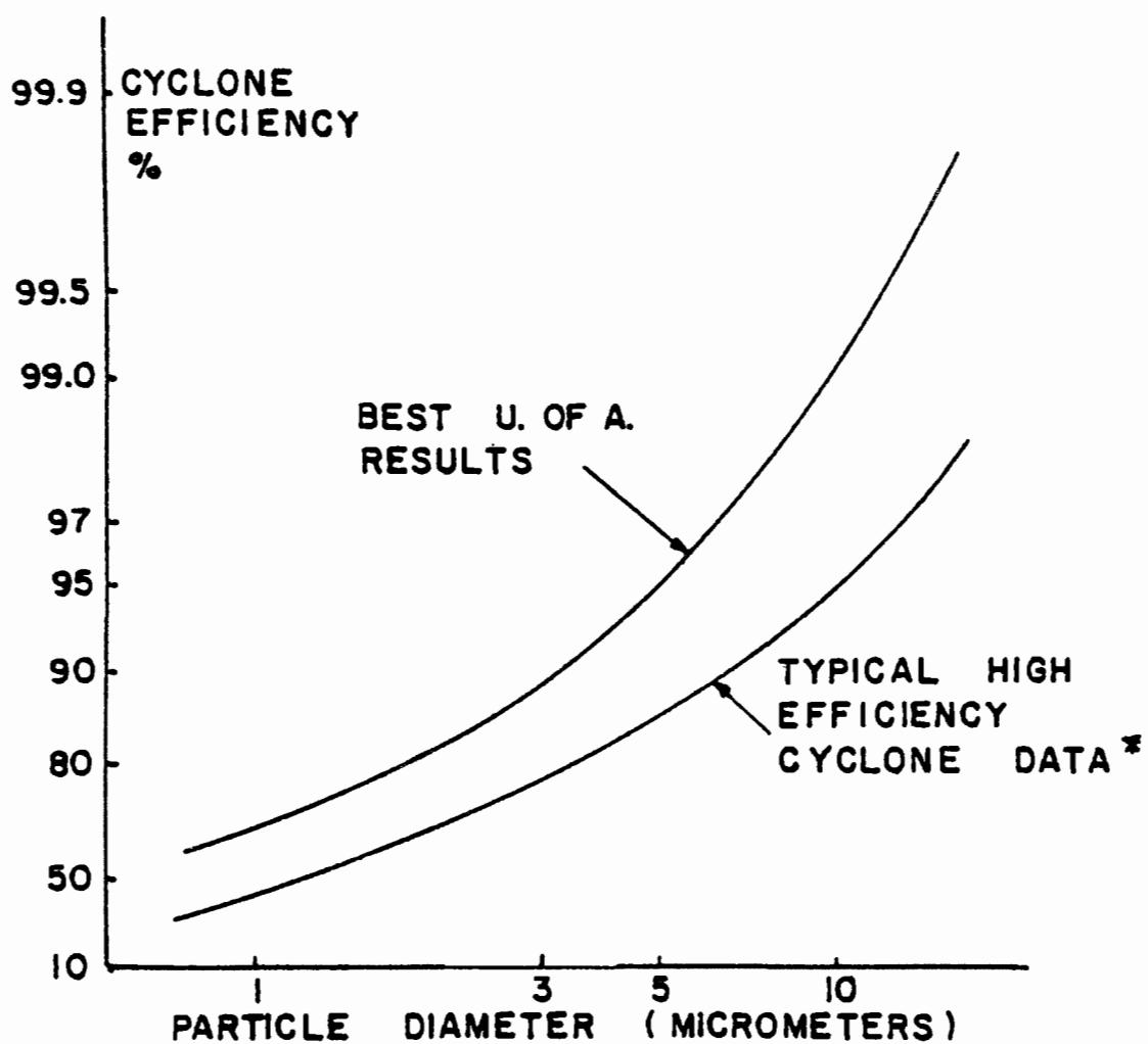
Figure 1 Improvement of cyclone efficiency with cone and charged fog, operating on cotton trash.
