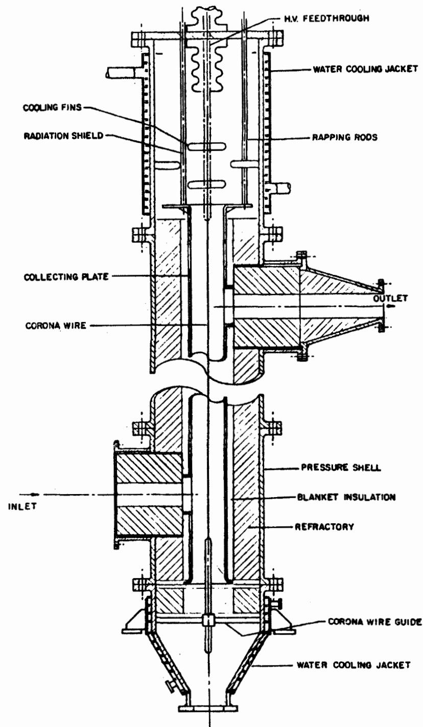
Figure 2. HTHP-ESP VESSEL
