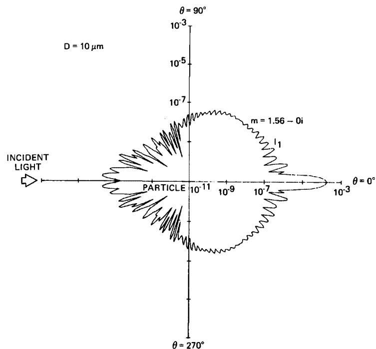
Figure 4. Typical Mie Scattering Intensity Pattern From A Nonabsorbing Sphere ( $\lambda = 0.647 \mu\text{m}$ )
