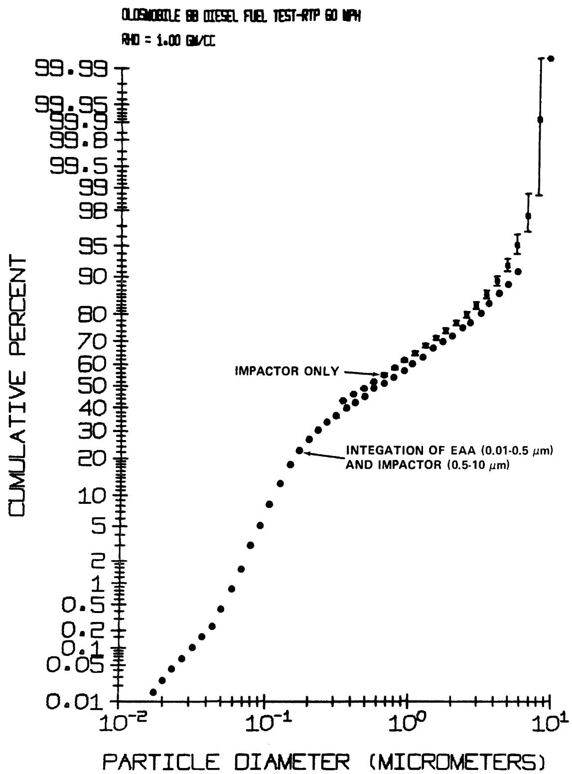
Figure 5. Particle size distribution for 60 mph condition.
