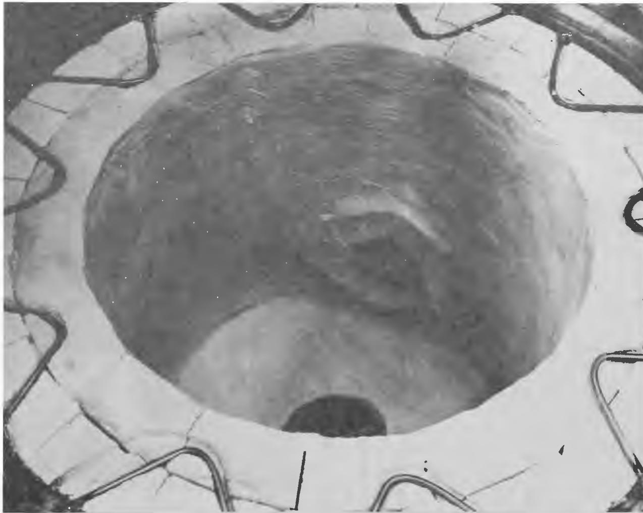
Figure 4. View inside the dome prior to installation. The exit hole for gases is visible on the side wall while the hole for the bubbler plug is partially visible in the lower center of the picture. This section is coated with a refractory cement but not powdered glass.
