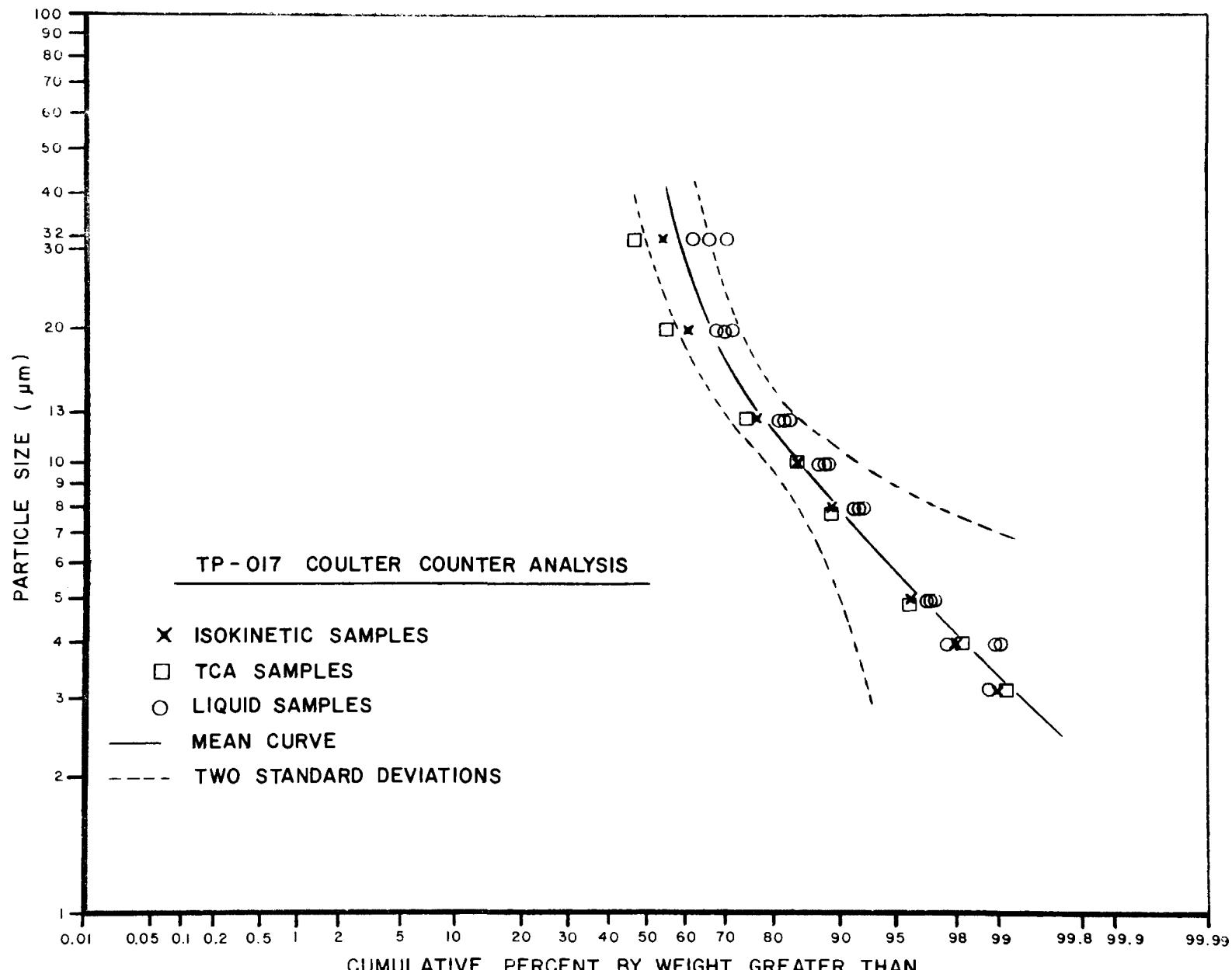
Figure 4. Cyclone Penetration Particulate Size Distribution Data
