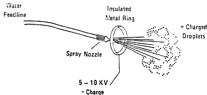
**Figure 1a. Charge induced via metal ring.**
