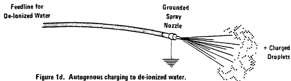
**Figure 1d. Autogenous charging to de-ionized water.**
