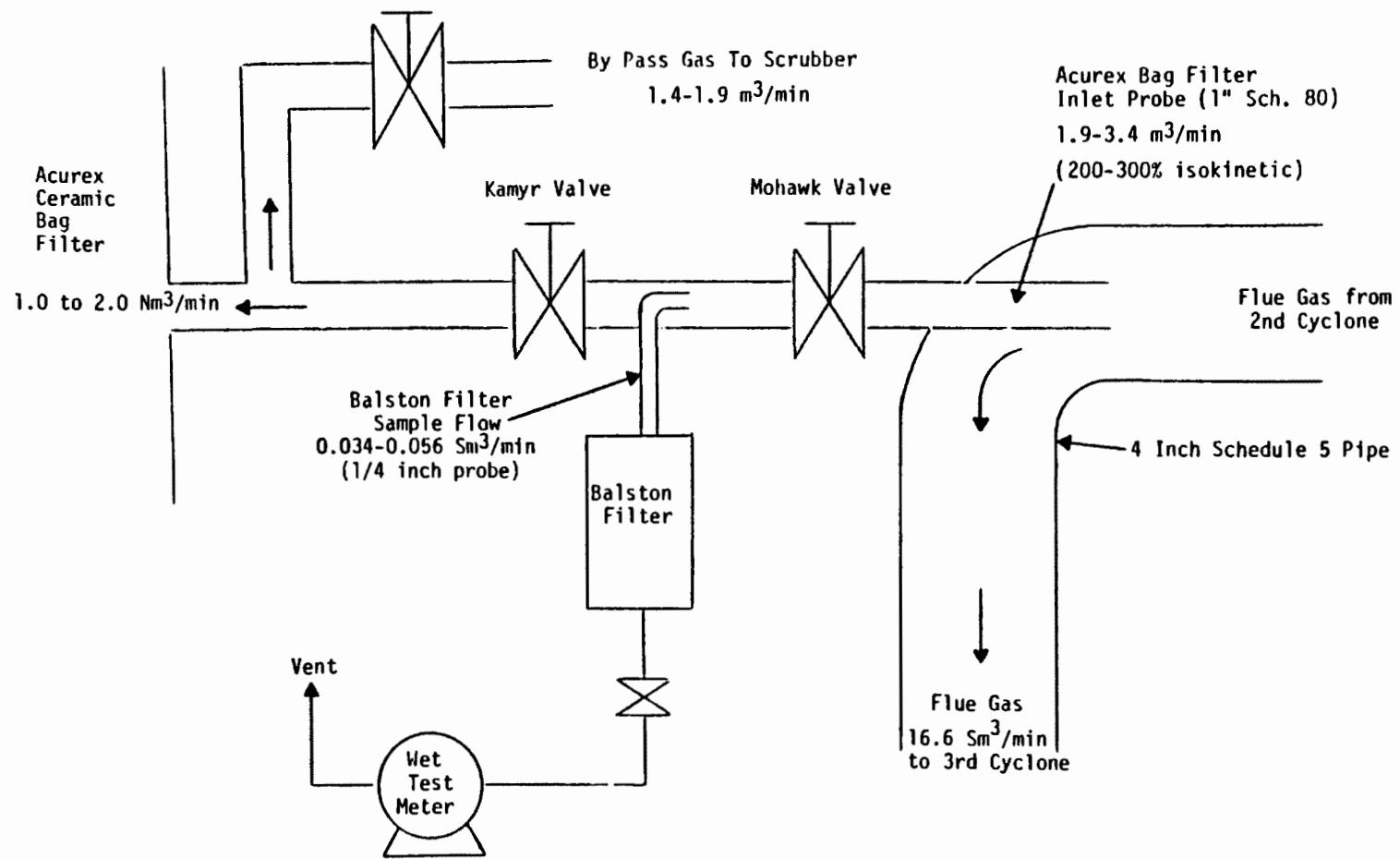
Figure 5. Acurex high-temperature ceramic bag filter gas inlet schematic.
