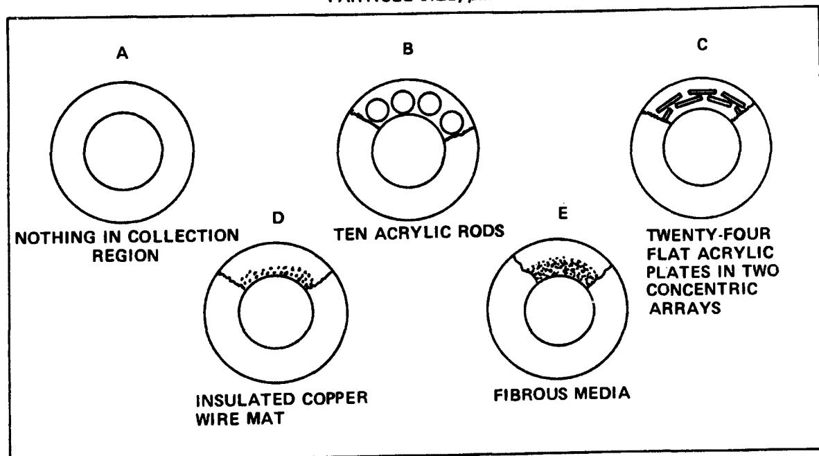
Figure 7. Collection efficiency of a concentric precipitator with dielectric collection media.<sup>8</sup>
