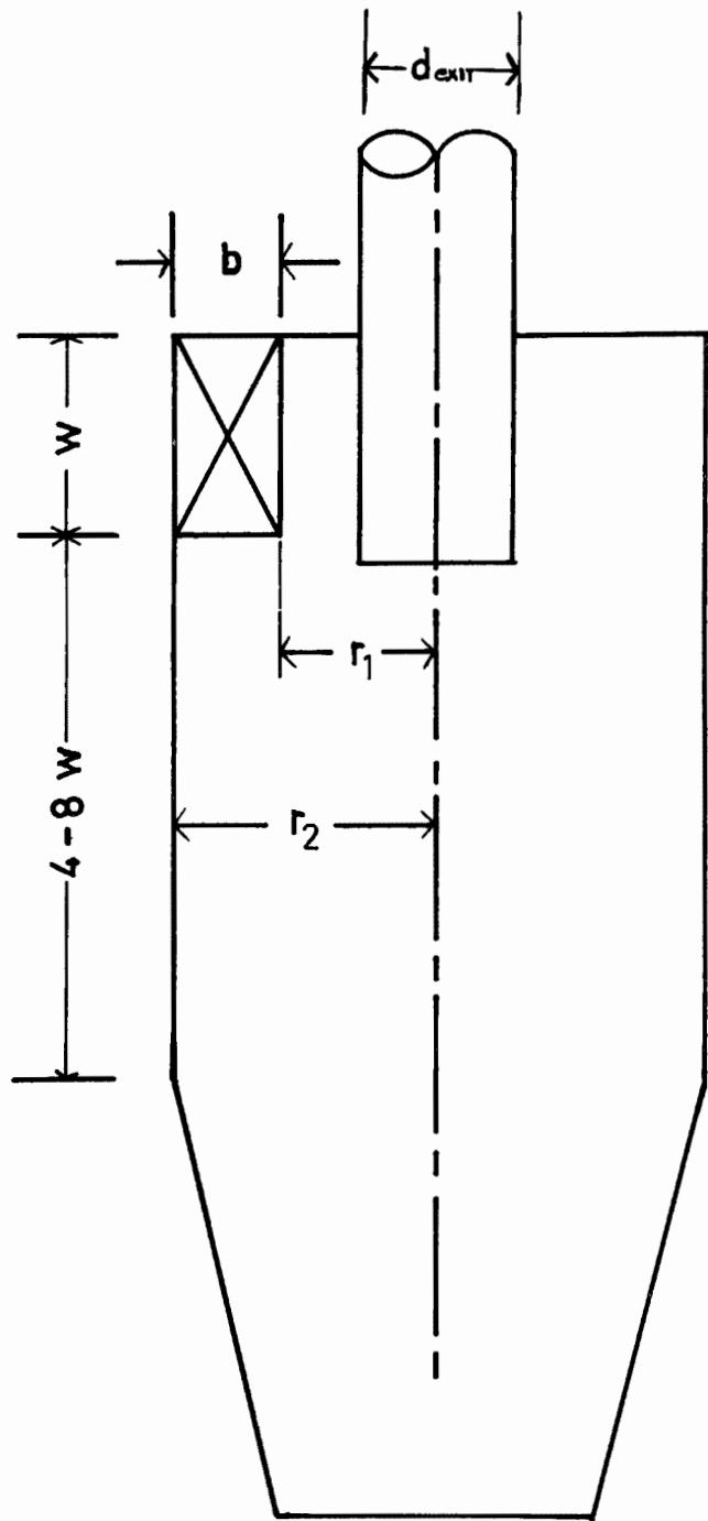
FIGURE 2. DIMENSION PARAMETERS OF CYCLONE
