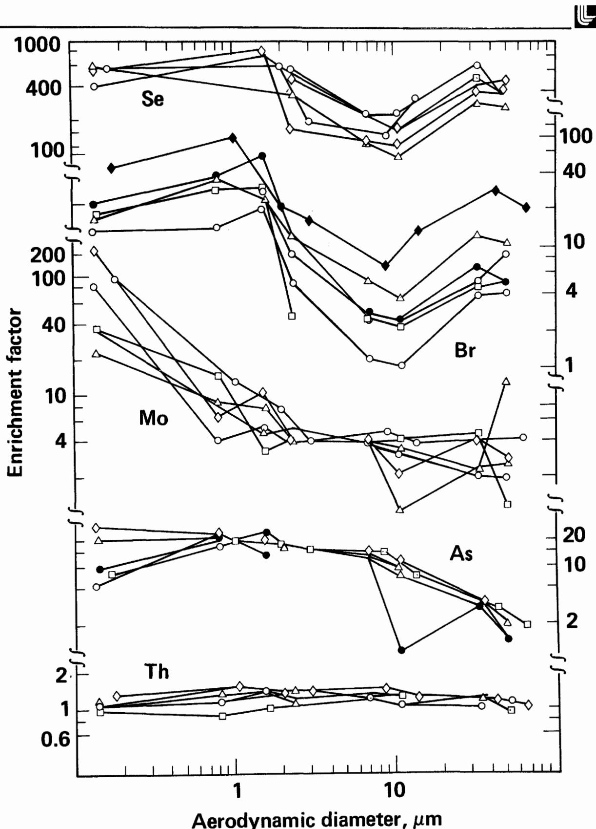
Figure 7. Relative concentration (enrichment factor) vs size profiles of fine elements associated with aerosol particles emitted from Plant C.
