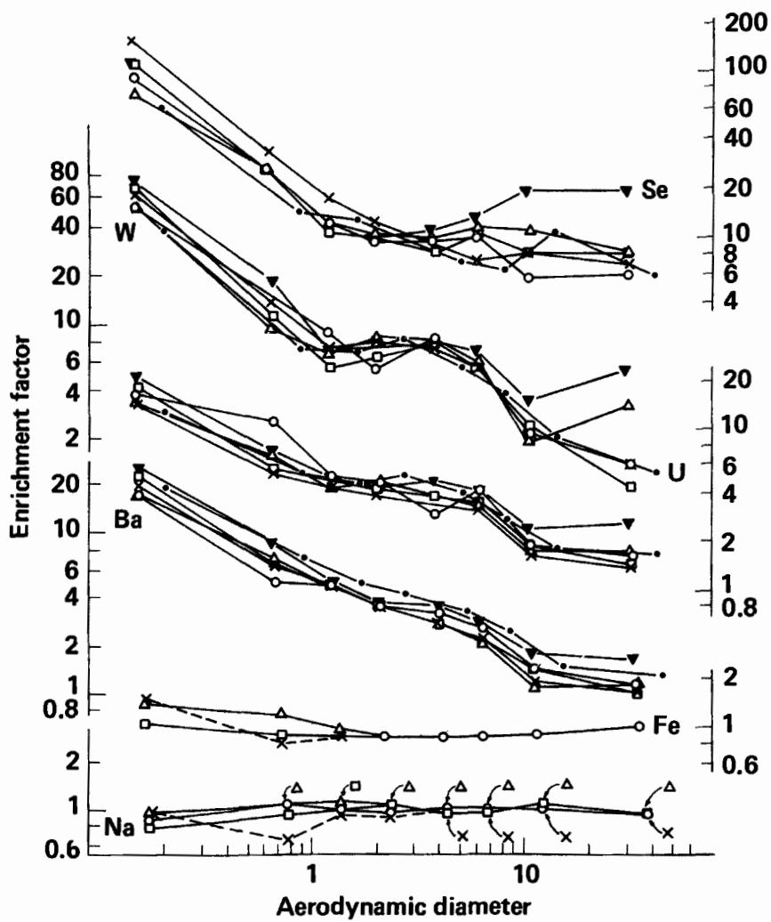
Figure 3. Concentration relative to coal vs particle-size curve for several elements contained in fly ash emitted from the ESP Unit 3.
