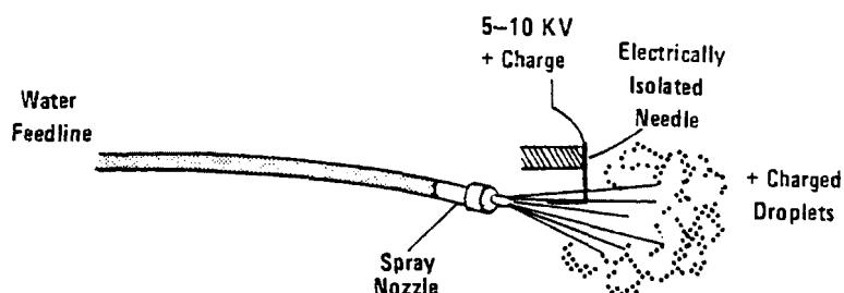
**Figure 1b. Charging via needle.**
