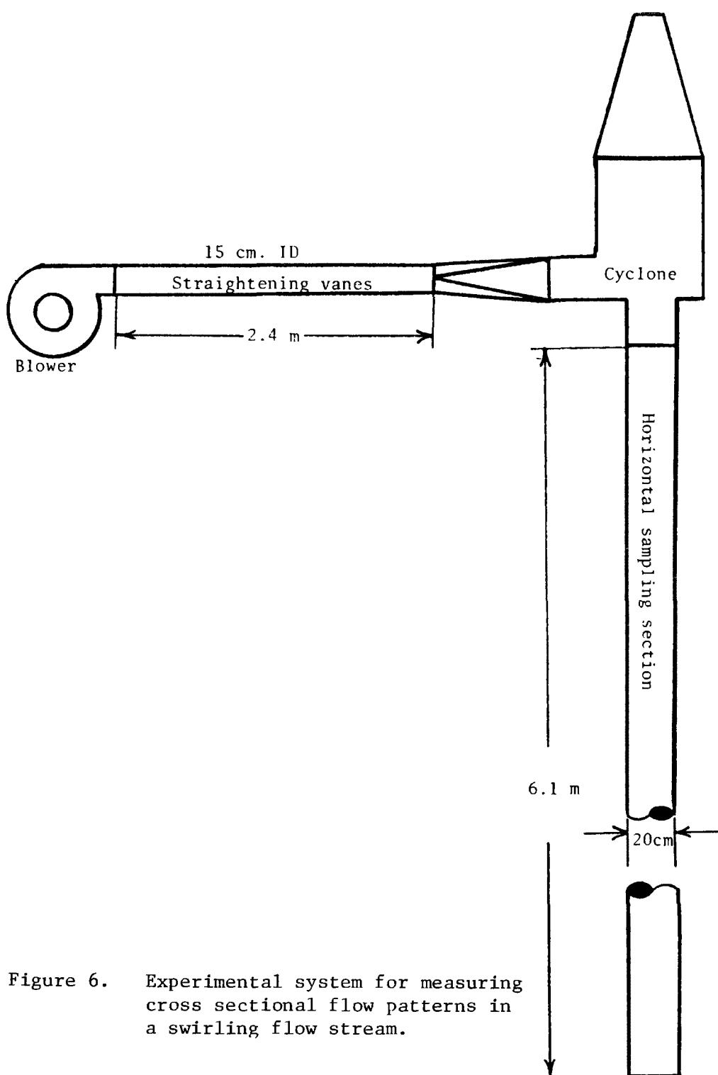
Figure 6. Experimental system for measuring cross sectional flow patterns in a swirling flow stream.
