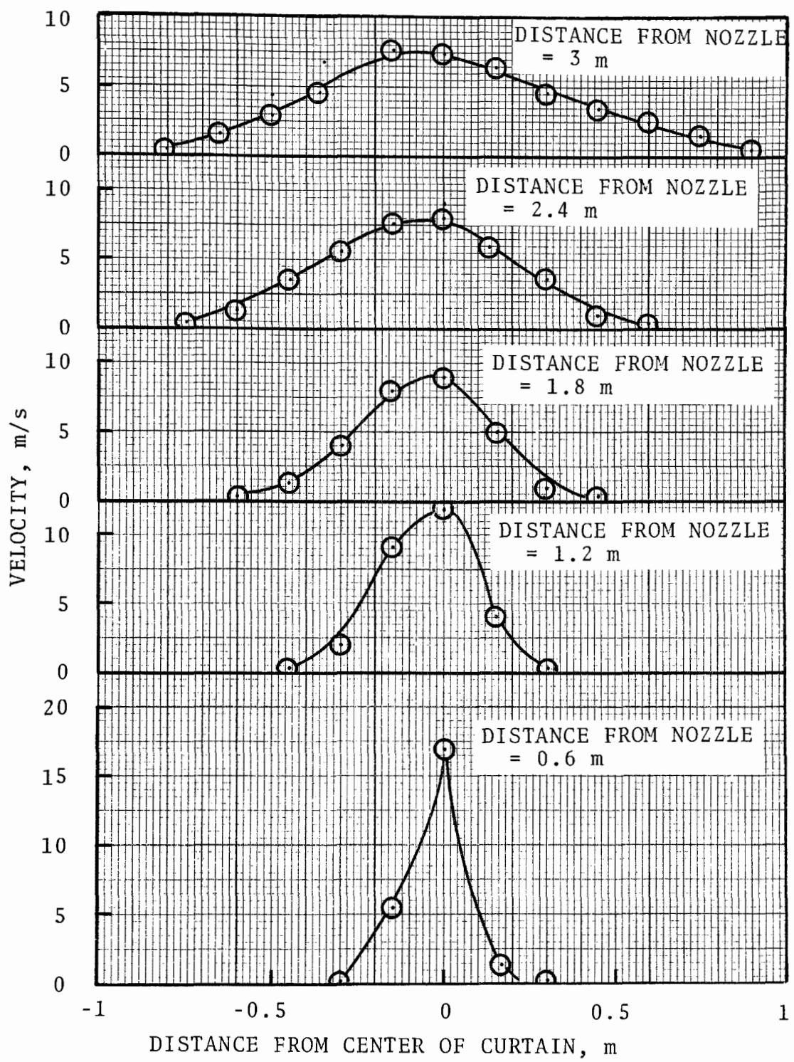
Figure 5. Experimental velocity profile.
