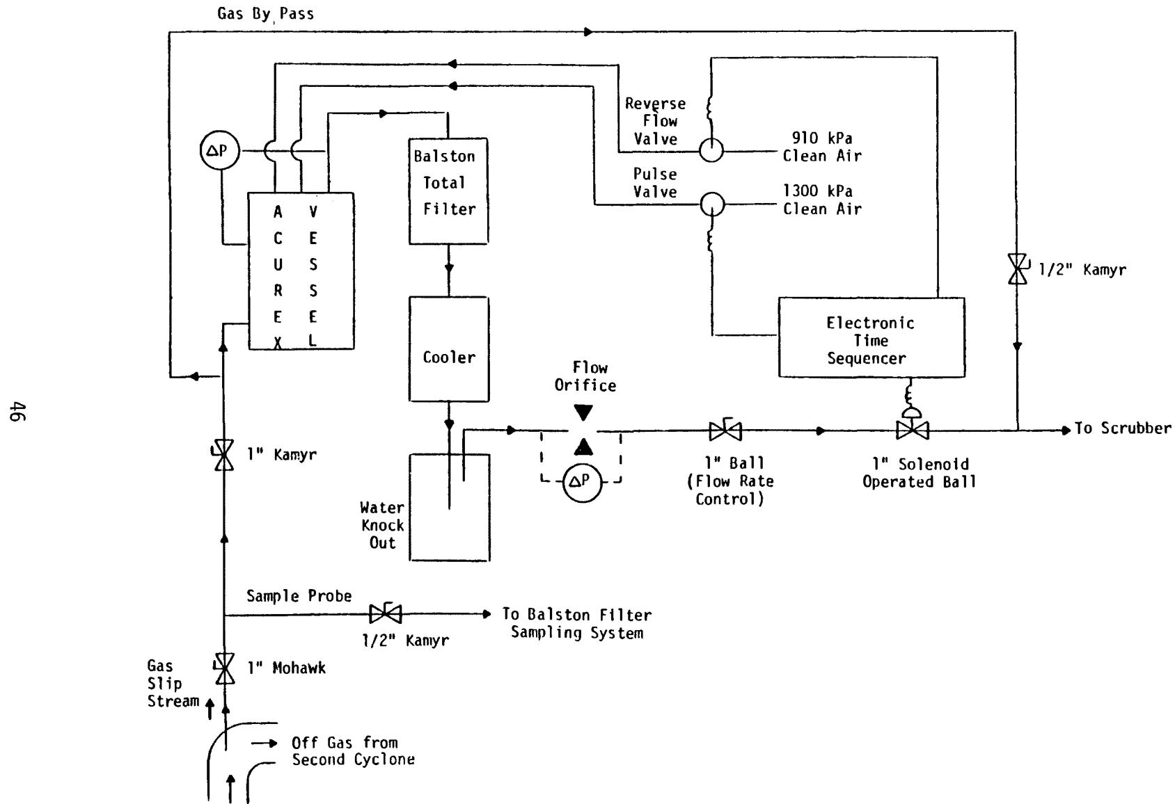
Figure 2. Acurex test filter installation schematic.
