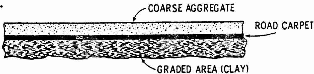
Figure 1. The Road Carpet concept, which spreads the vehicular load, prevents moisture from eroding the graded area, and keeps dirt from reaching the tires where it can be picked up and dispersed.
