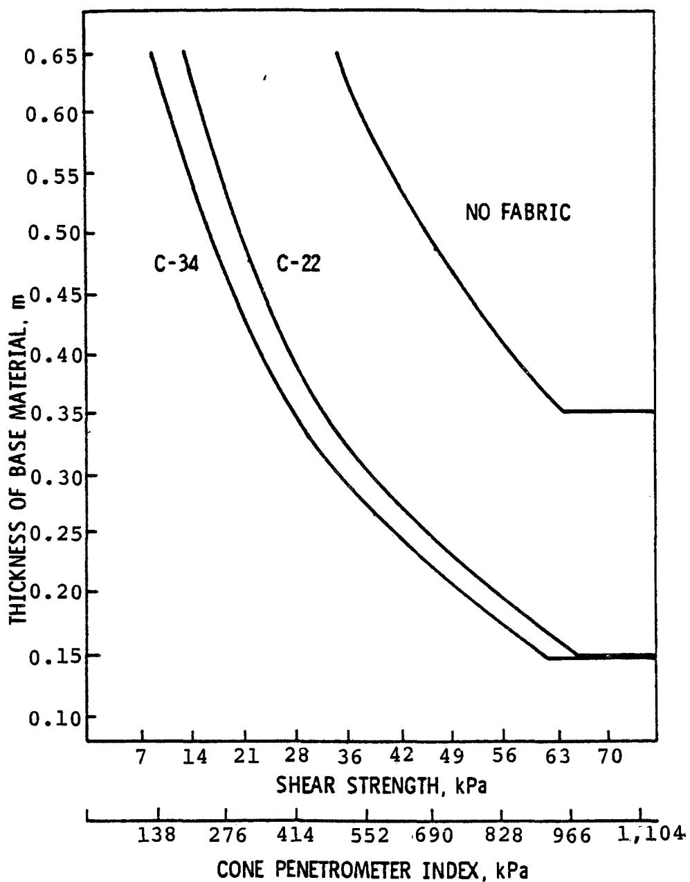
Figure 6. Design curves for 18 metric ton axle load on 10:00-20 tires for BIDIM fabric.
