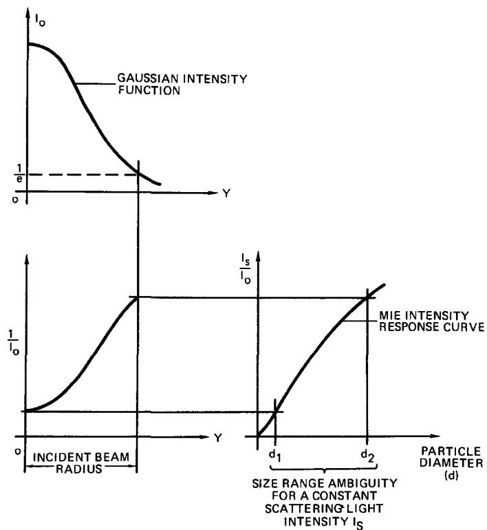
Figure 6. Illustration of Size Ambiguity Due To Nonuniform Incident Beam Intensity
