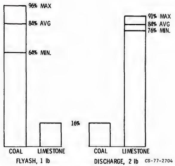
Figure 5 Source of solids removed from bed.
