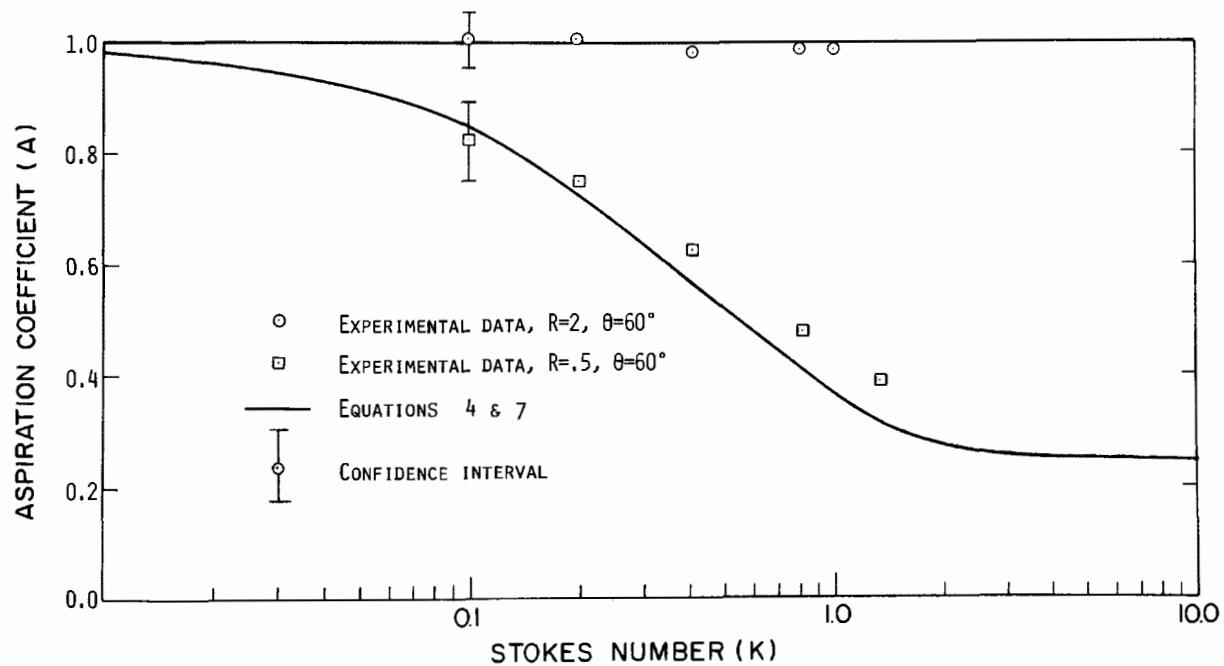
Figure 8. Sampling efficiency vs. Stokes number at  $60^\circ$  misalignment for  $R = 2.0$  and  $0.5$ .
