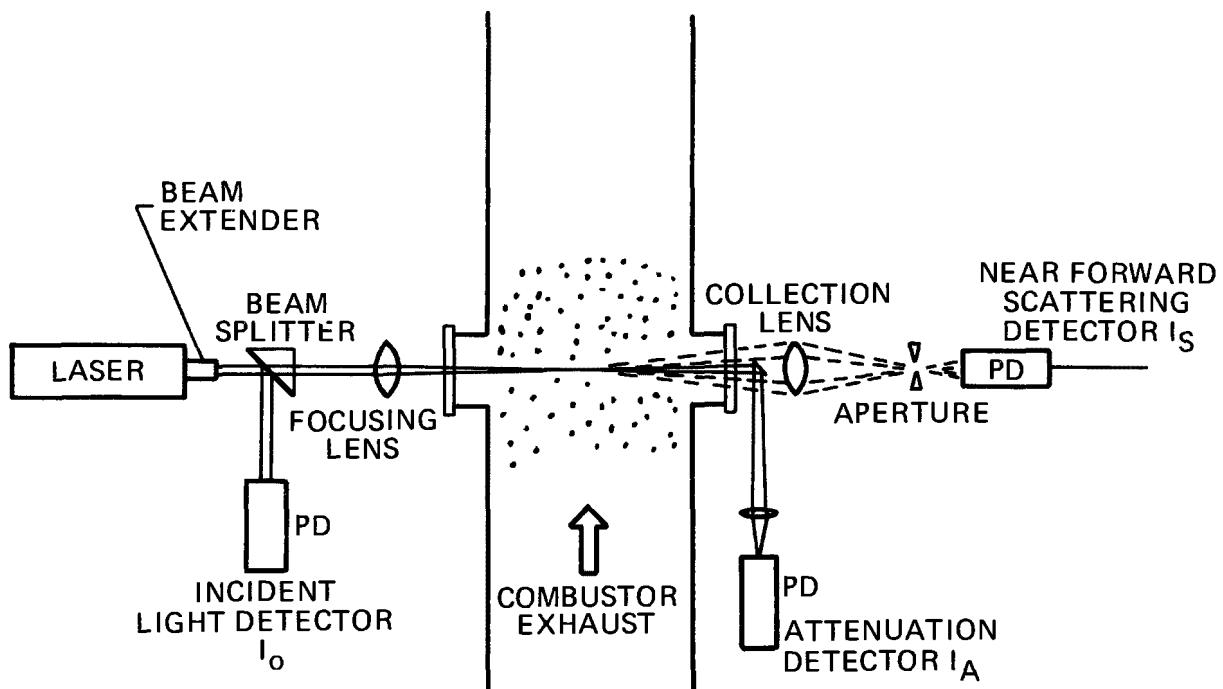
Figure 10. Schematic of the Small-Angle Near-Forward Scattering Experiment (SANFS)
