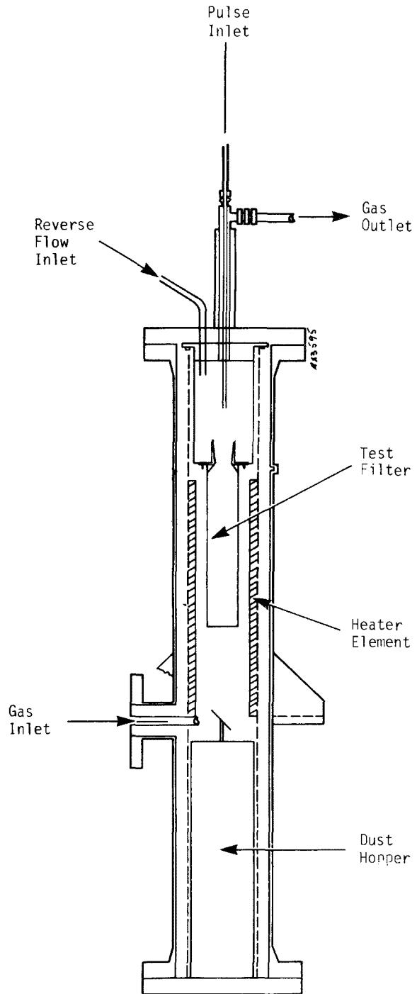
Figure 1. Filter housing pressure vessel cross section.
