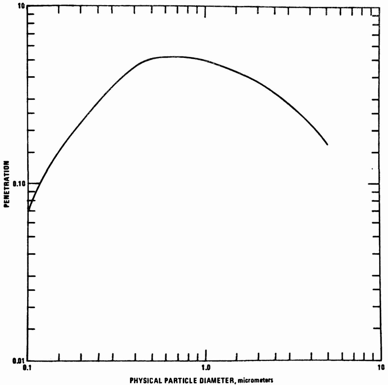
Figure 1. Graded efficiency curve for ESP with penetration of 0.0771.
