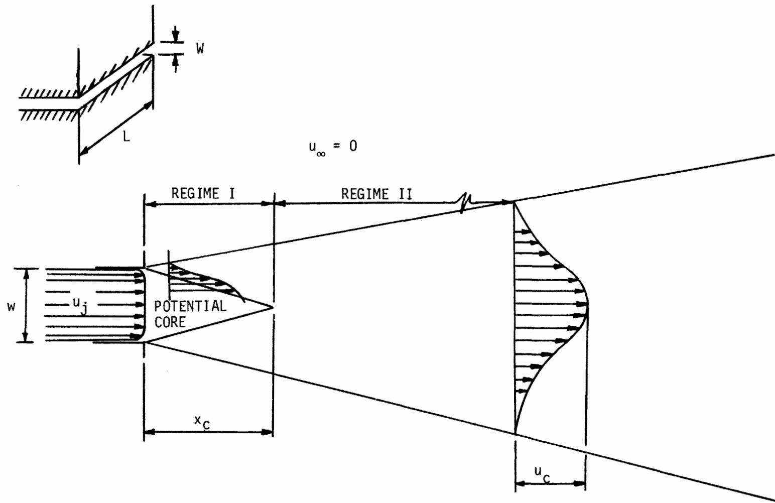
Figure 2. Two - dimensional jet with gas external velocity.
