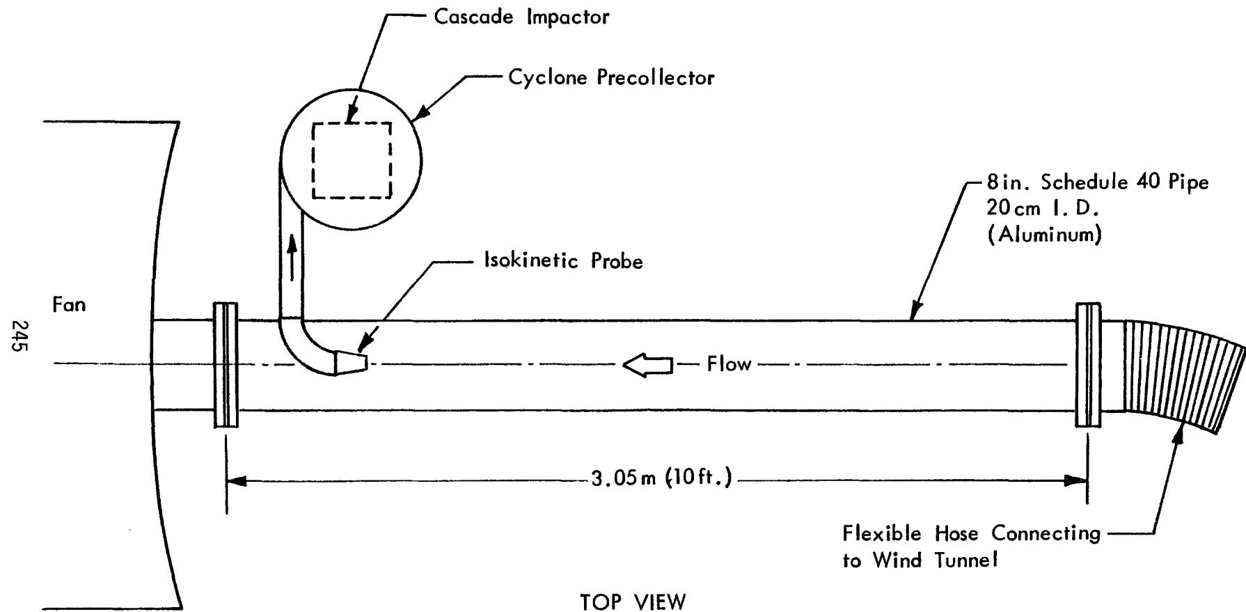
Figure 1. Emissions sampling module for portable wind tunnel.
