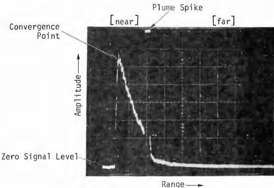
Figure 2 Linear Channel Video Signal,
