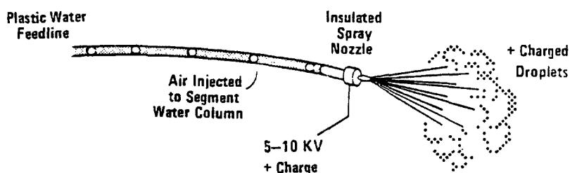
**Figure 1c. Direct contact water charging.**
