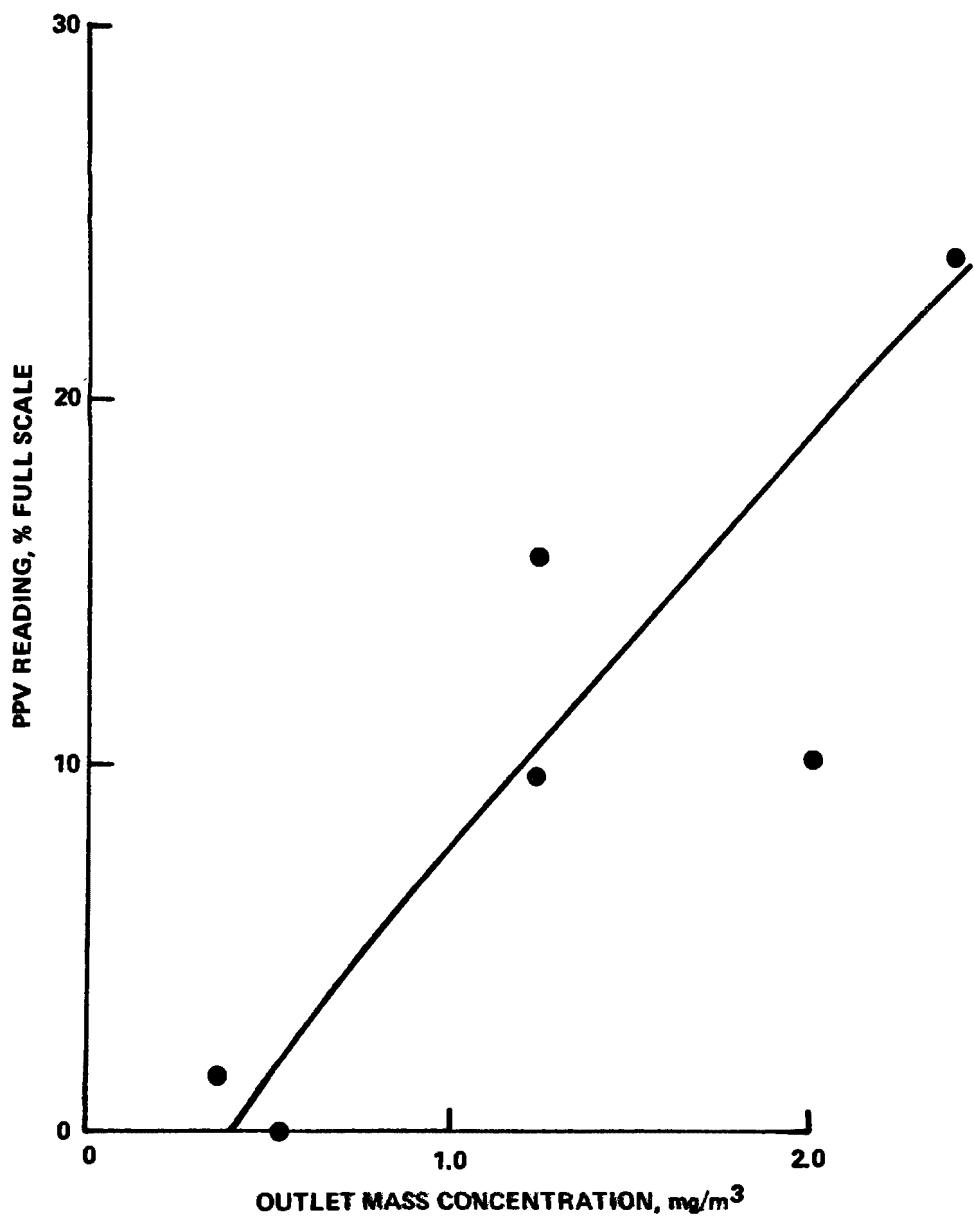
Figure 6. Relative PPV reading versus outlet mass concentration for ESP Scrubber experiments.
