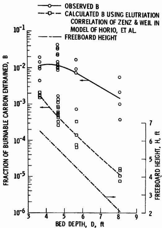
Figure 12 Effect of bed depth on entrained carbon.
