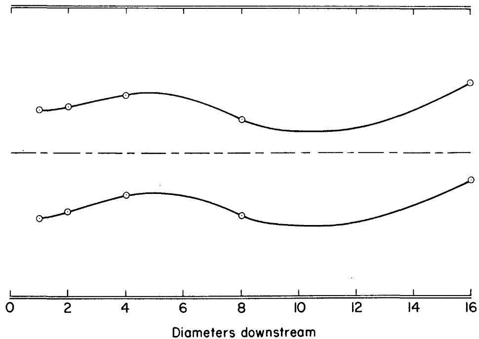
Figure 10. Location of the negative pressure region as a function of distance downstream from the cyclone.
