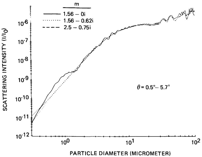
Figure 9. Calculated Mie Scattering Response Curve At Small-Angle Near-Forward Direction Using Three Wavelengths ( $\lambda = 0.647$ ,  $0.5145$ , and  $0.488 \mu\text{m}$ )
