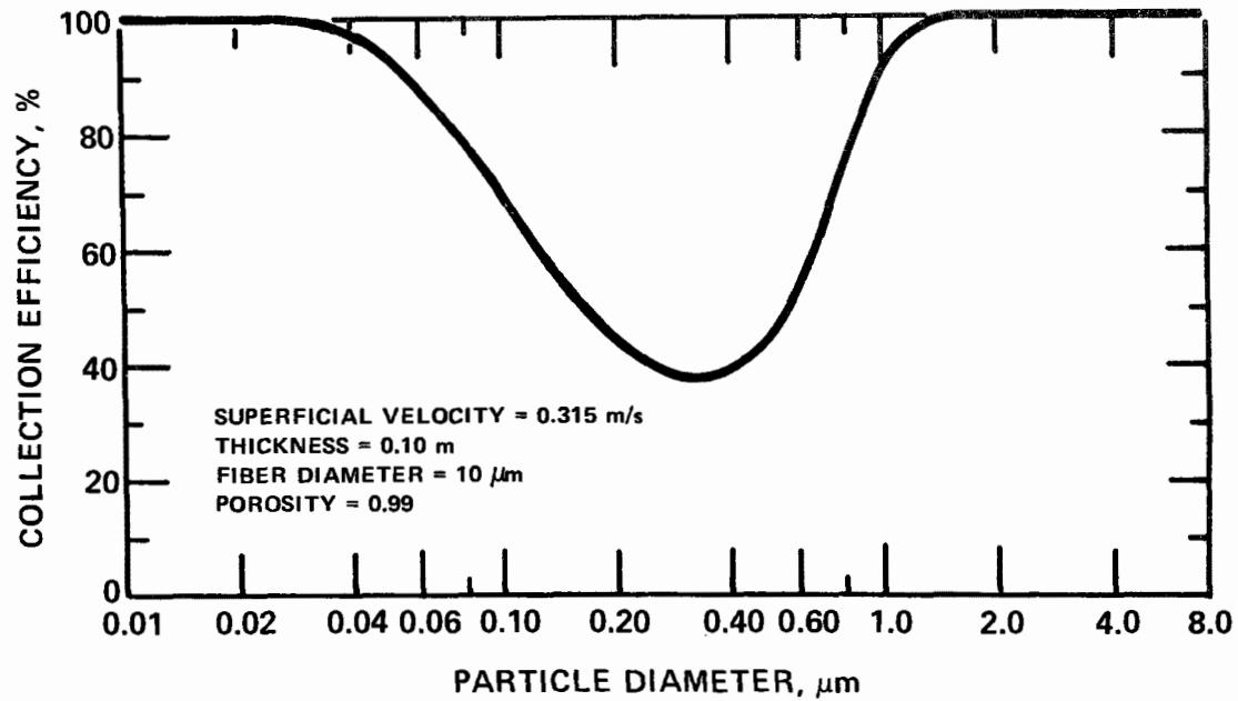
Figure 4. Fibrous filter efficiency versus particle diameter.
