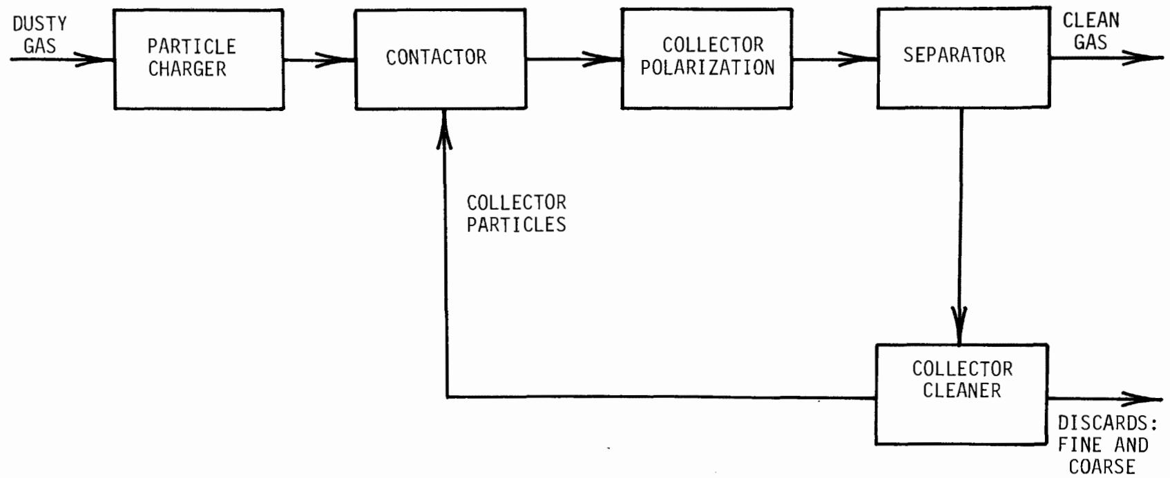
Figure 1. Schematic diagram of A.P.T. Dry Scrubber System.
