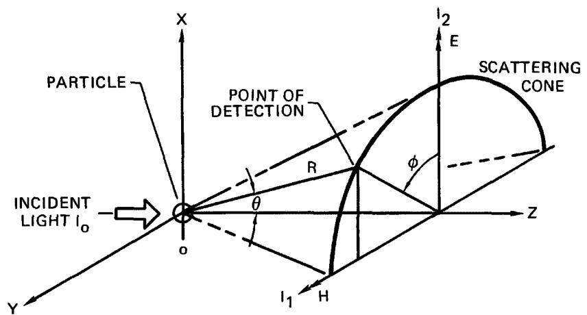
Figure 1. Schematic Of Light Scattering Geometry
