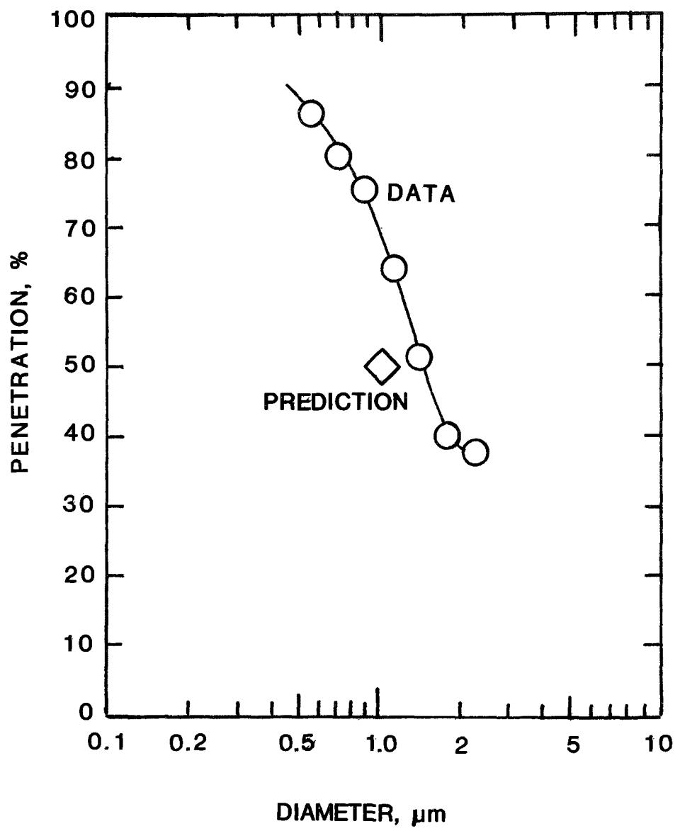
Figure 5. 100°C, 5 atm run with ceramic fiber substrate.
