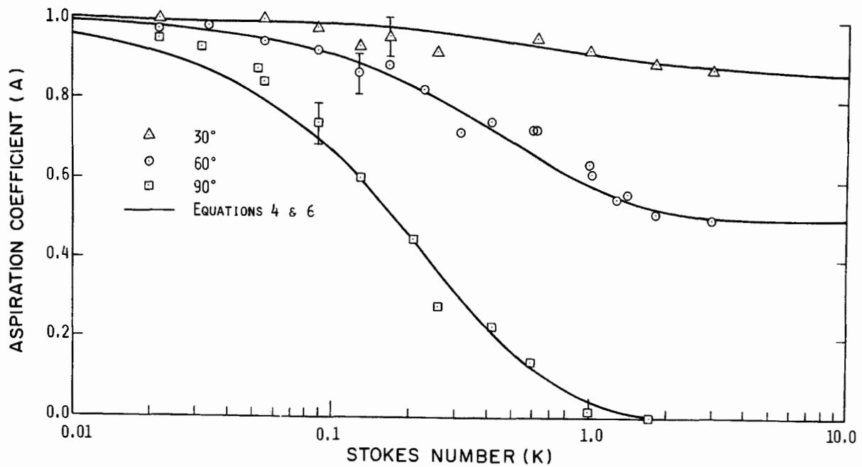
Figure 7. Aspiration coefficient vs. Stokes number--empirical equation and experimental data for 30, 60, and 90 degrees.
