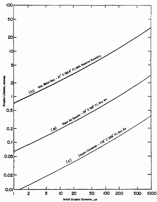
**Figure 3. Lifetime of water droplets traveling at their terminal velocity.**
