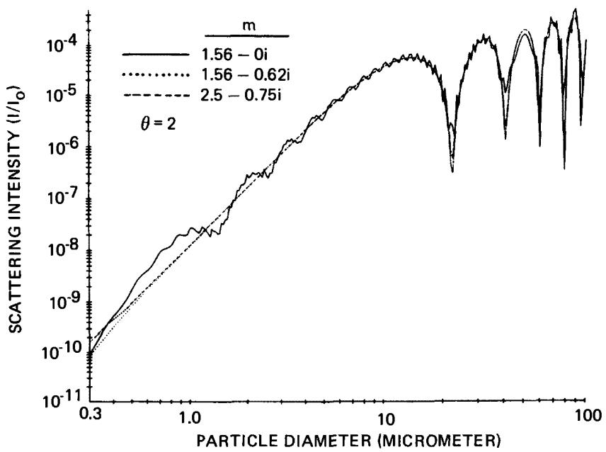
Figure 7. Calculated Mie Scattering Response Curve at  $\theta = 2^\circ$  and  $\lambda = 0.647 \mu\text{m}$
