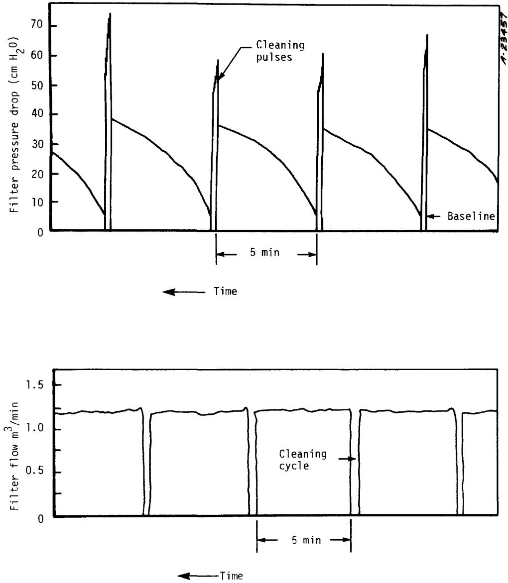
Figure 4. Acurex HTHP ceramic bag filter pressure drop and flow.
