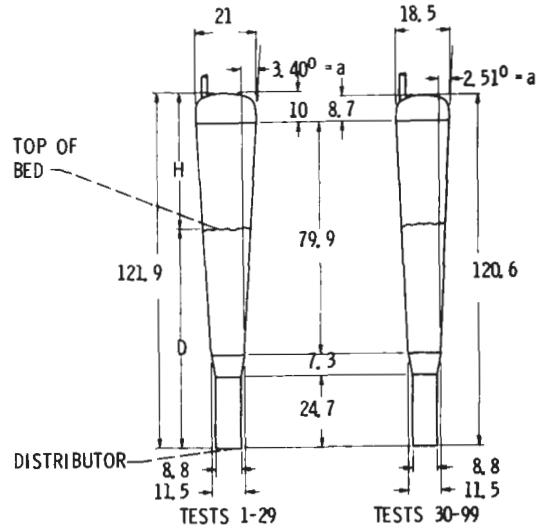
Figure 2 Two internal geometries of combustor (dimensions in inches except D and H; discharge solids removal auger and heat exchanger tubes omitted).
