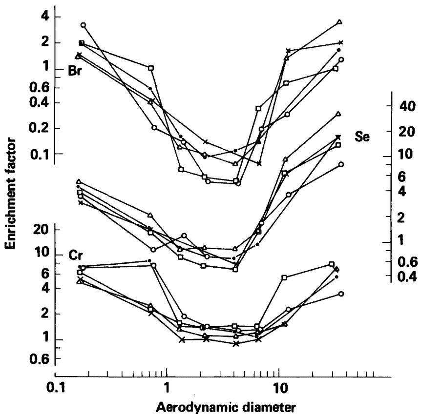
**Figure 6.** Relative concentrations of three elements in discrete size fractions of stack fly ash from Plant A.
