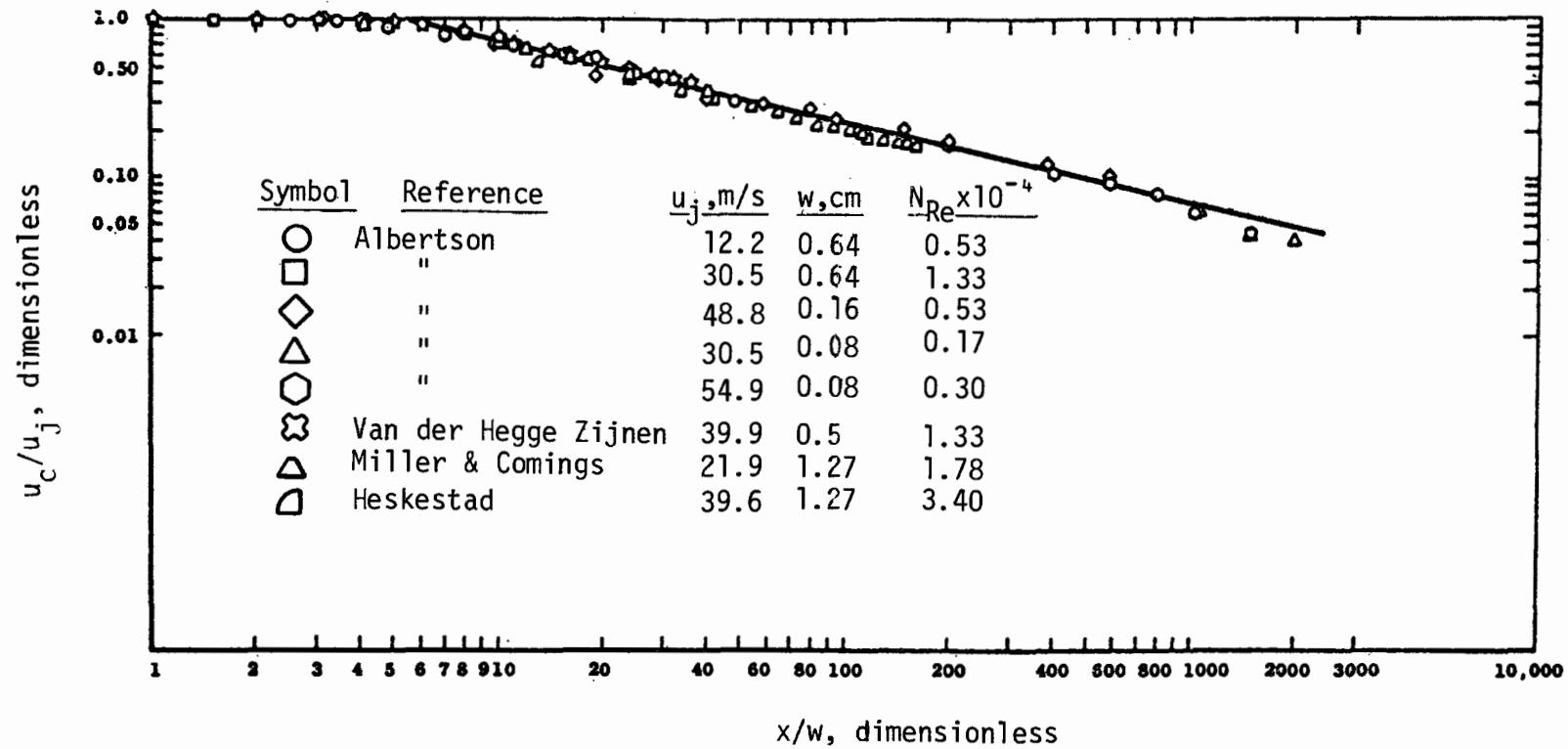
Figure 3. Axial decay of centerline velocity ratio, two-dimensional jet into still air.
