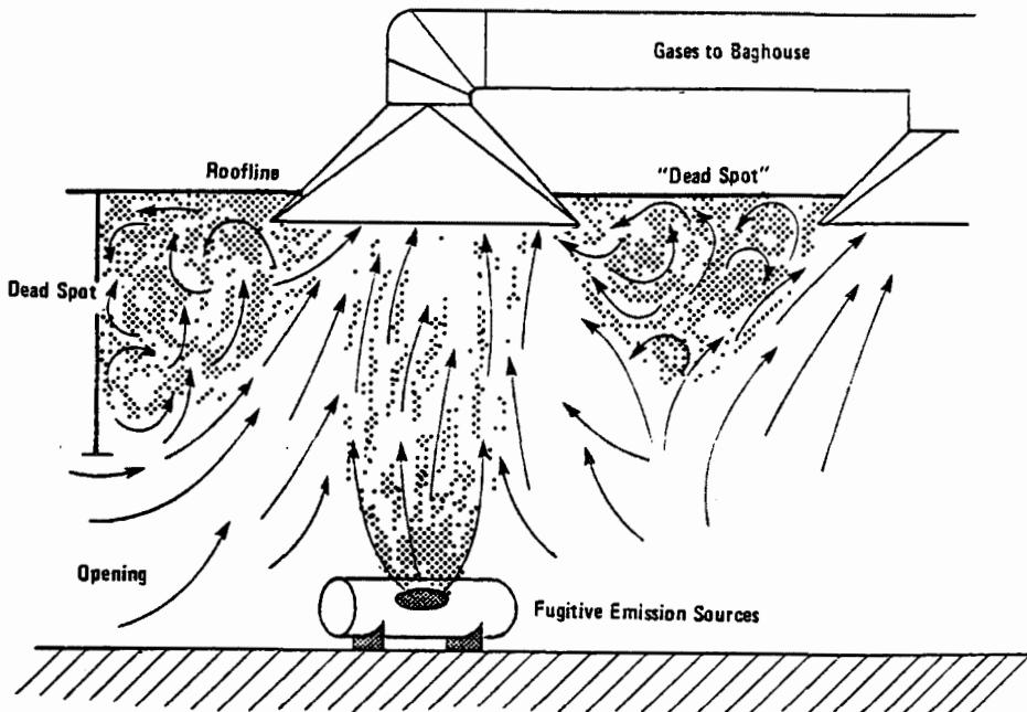
**Figure 4. Schematic of "Dead Spots" in building evacuation system.**
