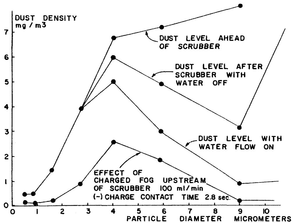
Figure 7 Data showing effects of applying charged fog ahead of 300 ACFM Buffalo Forge wet scrubber. Contact time: 2.2 seconds.
