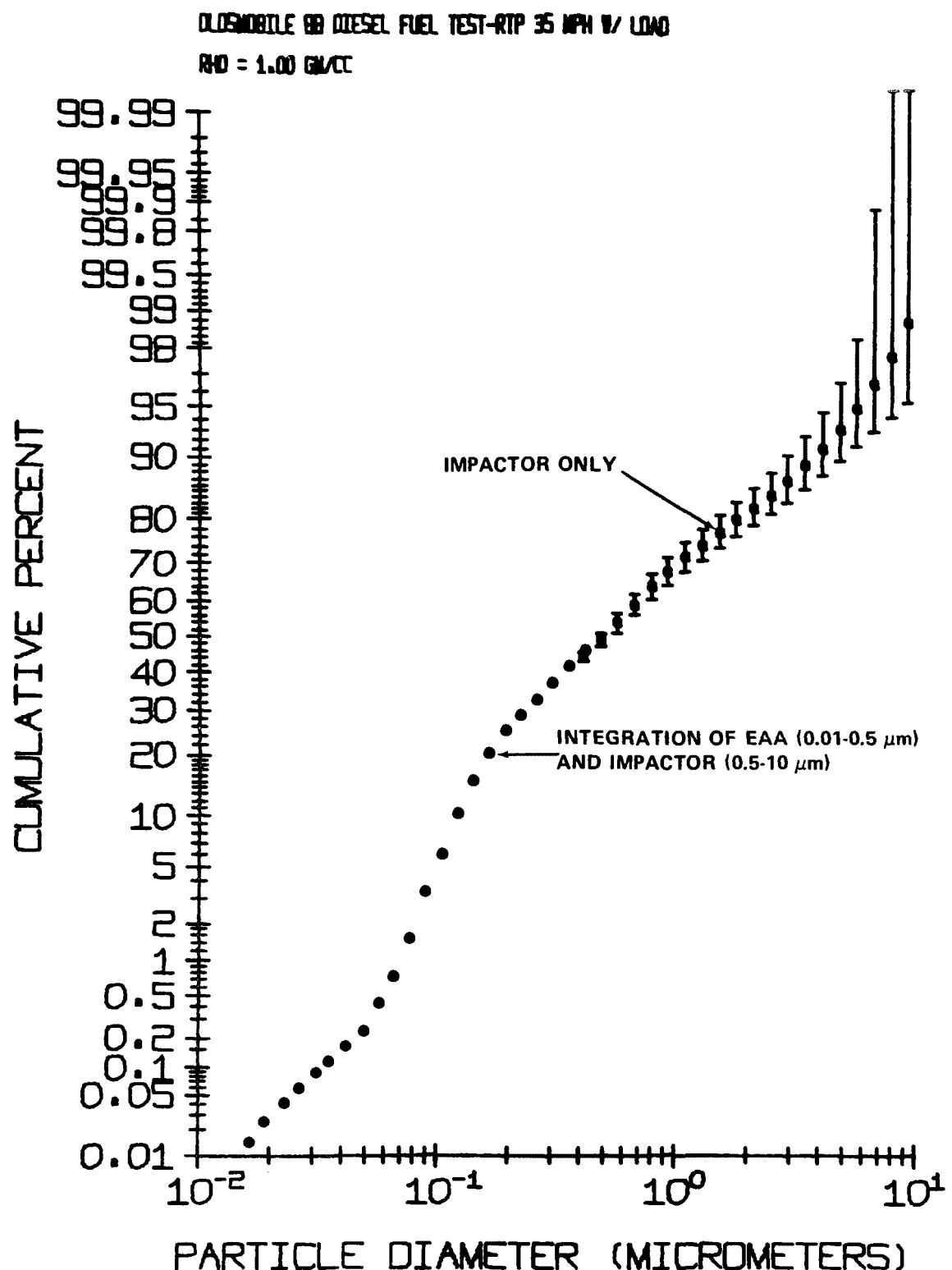
Figure 4. Particle size distribution for 35 mph with load condition.
