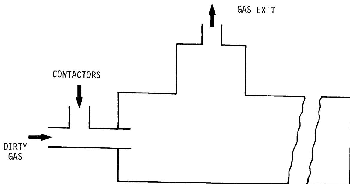
Figure 3. Contactor and gravity separator.
