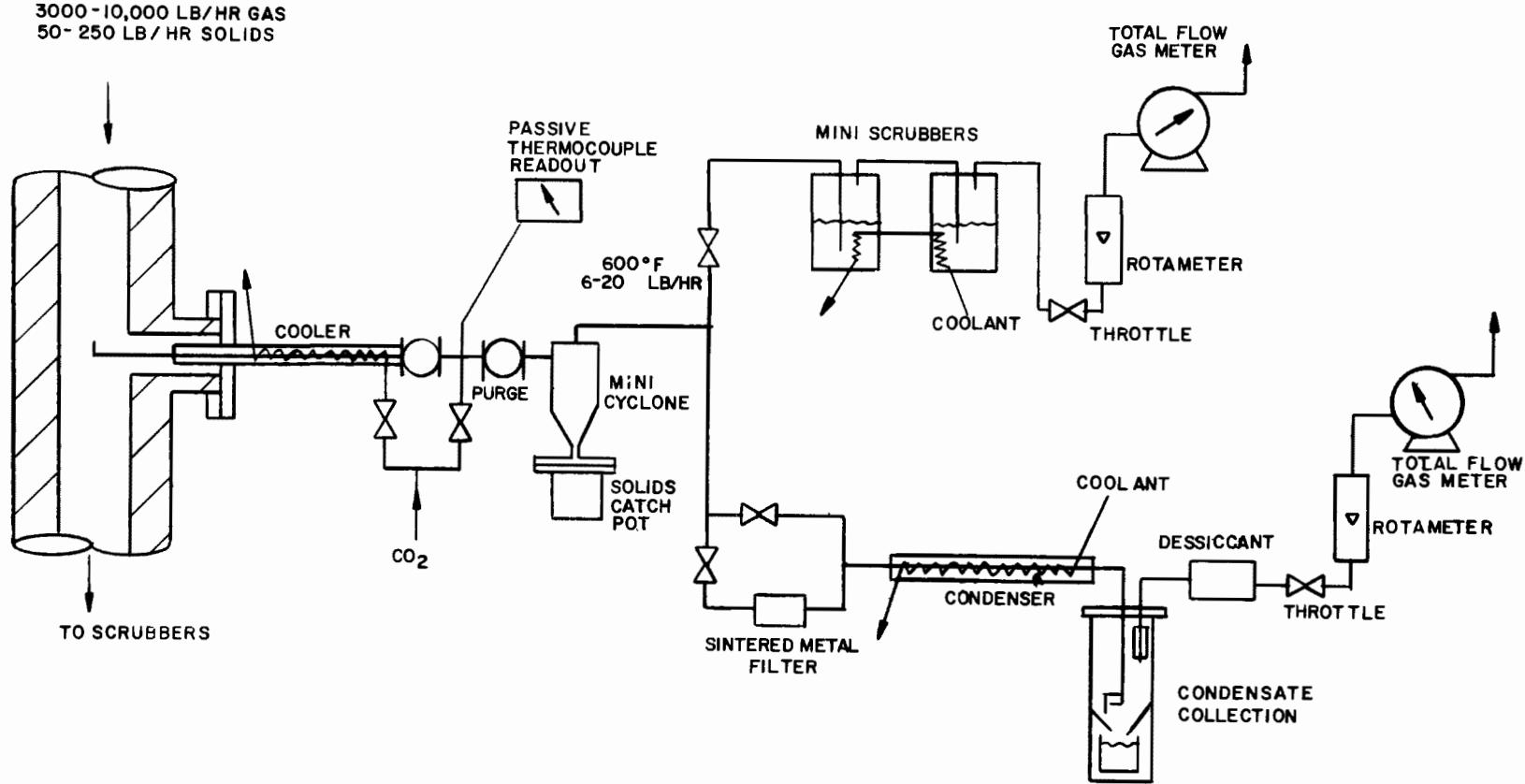
Figure 3. Westinghouse Coal Gasification High-Temperature, High Pressure Particulate Sampling and Characterization System
