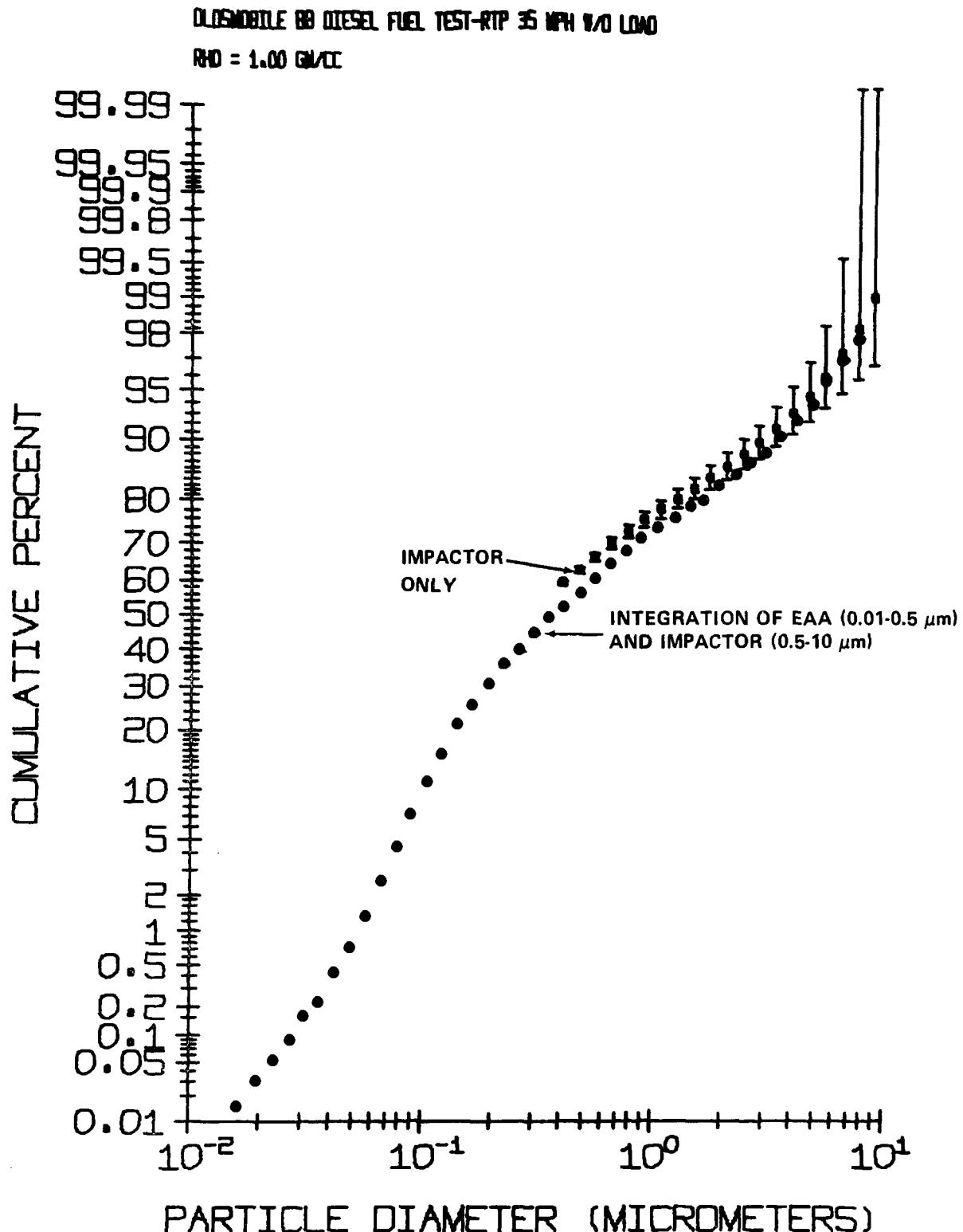
Figure 3. Particle size distribution for 35 mph no load condition.
