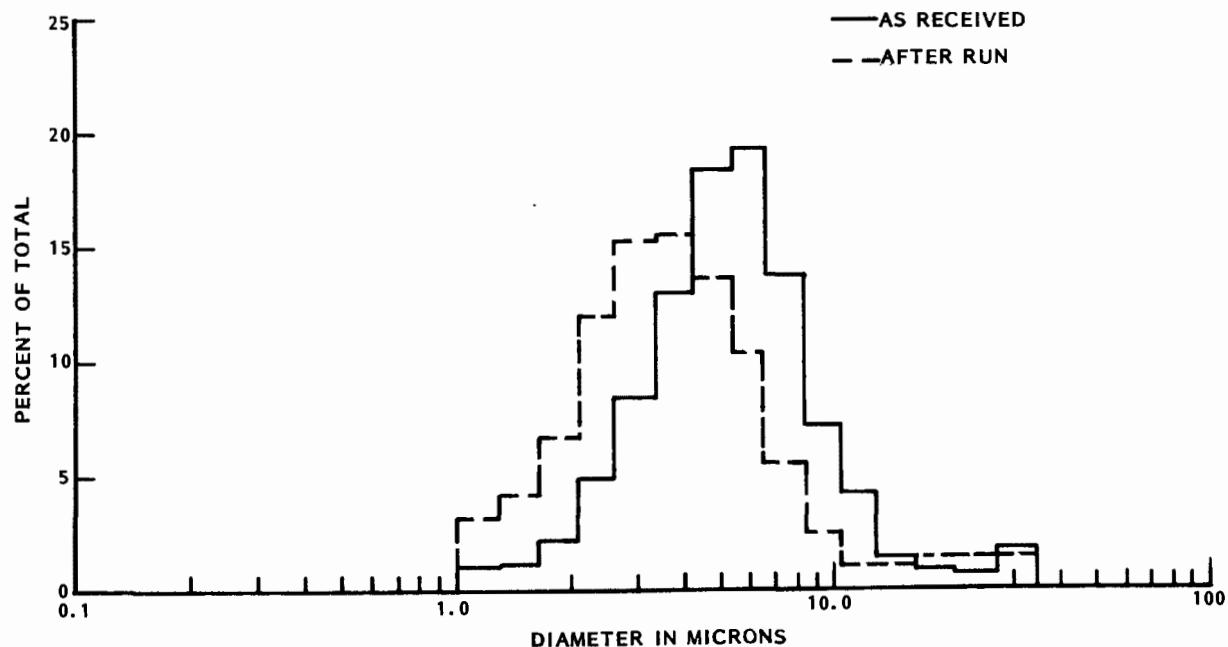
Figure 12. Coulter counter analysis of fly ash 3; — as received, - - after run using 100 micron orifice.
