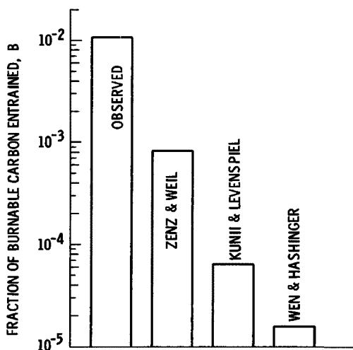
Figure 10 Comparison of burnable carbon entrained based on experiment and three elutriation correlations used in the model of Horio, et al. (1977).<sup>7</sup>
