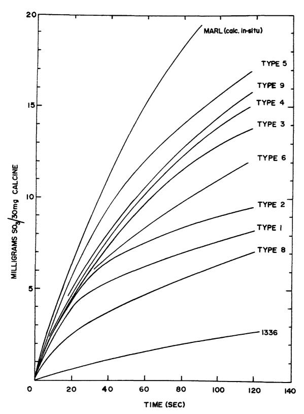
Figure 2-1. Comparison of Reactivity of Calcines with  $SO_2$  at  $980^{\circ}$ C. Particle size = 150/170 mesh.
