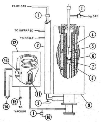
Figure 1-1. Differential Reactor
