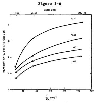
${\rm Reaction~rate~vs.~1/\overline{D}_p}$  Sulfate loading = 2 imes 10–3 g. moles/g.
