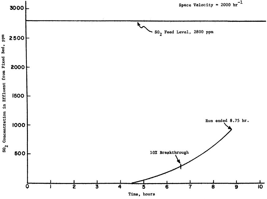
Figure F-1. Breakthrough Curve: 802 Sorption from Flue Gas at 250°F with Wesvaco Char
