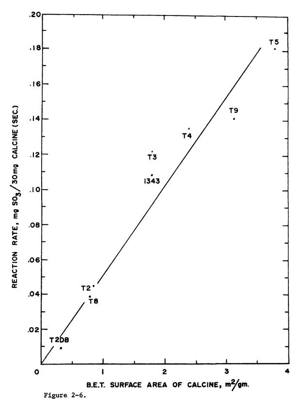
Reaction Rate vs. Surface Area of 150/170 mesh Particles. Rates Evaluated at  $980^{\circ}$ C. and Sulfate Loading of  $29.1 \times 10^{-4}$  gm.moles/gm.
