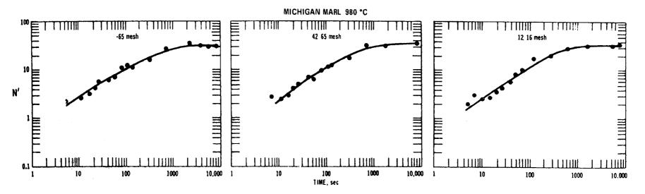
$N^{1} = mg. SO_{3}$  absorbed by 30 mg. calcine
