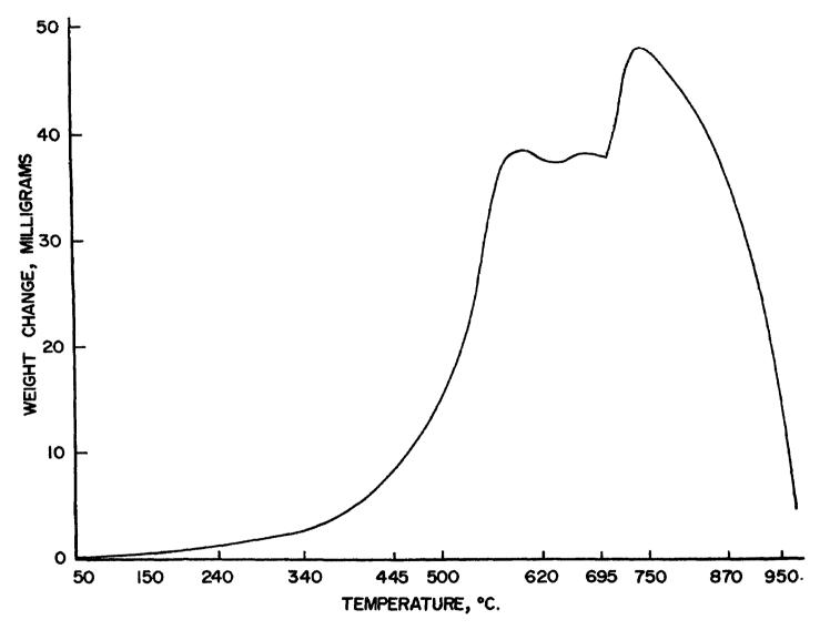
Figure E-1. Thermogravimetric Analysis of Reactivity of Cupric Oxide to  $SO_2$
