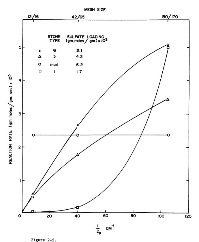
Reaction Rate at Constant Sulfation as a Function of Particle Diameter.
