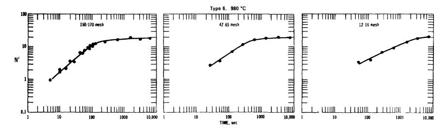
$N^{T} = mg$ .  $SO_{3}$  absorbed by 30 mg, calcine
