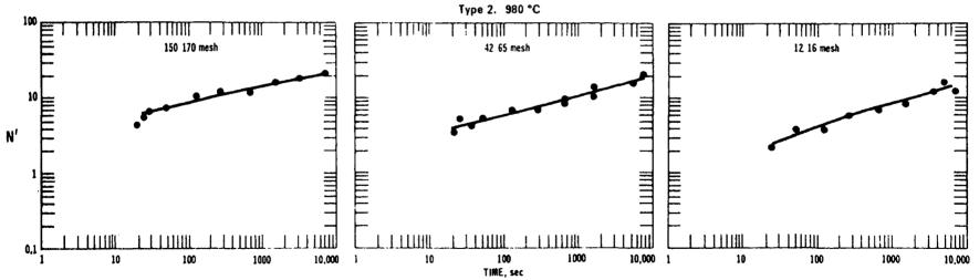
$N' = mg. SO_3$  absorbed by 30 mg. calcine
