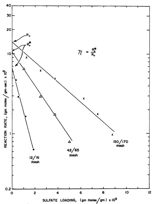
Figure 2-3. Estimation of Initial Rate,  $r_0$ , and Effectiveness Factor,  $\eta$ , for the Sorption of  ${\rm SO}_2$  by Type 4 Calcine,
