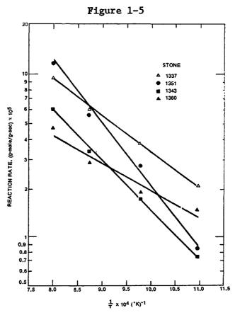
Arrhenius plots for the reaction of sulfur dioxide with four limestones
