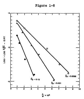
Relation of reaction rate and sulfate loading for dolomite
