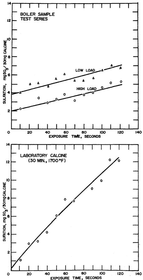
Figure 3-2. Reaction of SO<sub>2</sub> with Calcined Limestone at 1600°F in Flue Gas, 0.27 percent SO<sub>2</sub>.
