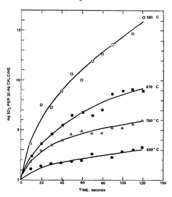
Sorption of sulfur dioxide by dolomite 1351 at various reactor temperatures  ${\bf r}$
