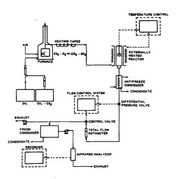
Flow diagram for fixed-bed reactor system
