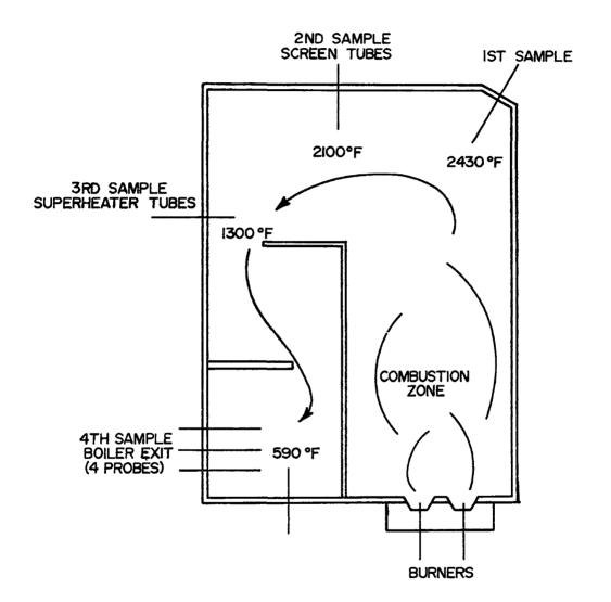
BOILER PLAN AND SAMPLE LOCATIONS, TOP VIEW
