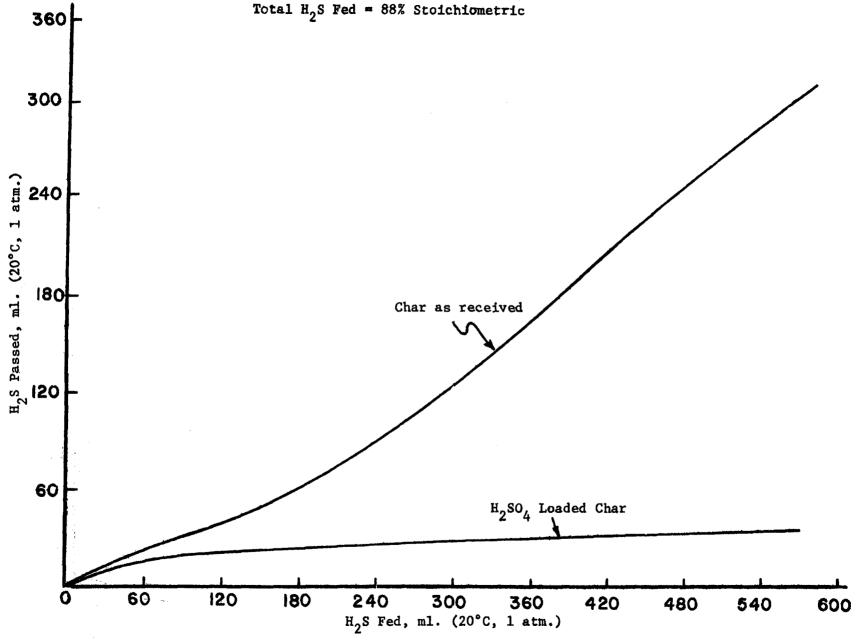
Figure F-4. 300°F H<sub>2</sub>S Reduction
