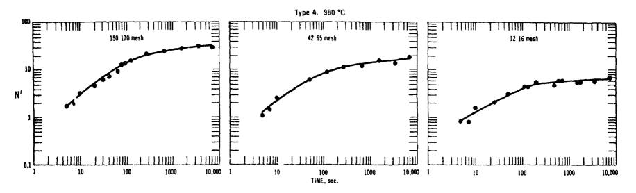
N' = mg. SO<sub>3</sub> absorbed by 30 mg. calcine
