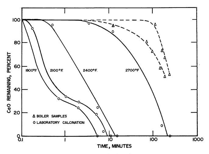
Figure 3-3. Rate of Hydration of Calcined Dolomite: Test Series 1
