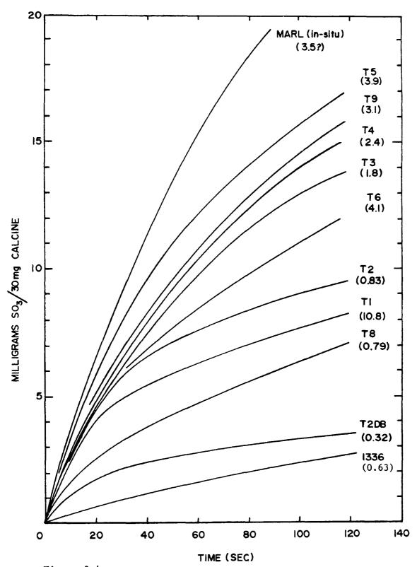
Figure 2-4. Comparison of Reactivity with B.E.T. Surface Area (in parentheses,  $m^2/gm$ .)
