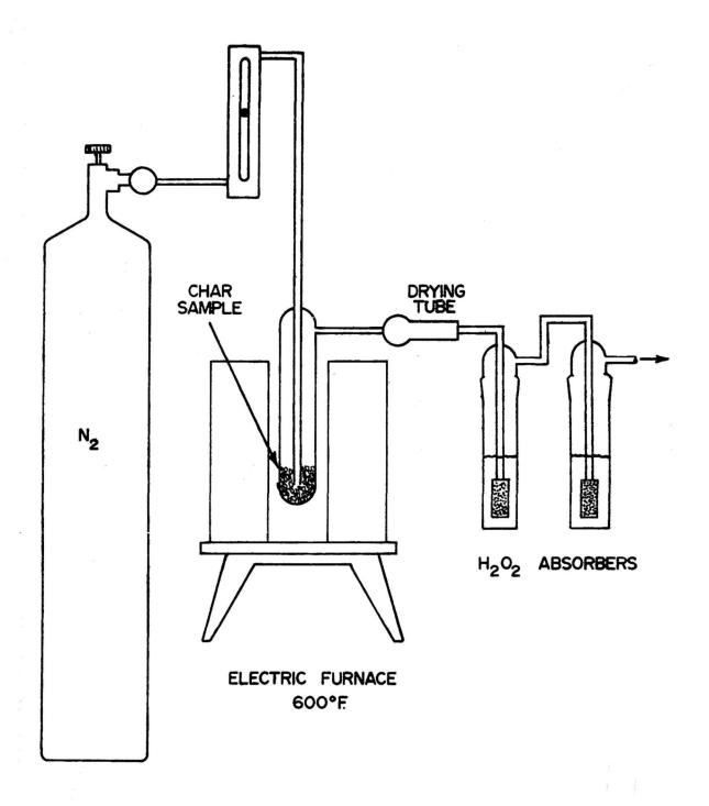
Figure F-6. Apparatus used for H<sub>2</sub>SO<sub>4</sub> Reaction Experiments
