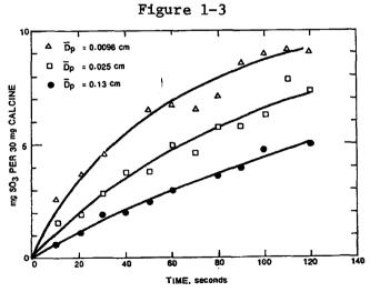
Sorption of sulfur dioxide by different particle sizes of dolomite 1351
