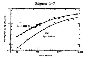
Sorption of sulfur dioxide by calcined limestones
