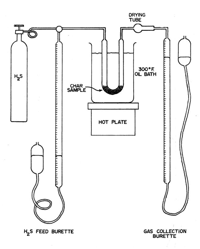
Figure F-2. Apparatus used for  $H_2SO_4/H_2S$  Reduction Experiments
