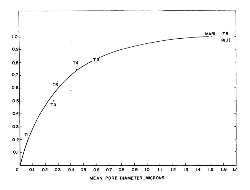
The rate of reaction increases with decreasing pore size until a critical pore diameter of about 0.1 micron is reached. Presumably pores smaller than 0.1 micron are rapidly blocked by reaction products. These blocked pores inhibit diffusion of  $SO_2$  into the solid interior, resulting in a lower rate. Maximum rate results when B.E.T. surface area is in the region of  $3.5 \text{ m.}^2/\text{g.}$  (corresponding to pore diameters of  $0.2 - 0.3\mu$ ) under isothermal reaction conditions.
