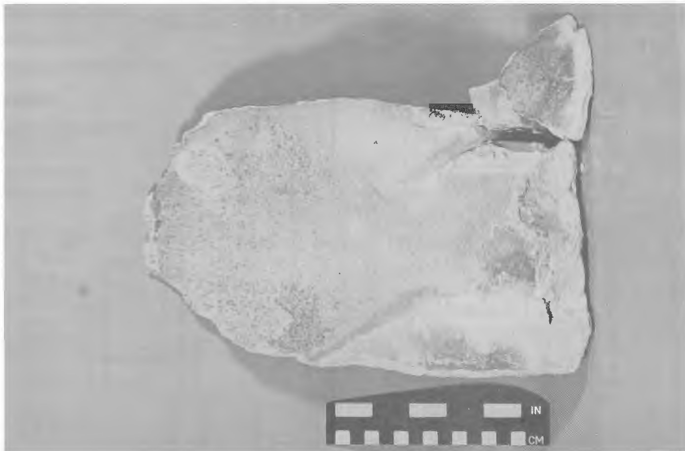
Figure 11. Deposit removed from regenerator after Run 3.
