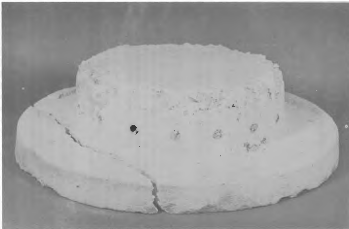
Figure 12. Distributor nozzles blocked by coarse bed material.
