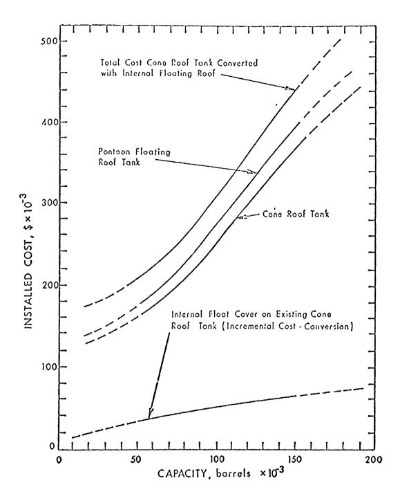
Figure 1. Estimated installed cost of methyl alcohol storage tanks (equipment costs assumed to be the same as gasoline storage tanks) $^{22}$
