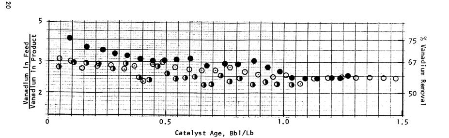
Up to a catalyst age of 0.5 Bb1/Lb, the activity of the two catalysts is about equal, but below the LX-22-5 catalyst. There is no apparent explanation for the unusually high initial demetallization activity exhibited by LX-22-5. From age 0.5 Bb1/Lb to the end of the run, the 1.0 weight percent molybdenum catalyst exhibited slightly higher demetallization rates over the 2.0 weight percent molybdenum catalyst and had about the same rate as the LX-22-5 catalyst at the end of the run.
