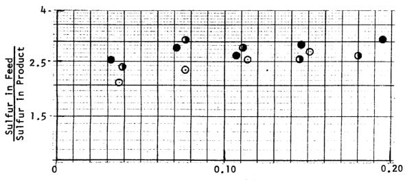
On the basis of the five-day screening test, the commercial production catalyst was accepted to be equal to the laboratory-prepared plant simulation 1.0 weight percent molybdenum catalyst with respect to demetallization and desulfurization. To test deactivation rates, aging tests were scheduled using Tia Juana vacuum residuum as well as other feedstocks.
