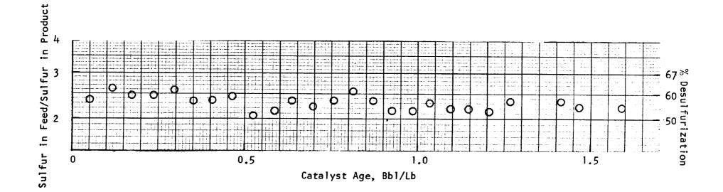
LX-22 catalyst (2.0 W % molybdenum on 20 x 50 mesh bauxite, prepared by HRI). Initial vanadium removal was about 89 percent and this value dropped to about 77 percent at a catalyst age of 1.6 Bbl/Lb. Nickel removal ranged from 63 to 75 percent and sulfur removal was about 55 percent. While the level of vanadium removal obtained with this feed was high, the rate of activity decline was modest when compared with the results of other feeds.
