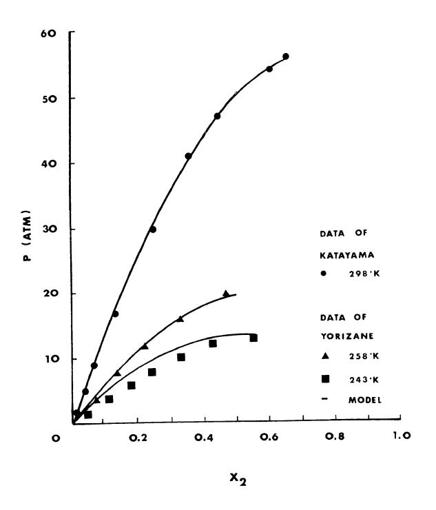
Table 11. Calculated and experimental equilibrium data for methanol-hydrogen sulfide at 258°K.
