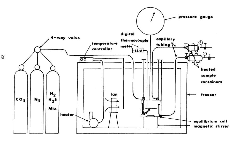
Figure 9. Calibration apparatus.
