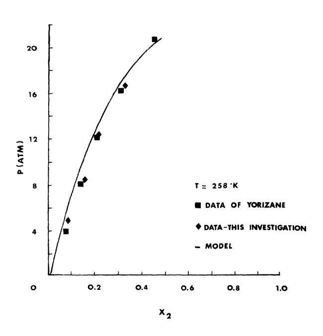
Table 22. Comparison of model and experimental equilibrium data for carbon dioxide-methanol at 258°K.
