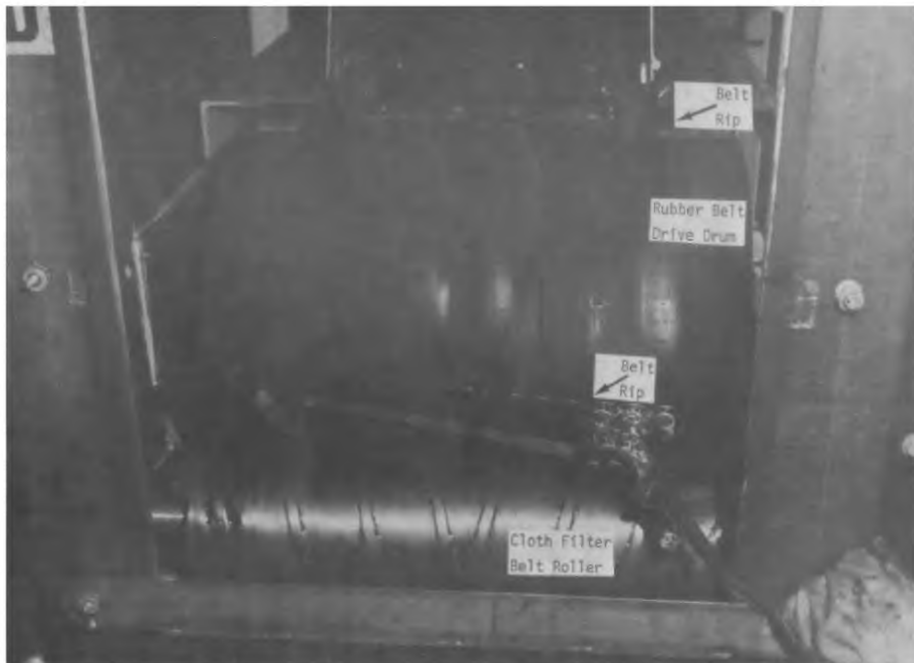
Figure 7. Ripped S-1 filter belt (cloth belt removed)
