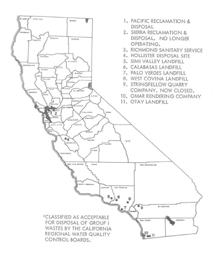
Figure 2. Extremely hazardous waste Class I disposal sites in State of California.
